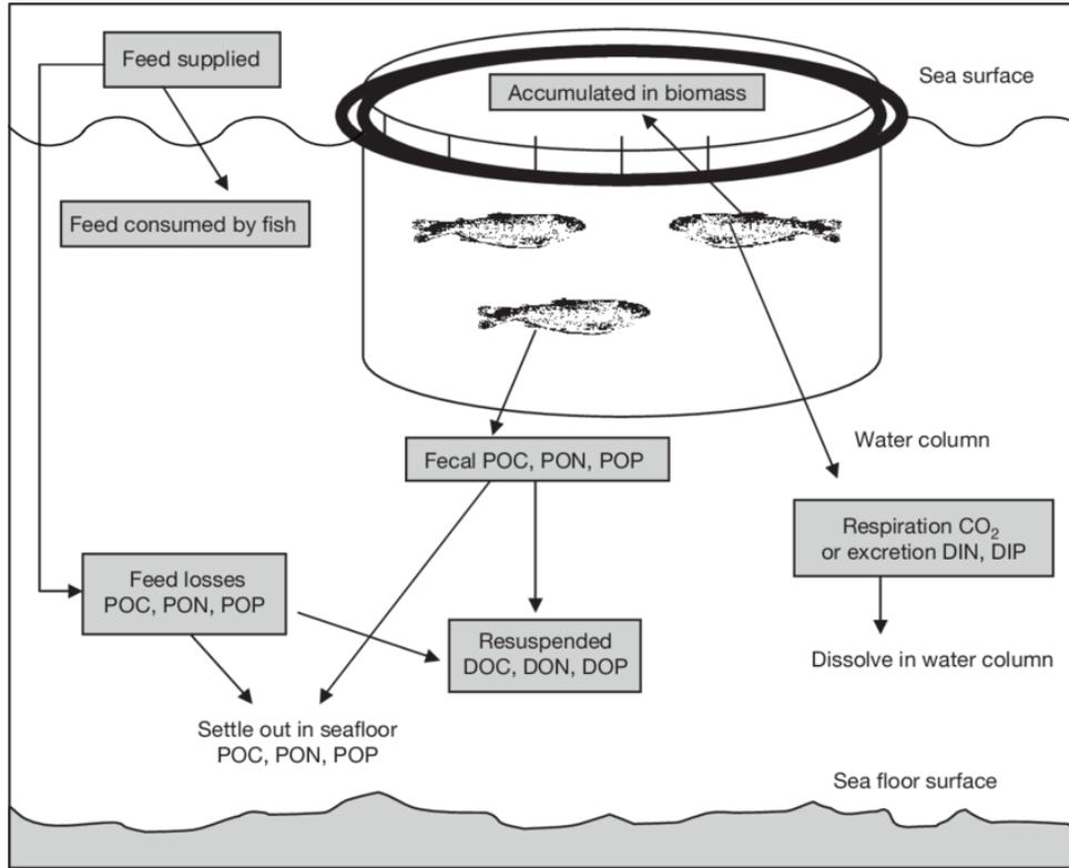
Figure 1.2. The flow and fate of organic waste from salmon cages during production. Particulate organic carbon, nitrogen and phosphorus (POC, PON and POP, respectively) originate from fish feed and fish feces and settle onto the seafloor. Source: Wang et al. (2012).
