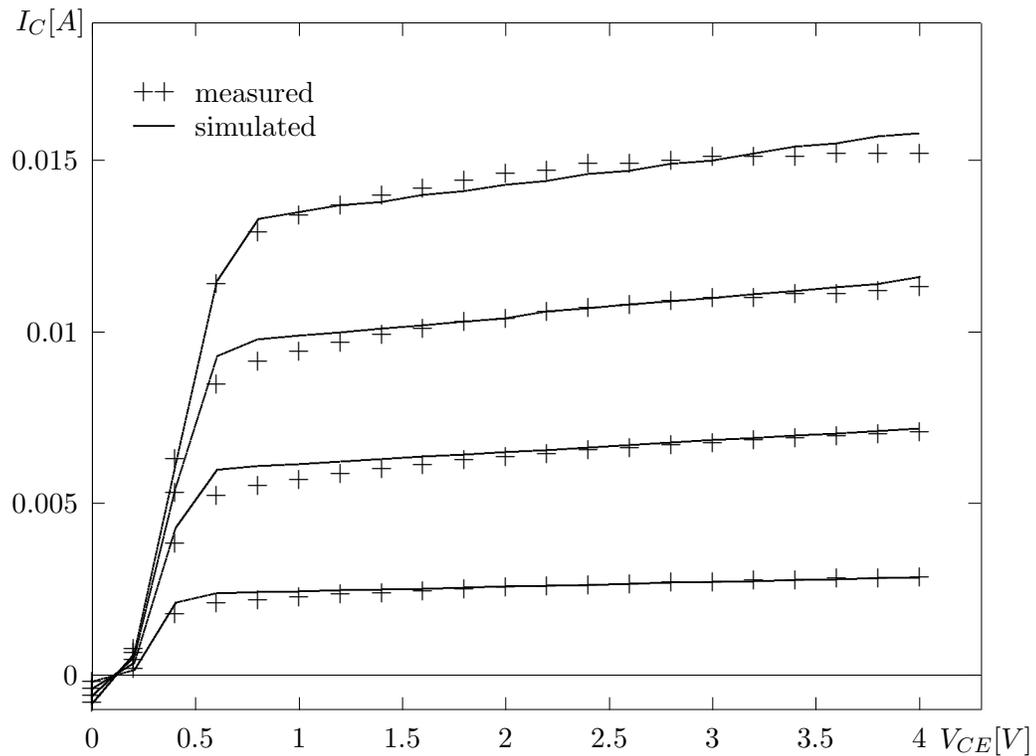
Fig.5. HBT common-emitter DC characteristics; extracted values of parameters.
