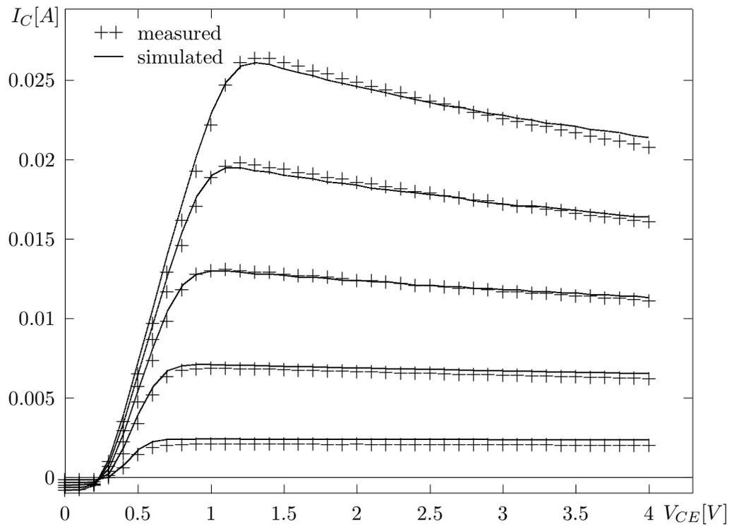
Fig.10. HBT common-emitter DC characteristics; extraction with self-heating effects.
