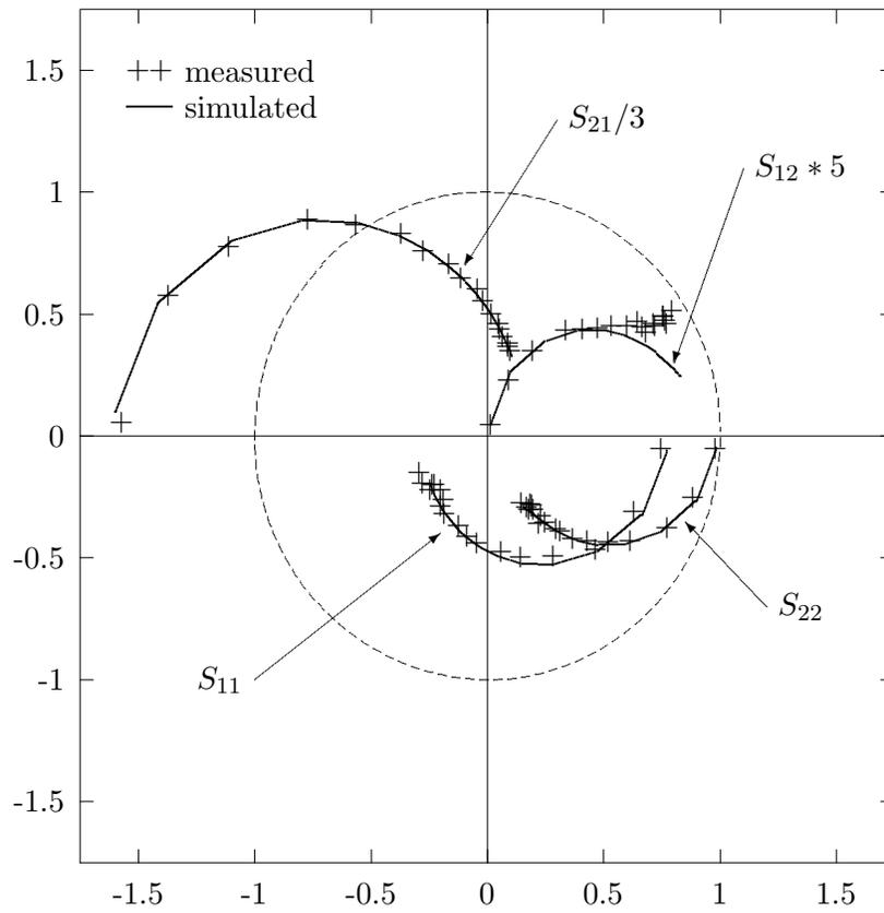
Fig.7. HBT  $S$ -parameters as functions of frequency; extracted values of parameters.
