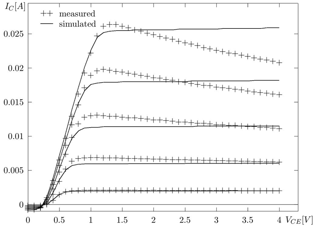
Fig.9. HBT common-emitter DC characteristics; extraction without self-heating effects.
