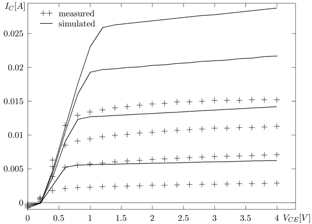
Fig.4. HBT common-emitter DC characteristics; initial values of parameters.
