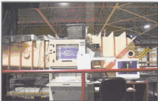
Figure A-6: The IOT cavitation tunnel and LDV control panels
