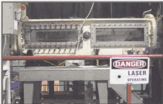
Figure A-5: The IOT cavitation test windows
