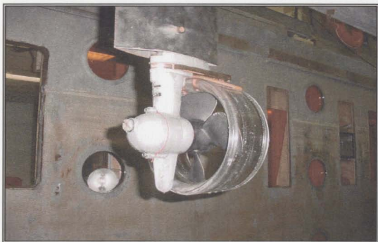
Figure A-4: DP thruster model in the INSEAN cavitation tunnel.
