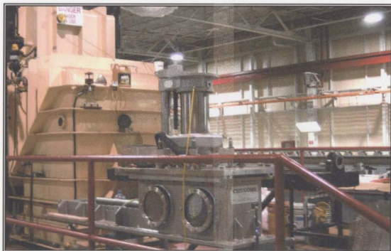
Figure A-7: The IOT cavitation tunnel dynamometer
