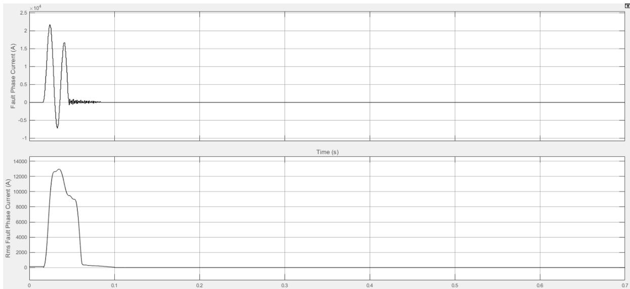
Figure 7.13 Fault current (phase and Rms)
