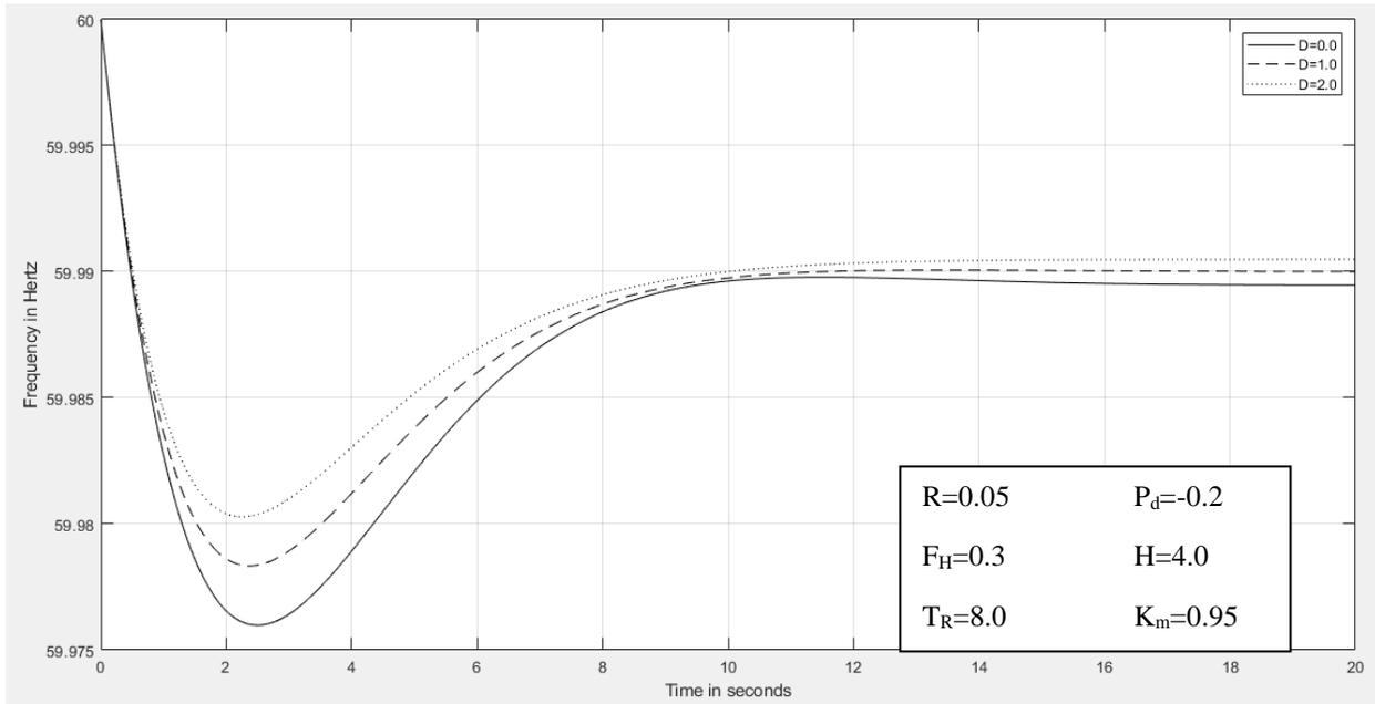
Figure 4.12 Frequency response for varying values of D
