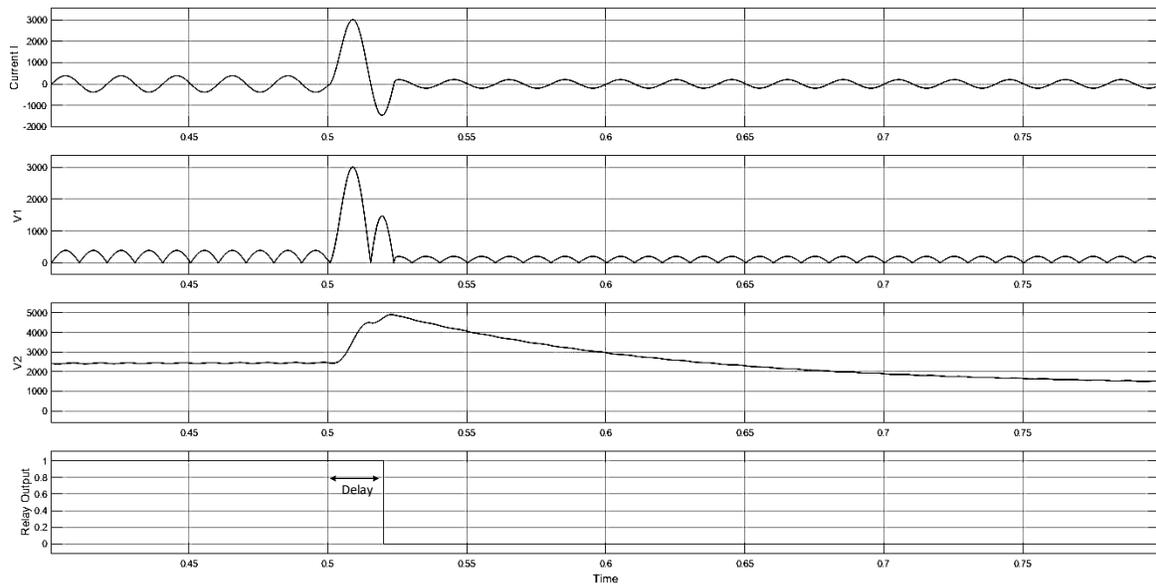
Figure 3.9 Waveforms of an analog solid-state instantaneous overcurrent relay
