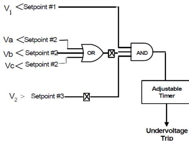
Figure 5.2 Condition of static load shedding [16]
