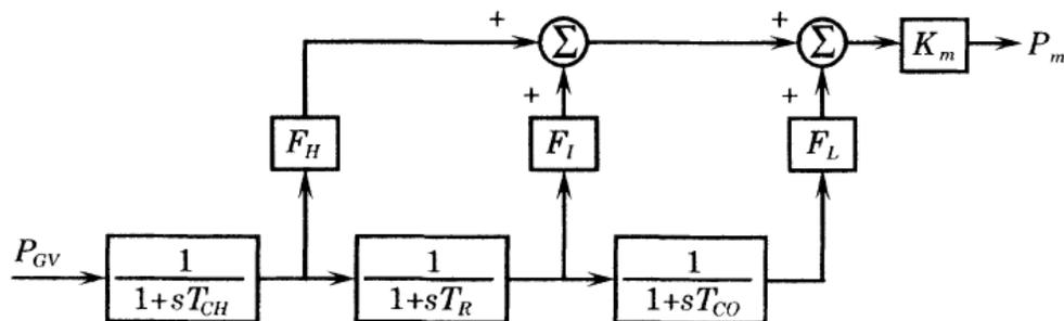
Figure 4.5. Mathematical model of the reheat turbine [1]
