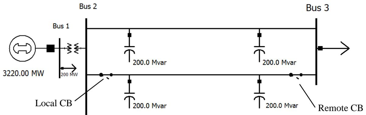
Figure 7.5 Oneline diagram of the modeled system
