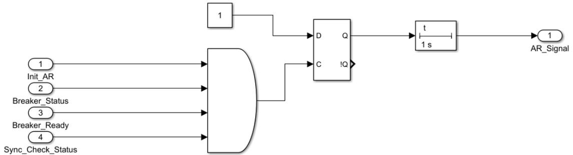
Figure 7.9 Auto-reclose relay subsystem
