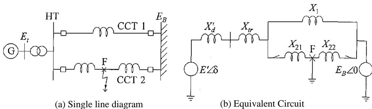
Figure 6.6 Bolted 3 phase fault in SMIB system [33]
