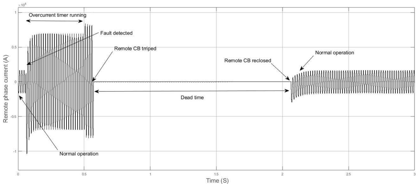
Figure 7.10 Line 2 phase current
