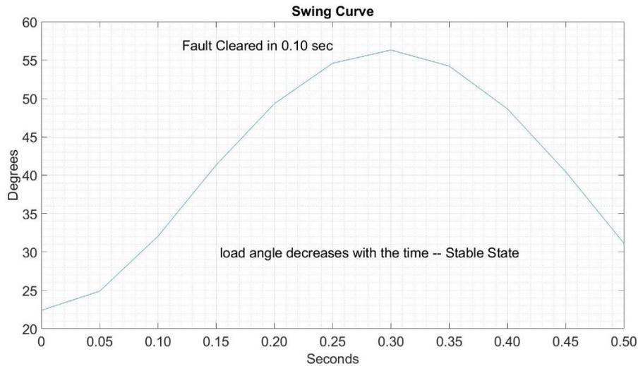
Figure 6.11 The plot of the swing equation for the fault cleared at 0.1 seconds (Stable)
