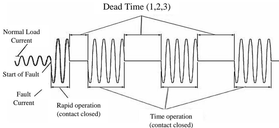
Figure 7.4 Typical sequence for Auto-recloser [36]
