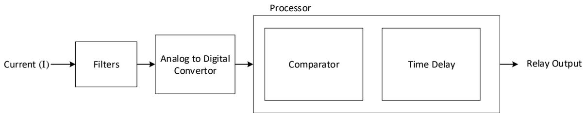
Figure 3.12 A sample blocks used for an analog solid-state instantaneous overcurrent relay
