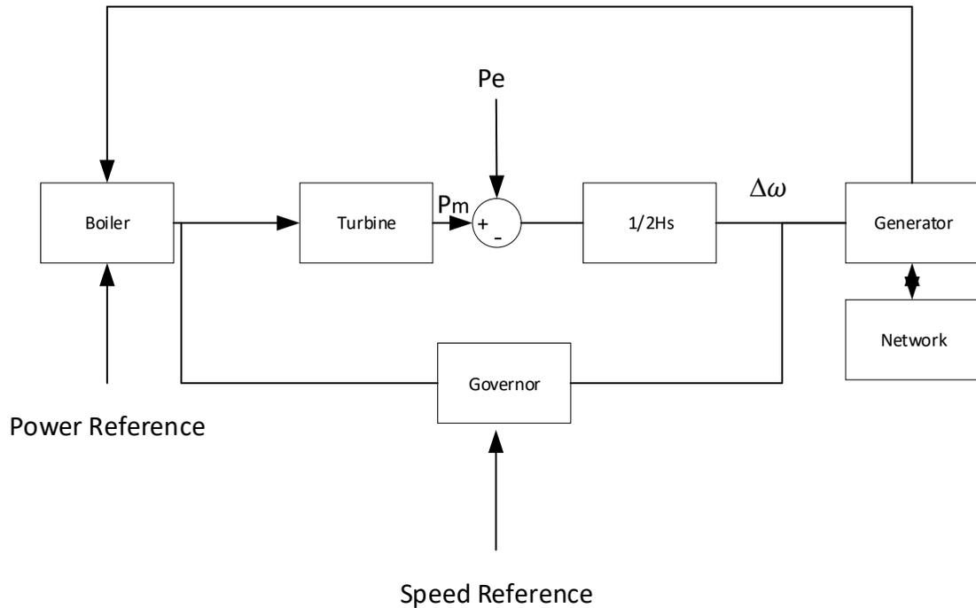
Figure 4.4. Generating Unit Frequency Control [1]
