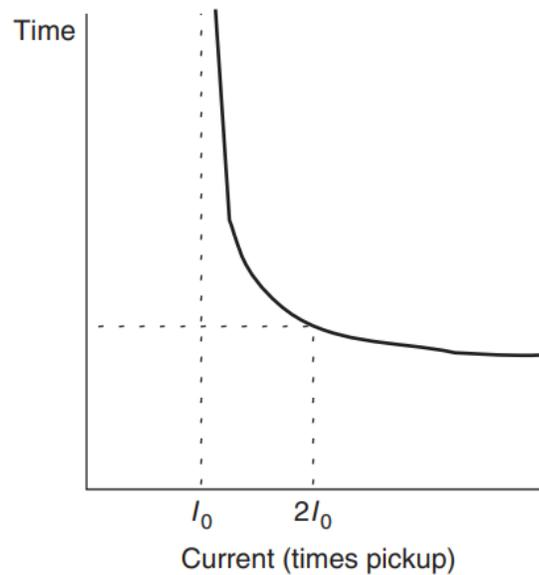
Figure 3.2 Operating time versus current of a plunger relay [1]
