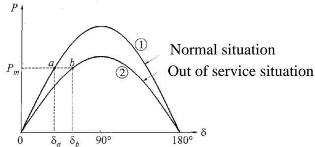
Figure 6.5 Power angle relation plot for SMIB system [33]
