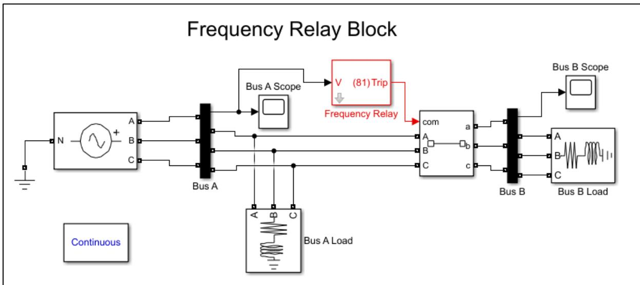
Figure 5.17 Simulated system block diagram
