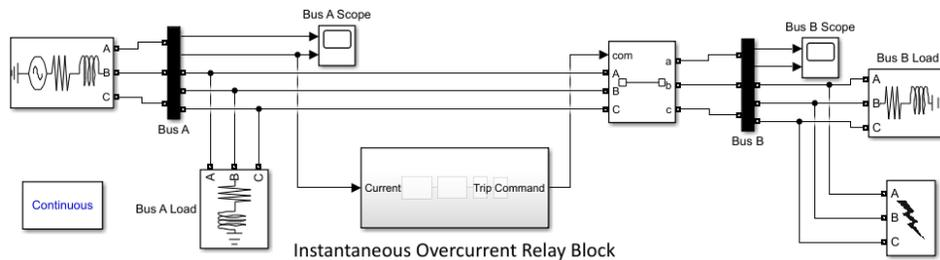
Figure 3.7 2-Bus power system in MATLAB Simulink
