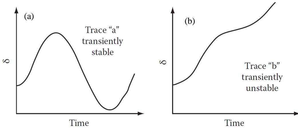
Figure 6.2 Trajectory of generator rotor angle through time [34]
