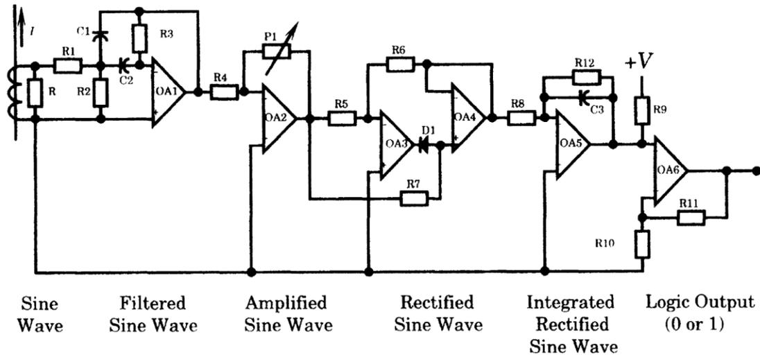
Figure 3.6 An instantaneous overcurrent unit [2]
