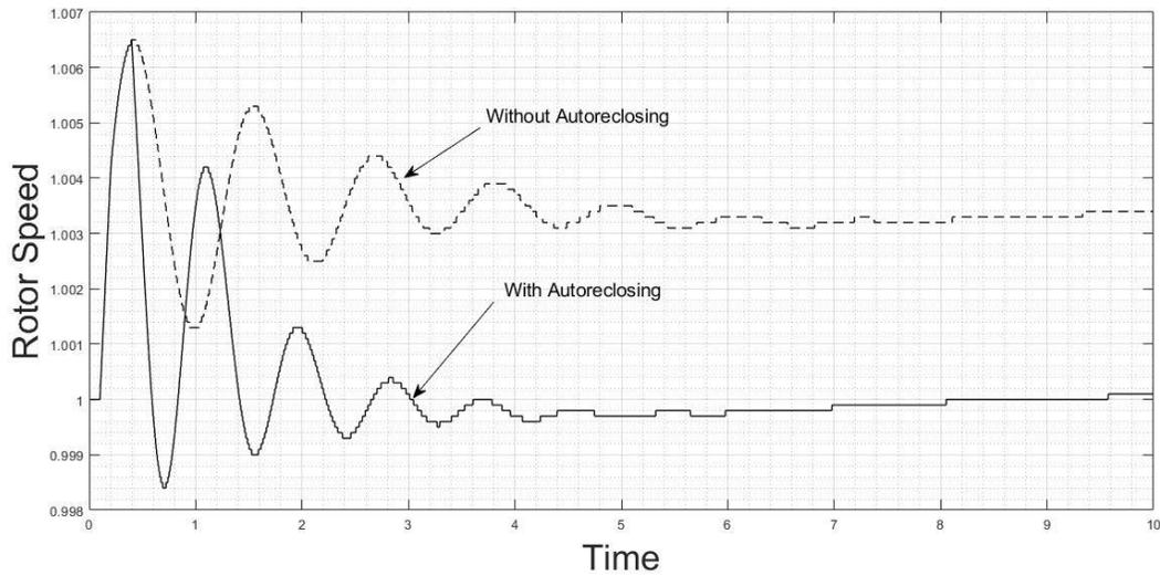
Figure 7.2 Rotor speed of Generator 10
