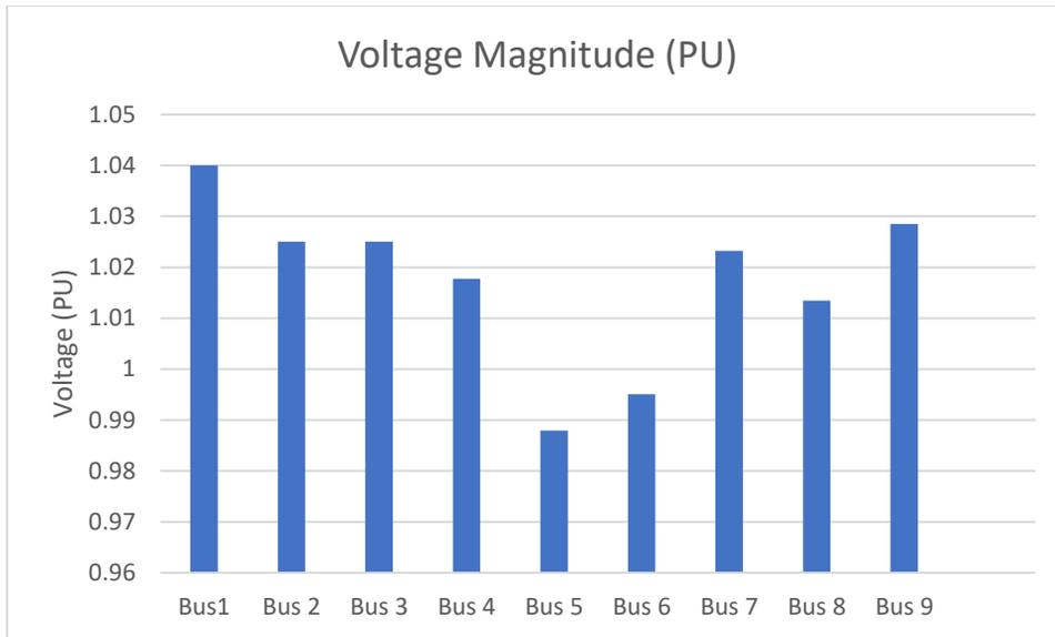
Figure 5.8 pre-fault system voltage profile
