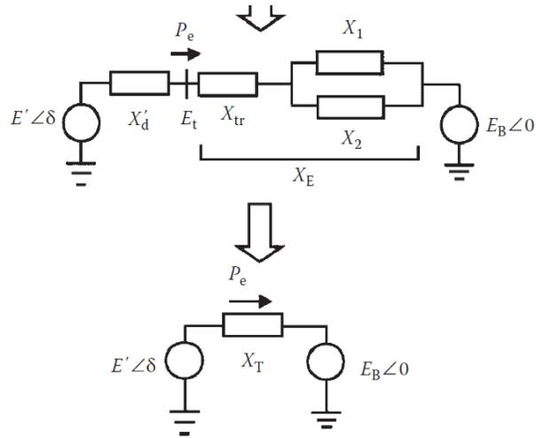
Figure 6.4 Reduced equivalent circuit of SMIB system [34]
