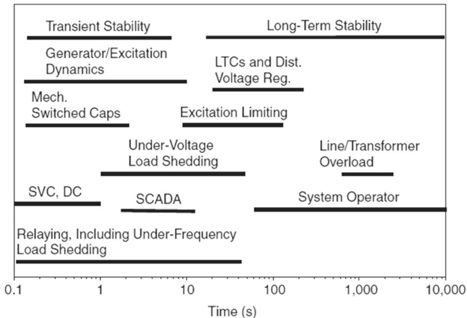
Figure 5.1 Operation time of the network security components after an error [16]
