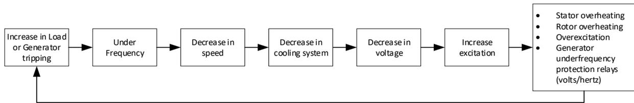
Figure 4.3 The effect of underfrequency on the generator
