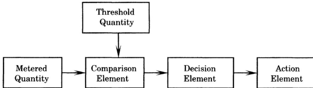
Figure 2.1 The elements of a protective device [2]
