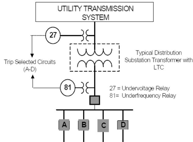
Figure 5.3 Static load shedding in power systems [16]
