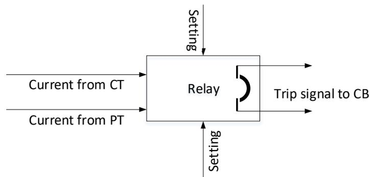
Figure 2.3. Conceptual diagram of a relay [6]
