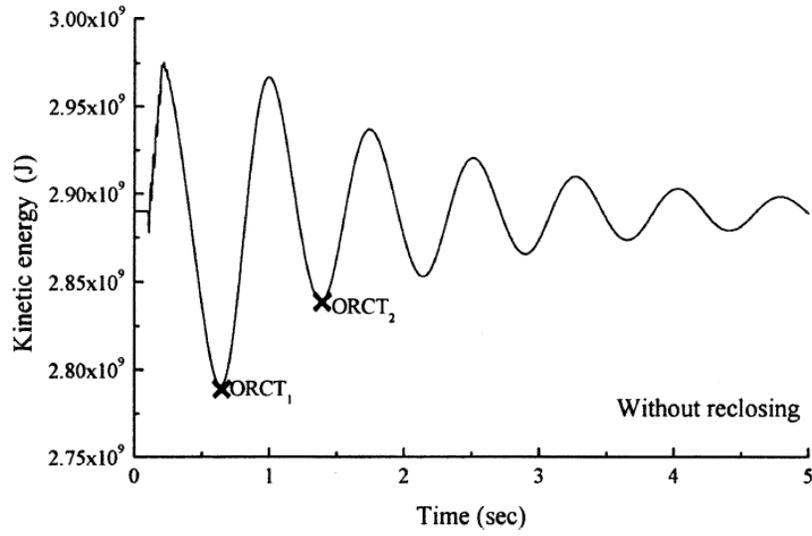
Figure 7.18 Kinetic energy of a synchronous generator subjected to a permanent fault [40]
