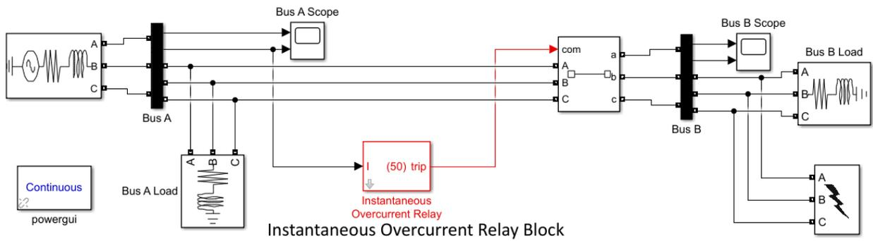
Figure 3.11 Application of a digital instantaneous overcurrent relay in a 2-Bus power system
