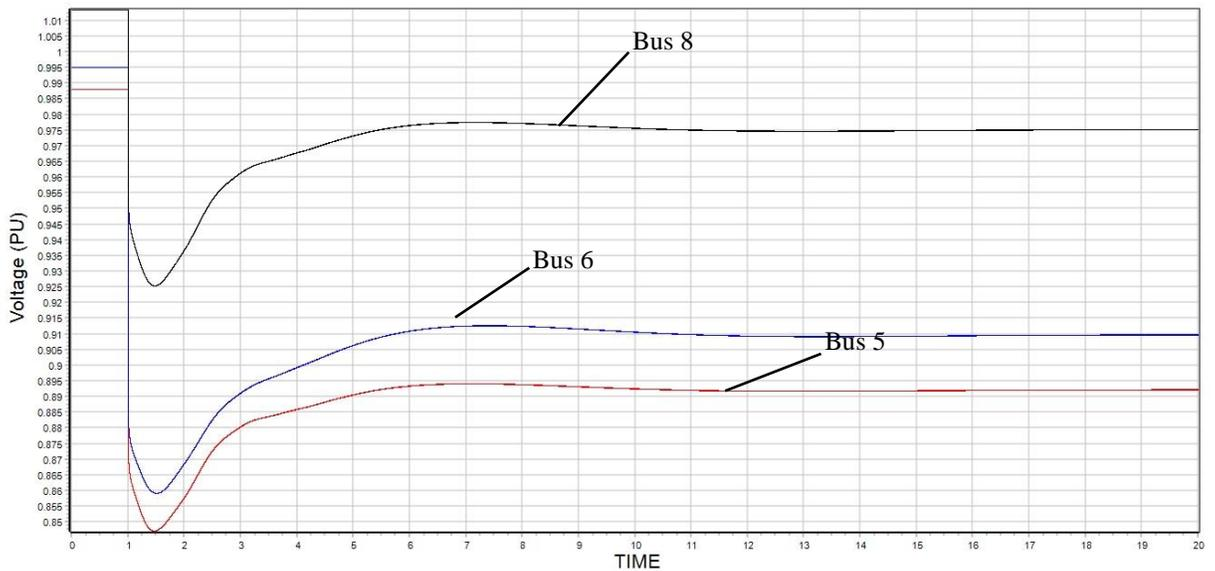
Figure 5.9 Voltage profile after the loss of Generator 12
