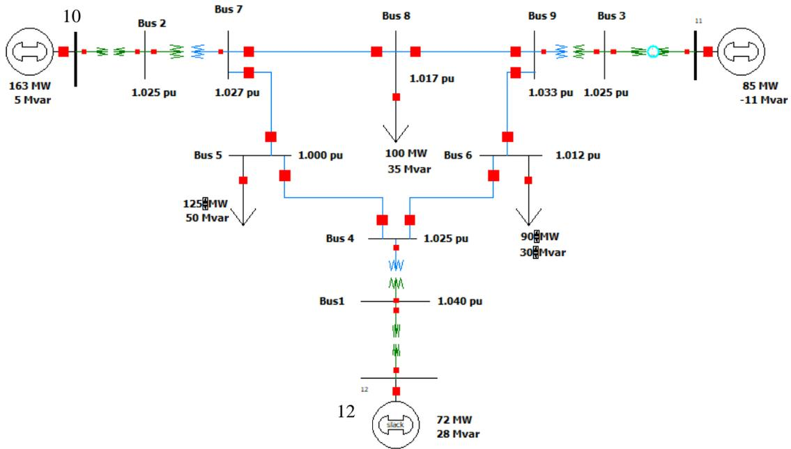
Figure 6.12 Standard IEEE 9-bus oneline diagram
