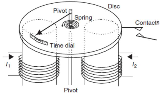
Figure 3.3 Principle of construction of an induction disc relay [1]
