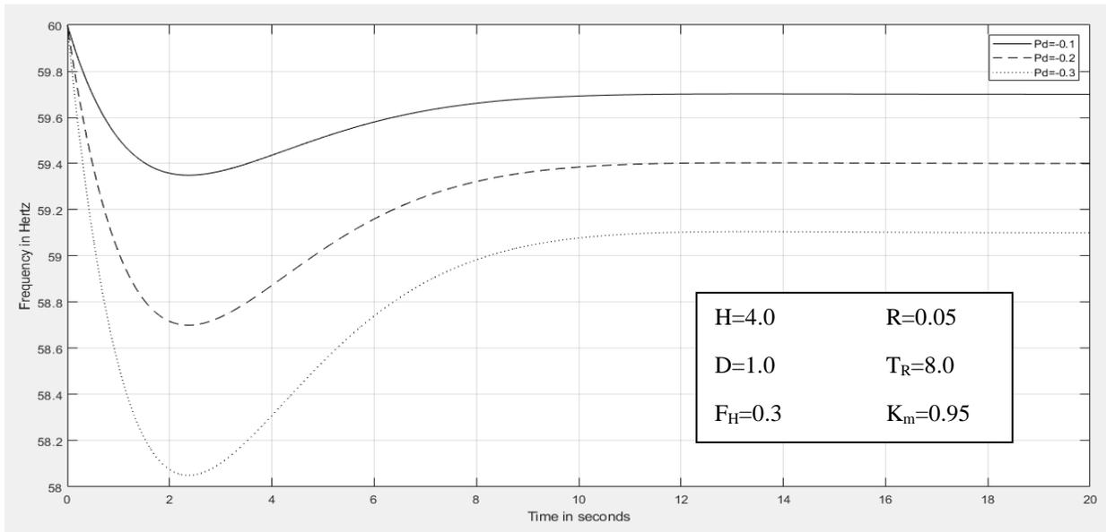
Figure 4.7. Frequency response for different values of  $P_{step}$
