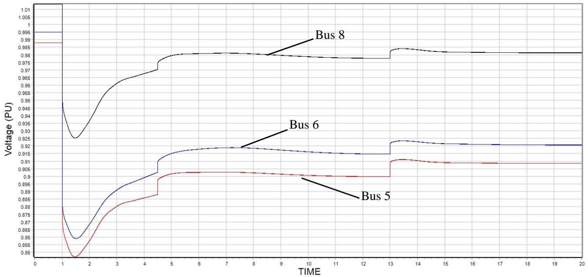
Figure 5.10 Voltage profile with static load shedding
