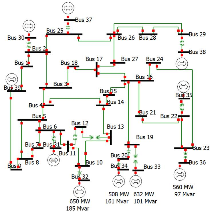
Figure 6.19 Oneline diagram of the IEEE 10-Generator 39-Bus New England Test System
