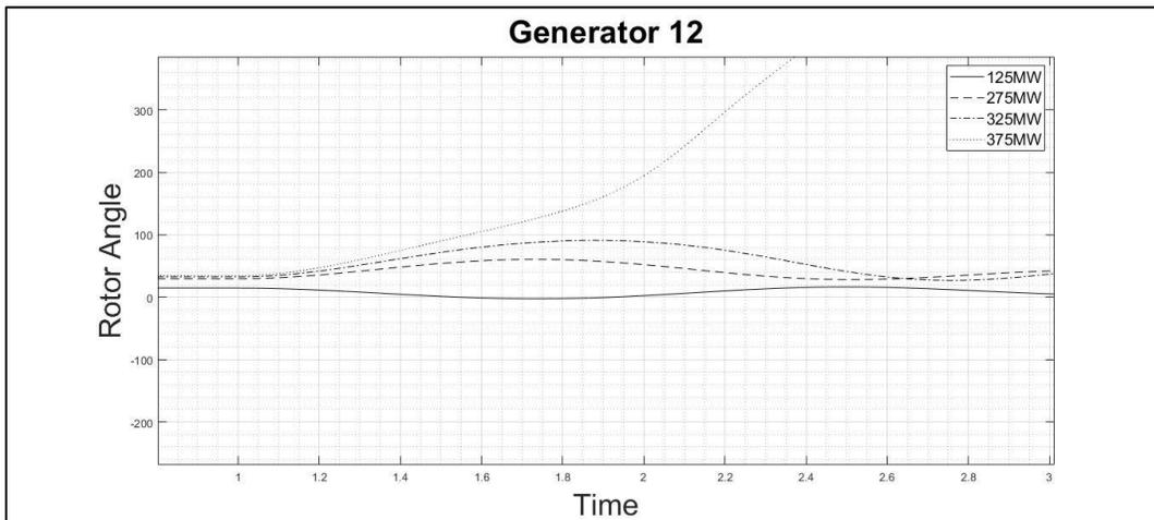
Figure 6.15 Rotor angle of the generator 12
