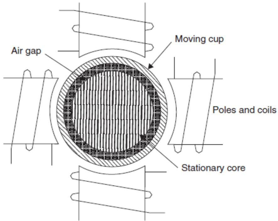
Figure 3.4 Moving cup induction relay [1]
