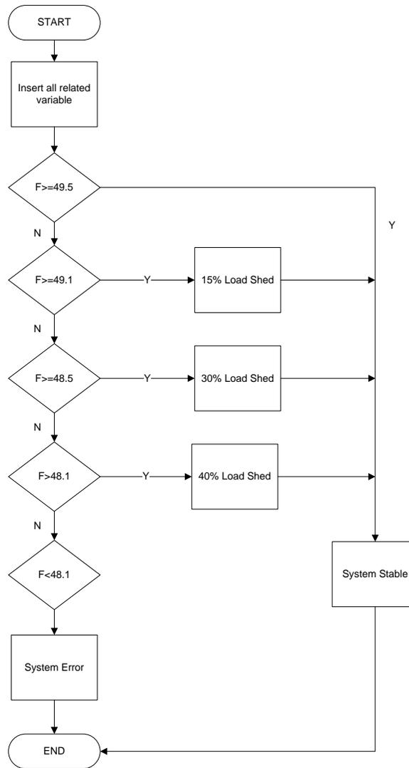
Figure 5.15 The process of underfrequency load shedding [27]
