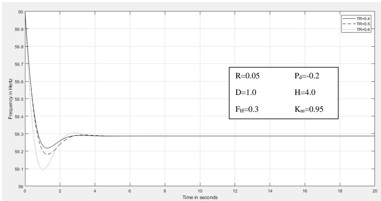
Figure 4.10. Frequency response for different amounts of  $T_R$
