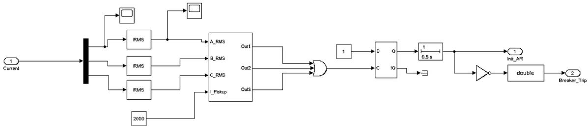
Figure 7.6 Definite time over-current relay subsystem
