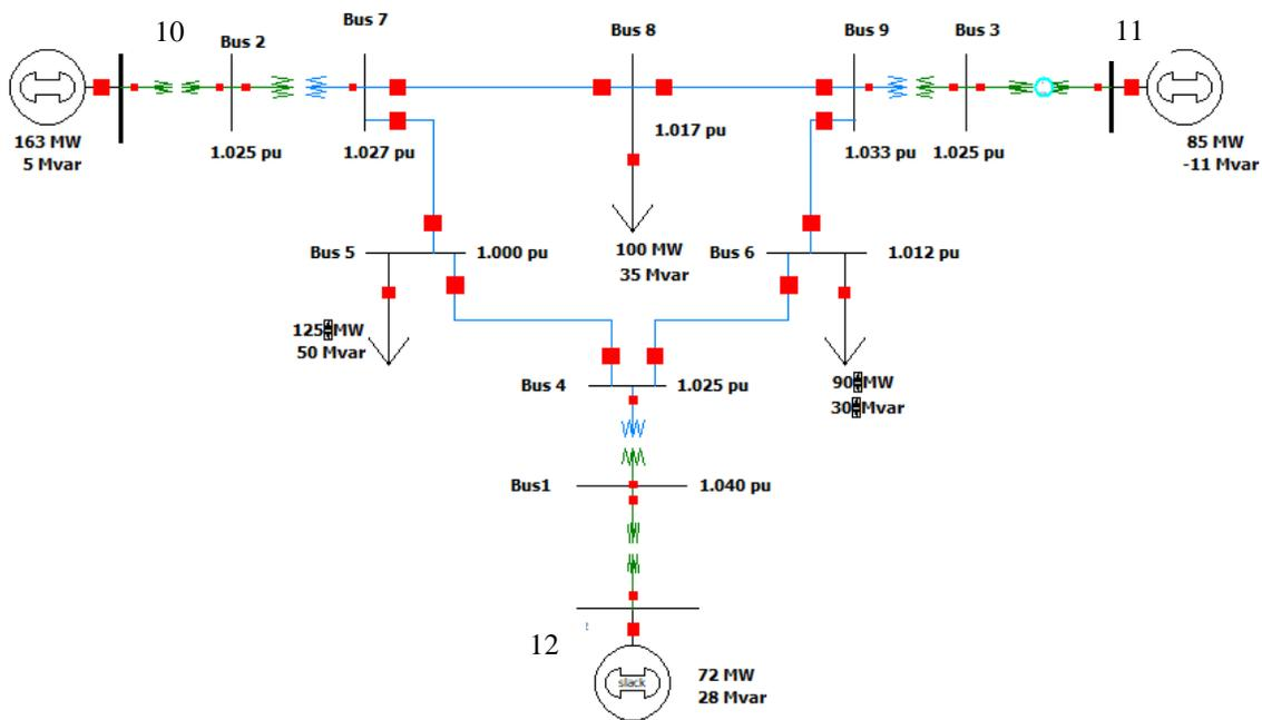
Figure 5.7 Standard IEEE 9-bus oneline diagram
