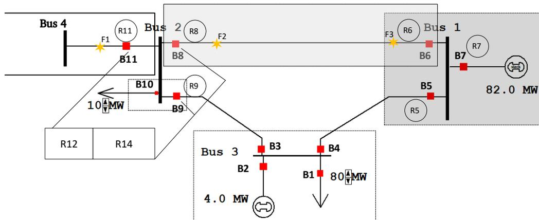
Figure 2.4. 3-bus designed power system protection
