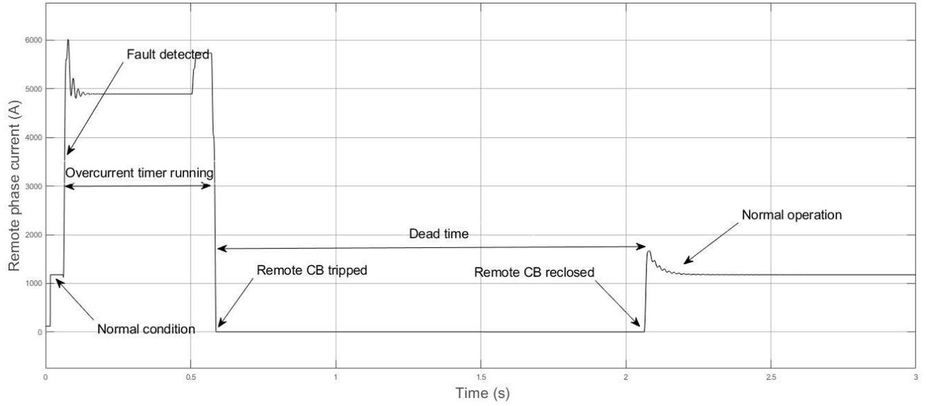
Figure 7.11 Line 2 rms current
