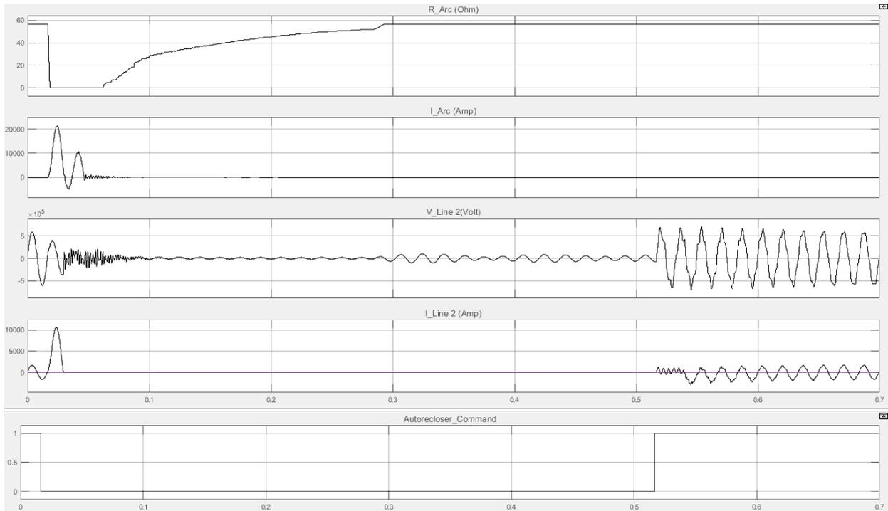
Figure 7.15 The result of arc and autoreclosing simulation
