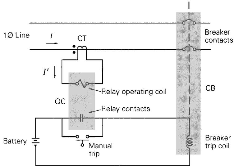
Figure 2.2 A sample over-current protective device [5]
