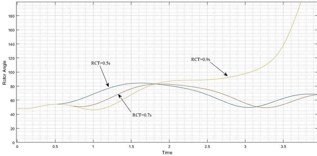
Figure 7.16 Rotor speed responses in each case of reclosing time
