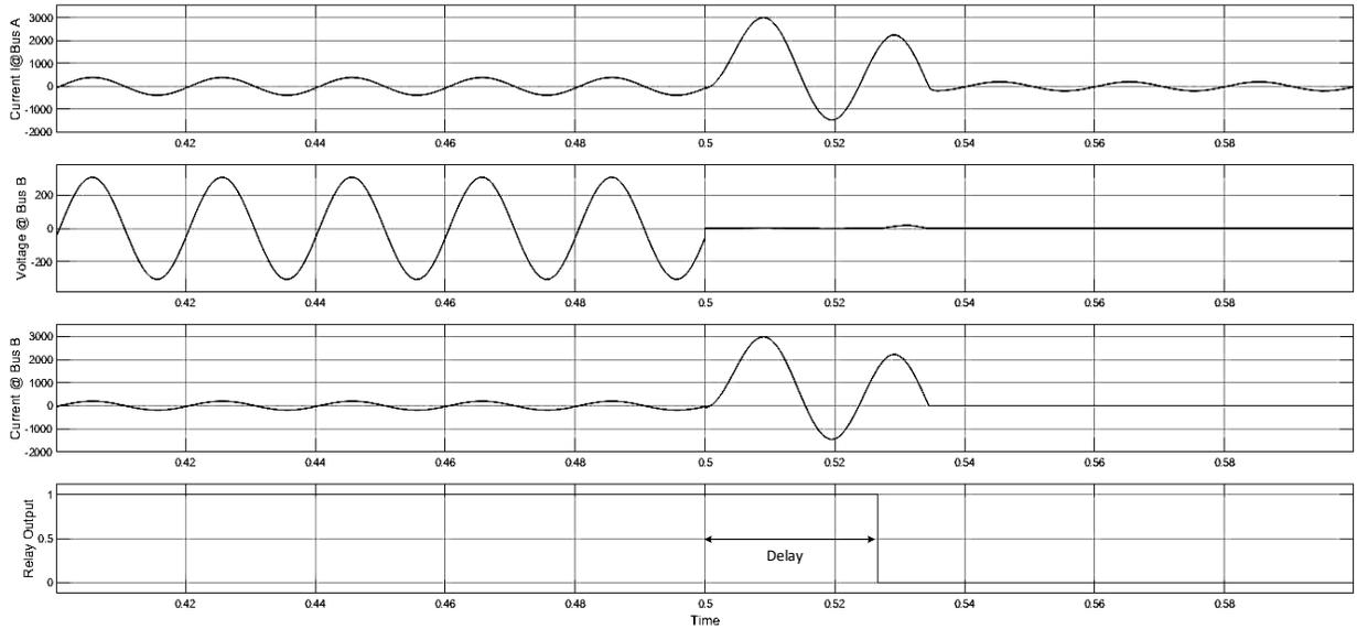
Figure 3.13 Waveforms of a digital solid-state instantaneous overcurrent relay
