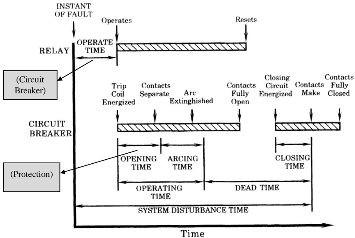
Figure 7.3 Single-shot autoreclose operation for a transient fault [1]
