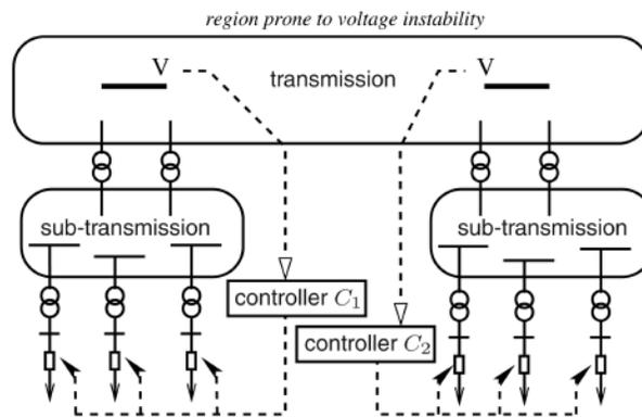
Figure 5.5 General structure of load shedding using DSC [19]
