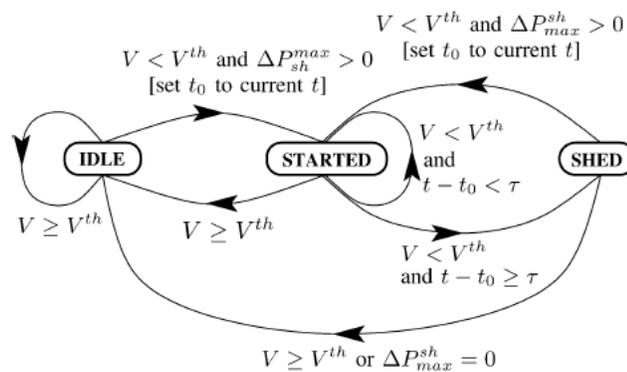
Figure 5.6 General structure of under-voltage load shedding [19]
