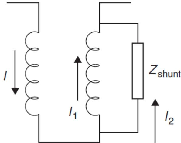
Figure 3.5 Inductive-type relay designed to perform as an overcurrent relay
