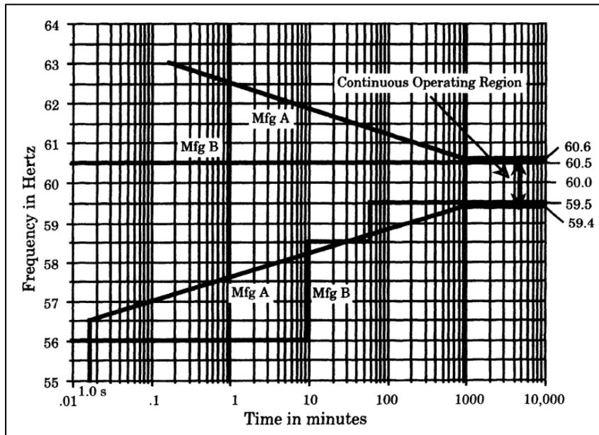
Figure 4.2. Turbine frequency lifetime [2]
