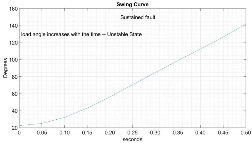
Figure 6.10 The plot of the Swing equation for a sustained fault (Unstable)
