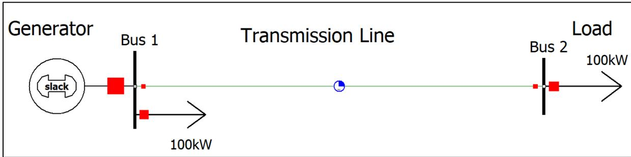
Figure 5.16 Oneline diagram of a two-bus power system
