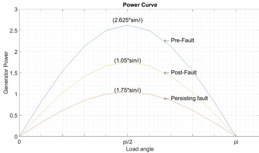
Figure 6.9 Power angle relation plot of the SMIB system example
