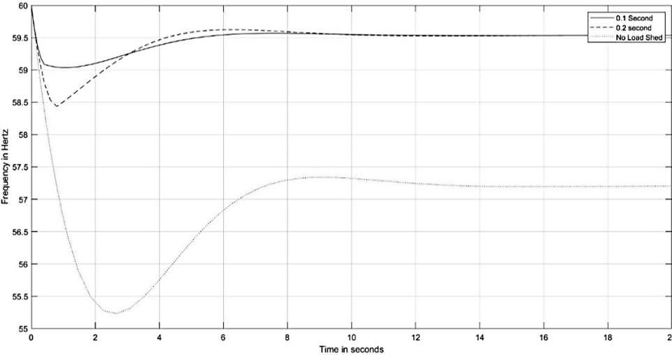
Figure 5.14 The effect of the Time Delay on UFLS
