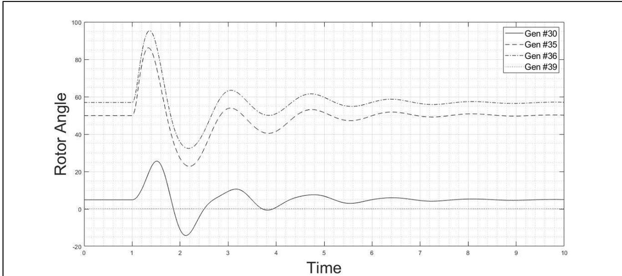
Figure 6.21 Rotor angle of the generators
