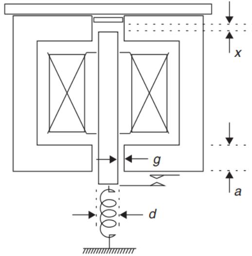
Figure 3.1 Plunger-type relay [1]
