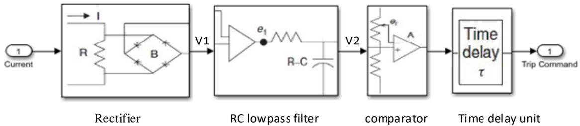
Figure 3.8 A sample blocks used for an analog solid-state instantaneous overcurrent relay
