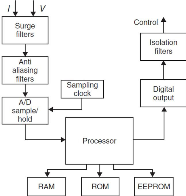
Figure 3.10 Major subsystems of a computer relay [1]
