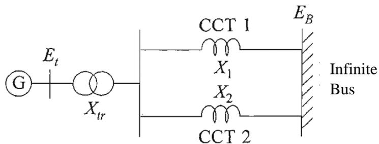
Figure 6.3 SMIB system with two transmission lines [33]
