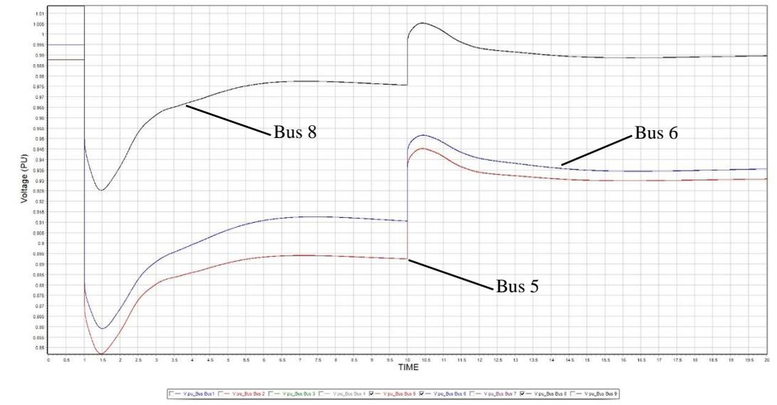
Figure 5.11 Voltage profile with adaptive load shedding
