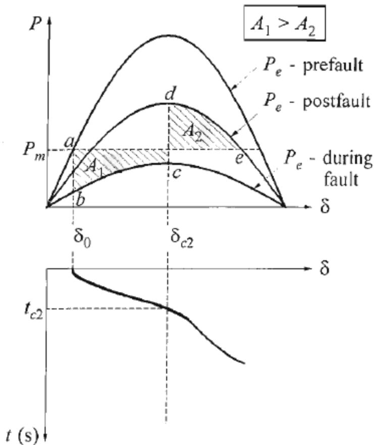
Figure 6.8 Power angle relation plot of SMIB (Unstable)[33]
