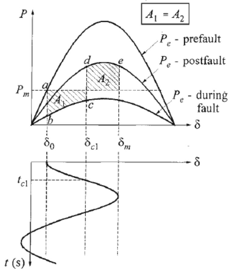
Figure 6.7 Power angle relation plot of SMIB (Stable) [33]
