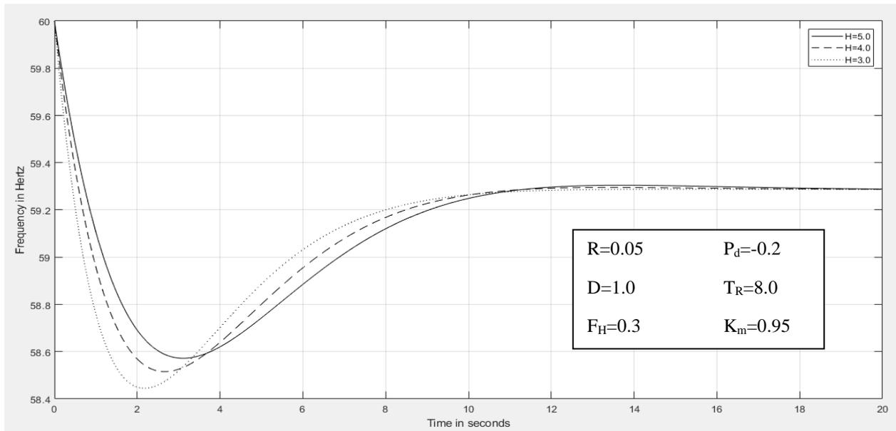
Figure 4.9. Frequency response for different amounts of H
