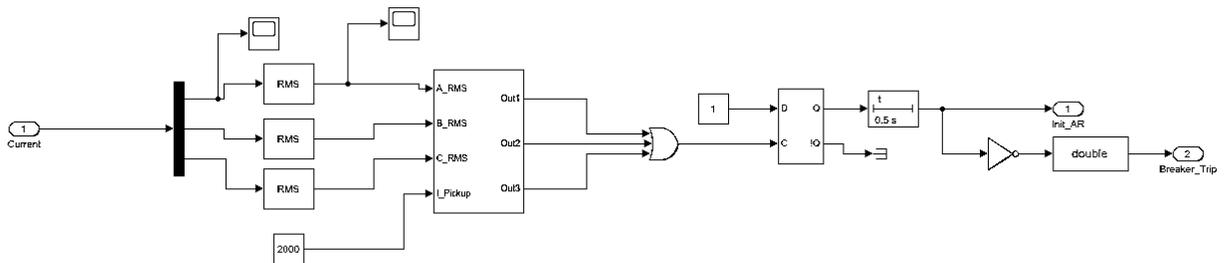
Figure 7.8 Definite time over-current relay subsystem
