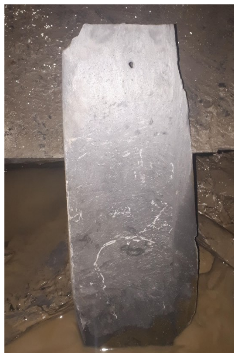
Figure 16: The fruits of our labour: a tile made from the material collected at Rhiwbach quarry, with a punctured nail hole at the top.
