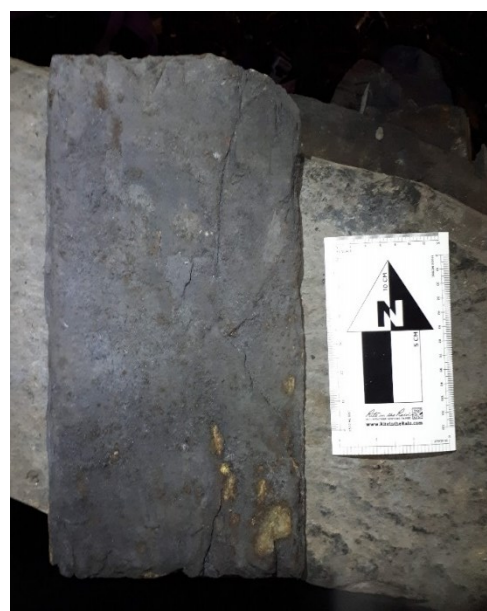
Figure 17: An unfinished slate from the Pen-y-Fridd quarry, with visible pyrite inclusions.
