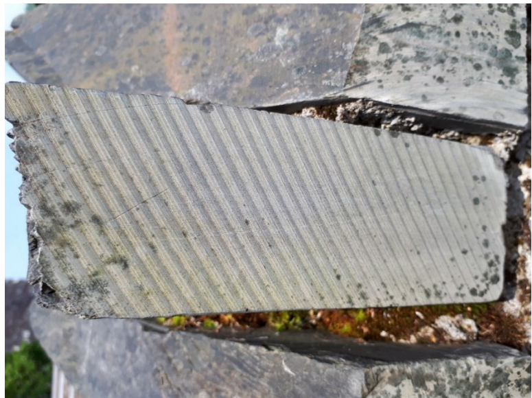
Figure 6: Striations on a circular sawn slate block.
