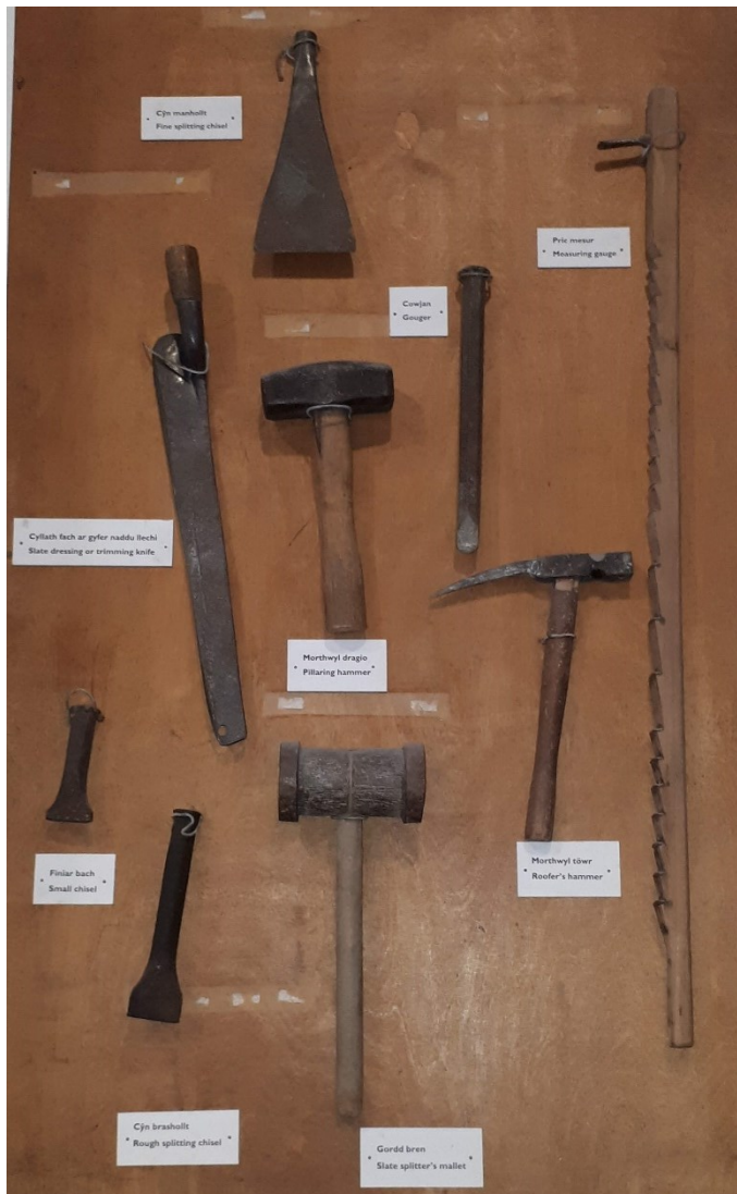
Figure 9: A collection of hand tools used by quarrymen. The pric mesur can be seen on the far right with a roofer's hammer to its left. A trimming knife and splitting chisel are on the far left.
