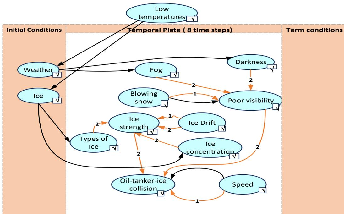
**Figure 3.3.** The DBN model of oil-tanker-ice collision for the Barents Sea (for winter navigation).
