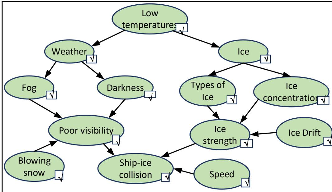
**Figure 3.2.** Ship-ice collision model for the winter navigation in Arctic waters
