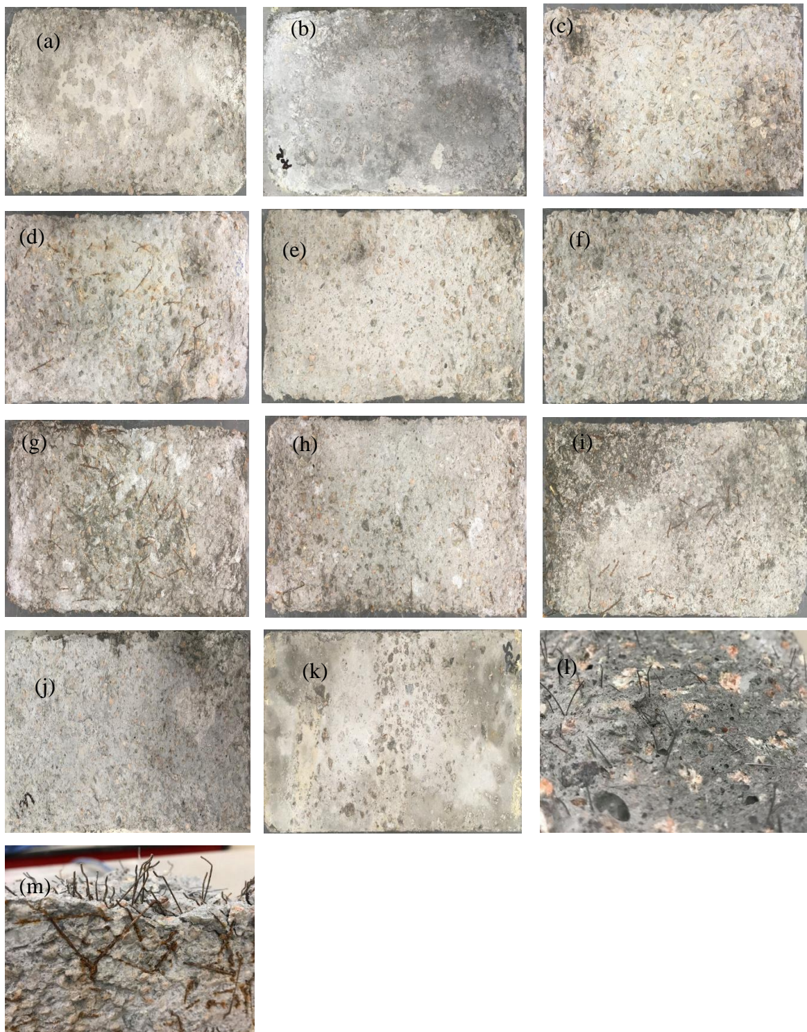
Figure 2-5 (a-k) Visual inspection of salt scaled specimens for the 11 mixtures after exposure to 50 cycles of salt scaling; (l and m) difference between SF13 and SF35 in corrosion resistance
