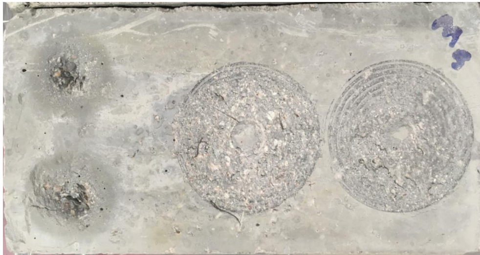
Figure 2-3 Tested specimen in abrasion test
