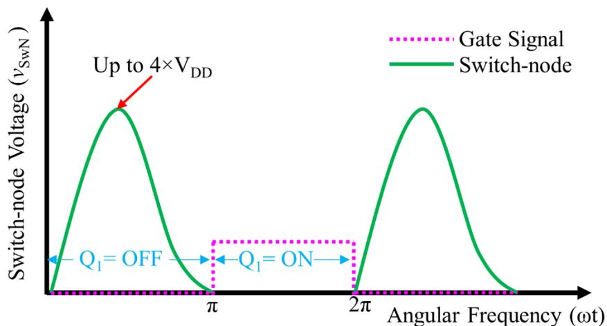
**Figure 2-2: Class-E inverter gate-source and switch-node waveforms**
