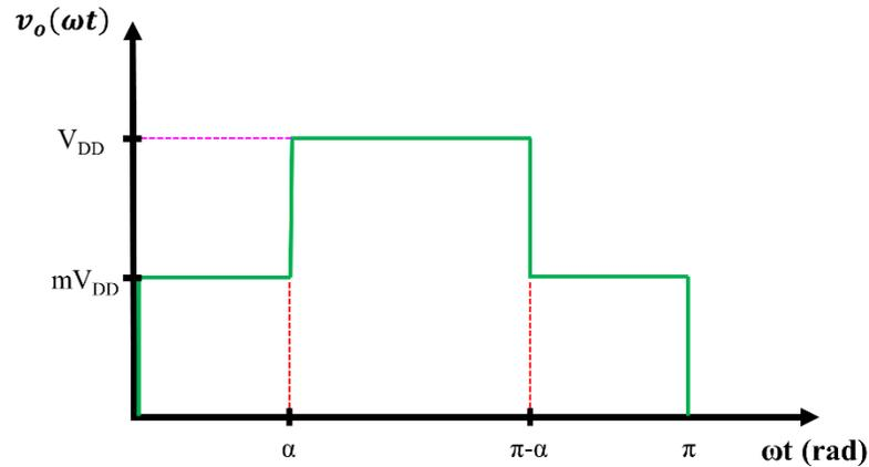
**Figure 5-1: Half cycle demonstration of an ideal stepped waveform with the possibility of zero 3<sup>rd</sup> and 5<sup>th</sup> harmonics**
