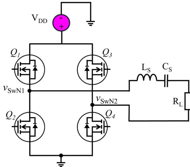
Figure 2-5: FB Class-D inverter
