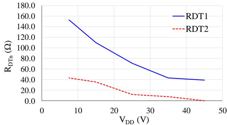
**Figure 4-7:  $R_{DT1}$  and  $R_{DT2}$  optimized values vs.  $V_{DD}$**
