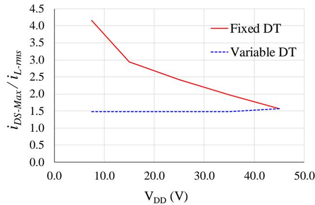
**Figure 3-14: Q<sub>1</sub> drain-source peak current over the RMS load current ( $i_{DS-Max}/i_{L-rms}$ )**
