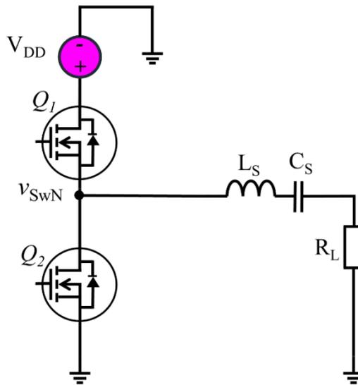
Figure 2-3: Circuit diagram of the Class-D half-bridge inverter
