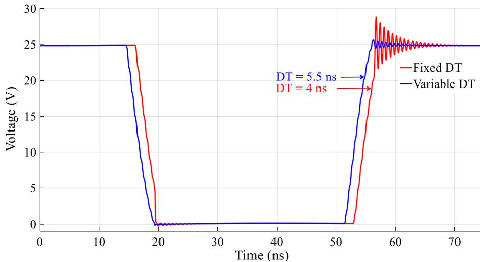
**Figure 3-10:**  $v_{SwN1}$  at  $V_{DD} = 25V$  with fixed DT and DDTC
