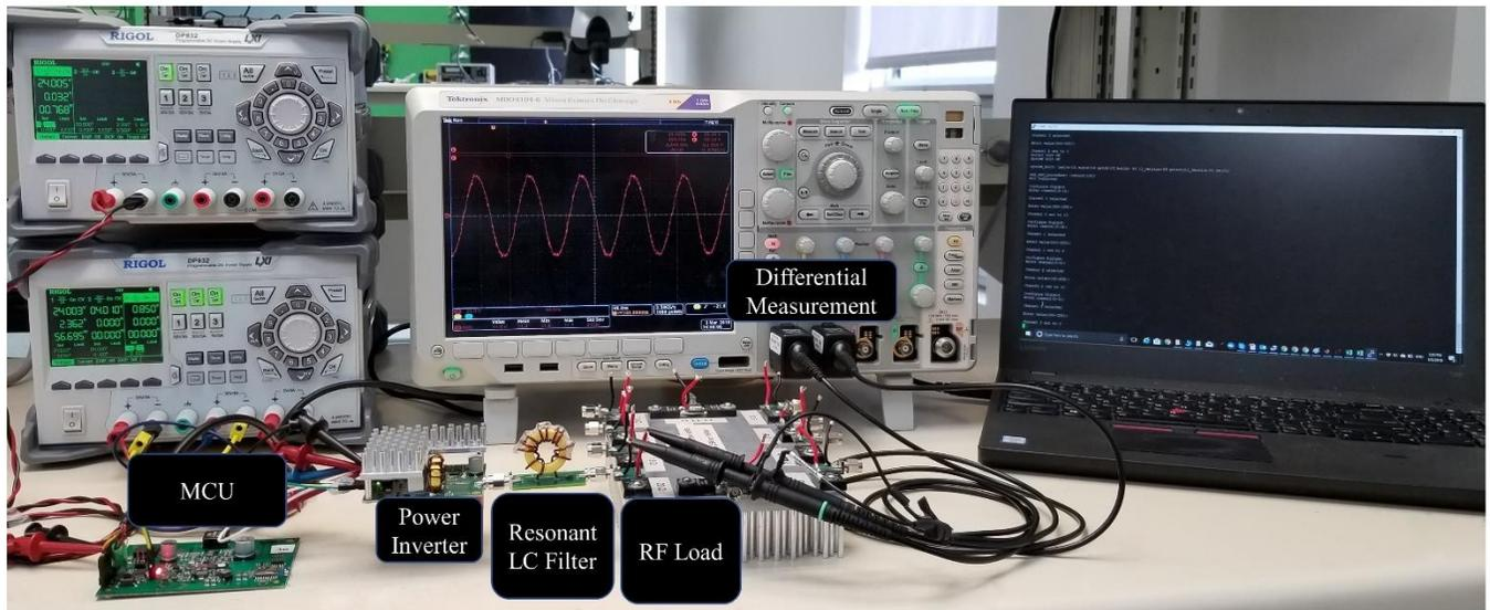
**Figure 4-6: Experimental test setup including MCU, inverter, resonant filter, and RF load**
