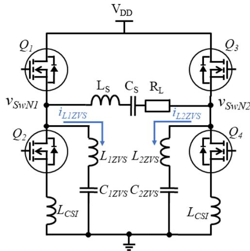
Figure 3-2: FB Class-D inverter with ZVS LC tank ( $L_{zvs}$  and  $C_{zvs}$ )
