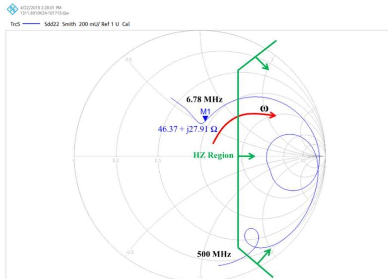
**Figure 5-20: Transformer input impedance on Smith Chart, secondary winding loaded with 50 $\Omega$**
