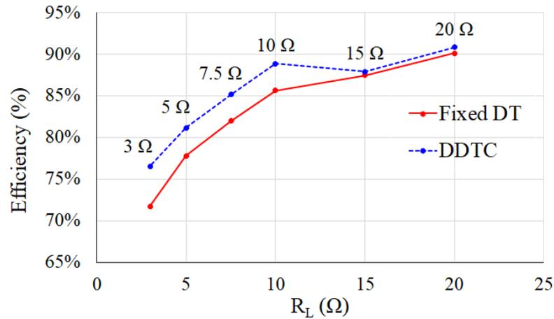
**Figure 4-13: FB Class-D power inverter efficiency at fixed 40W output power delivered to various  $R_L$**
