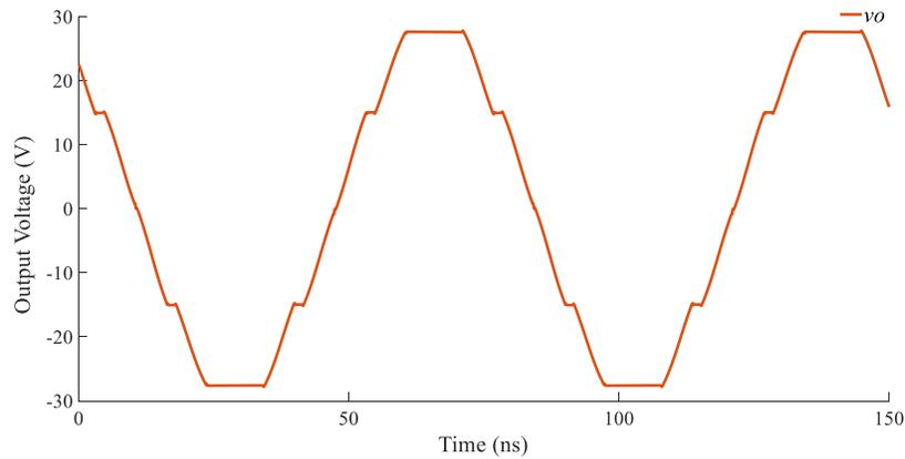
**Figure 5-7: Output voltage of the multi-level inverter,  $DT = 6$  ns,  $m = 0.5442$ , and  $\alpha = 35.23^\circ$**
