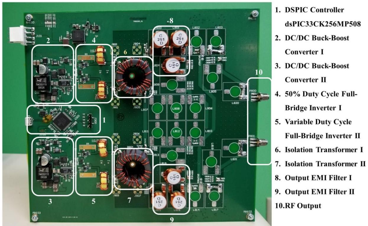
Figure 5-15: Multi-level prototype PCB implementation, 204 mm × 189 mm
