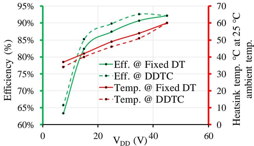
**Figure 4-12: FB Class-D power inverter efficiency and heatsink temperature with fixed DT and DDTC at different DC voltage levels**
