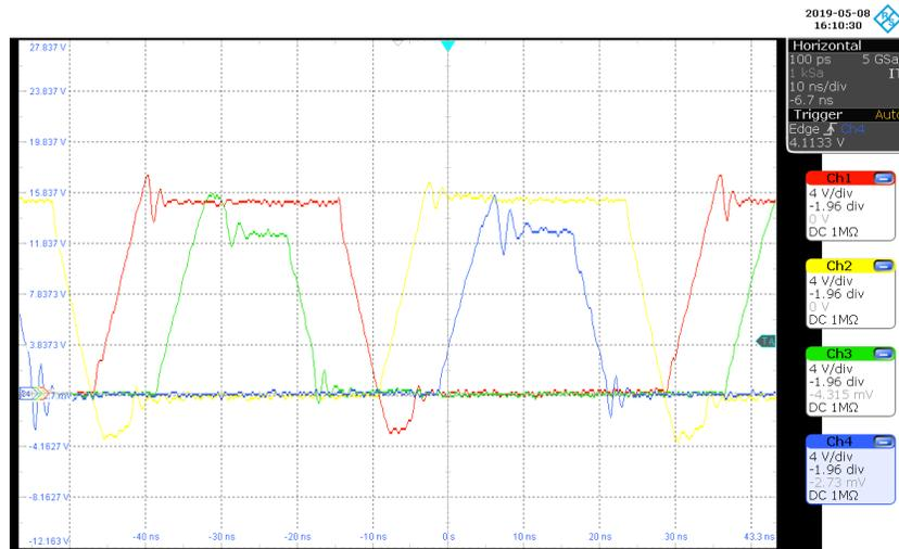
**Figure 5-17: Multi-level inverter individual Switch-nodes,  $m = 0.54$ ,  $\alpha = 35.32^\circ$ ,  $V_{DC1} = 15V$ , and  $V_{DC2} = 12.6V$**
