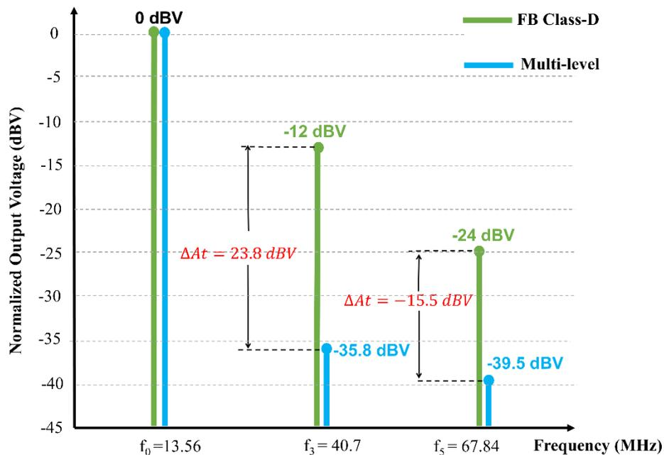
**Figure 5-19: Normalized output voltage harmonic comparison between multi-level and FB Class-D inverter using experimental results**
