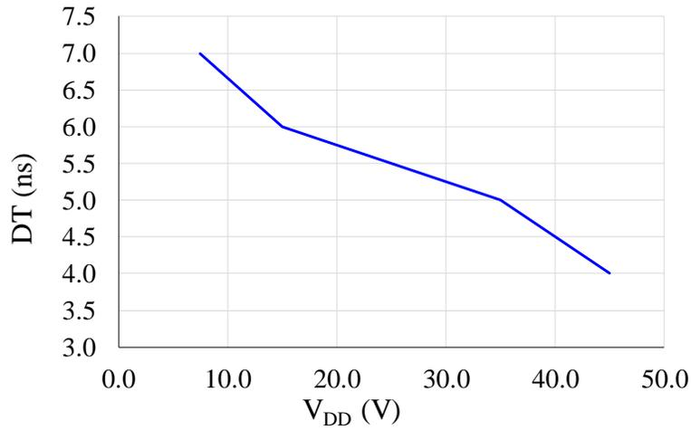
**Figure 3-12: The range of DT for soft-switching vs. V<sub>DD</sub>**
