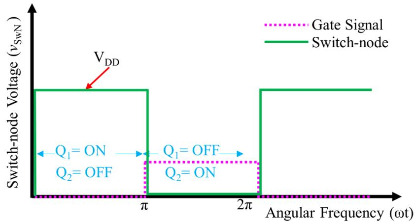
Figure 2-4: Class-D gate and switch-node waveforms
