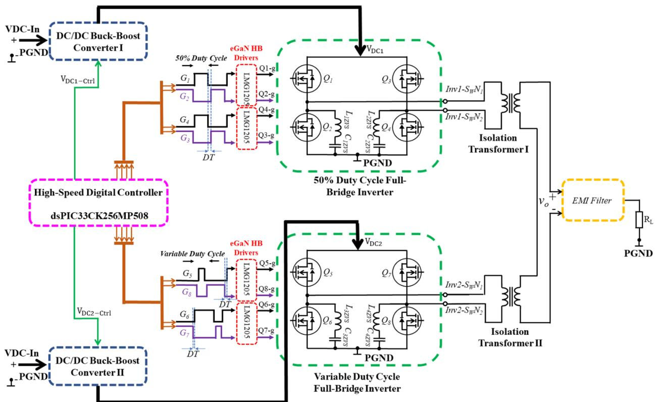
Figure 5-14: Multi-MHz multi-level inverter hardware block diagram
