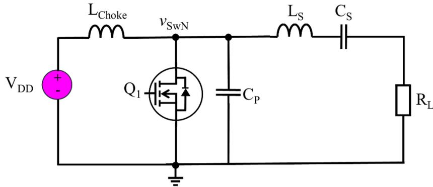
**Figure 2-1: Circuit diagram of the classic Class-E inverter**
