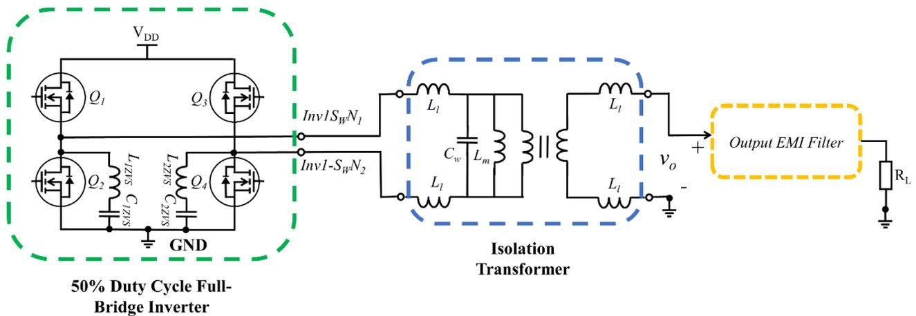
Figure 5-22: Isolation transformer detailed circuit modeling with parasitic components
