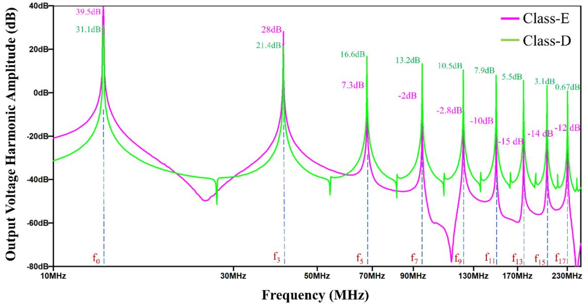
Figure 2-6: FB Class-D and Class-E push-pull output voltage harmonic analysis
