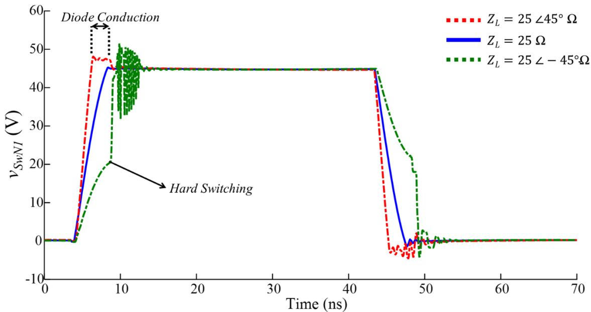
**Figure 3-15: Switch-node 1 voltage ( $V_{SwN1}$ ) under different loading conditions**
