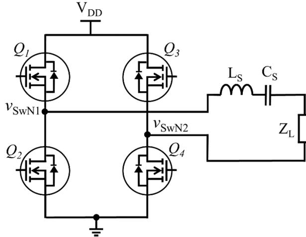
Figure 3-1: FB Class-D inverter with series resonant filter and load
