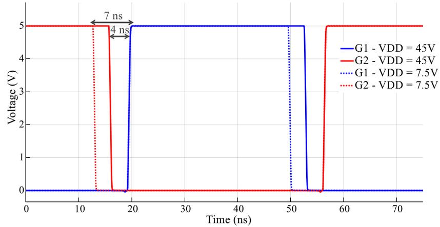
**Figure 3-5: G<sub>1</sub> and G<sub>2</sub> gate signals at V<sub>DD</sub> = 7.5V and 45V**
