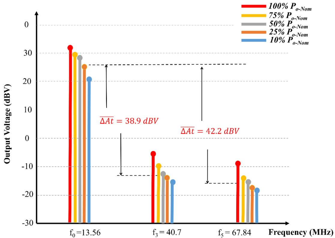
Figure 5-12: Multi-level inverter output voltage harmonic analysis during output power regulation
