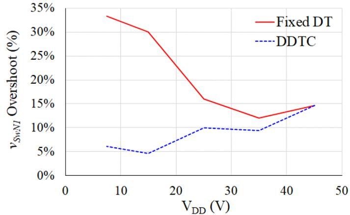
**Figure 4-11: Switch-node 1 ( $v_{SwN1}$ ) overshoot at different  $V_{DD}$  levels**
