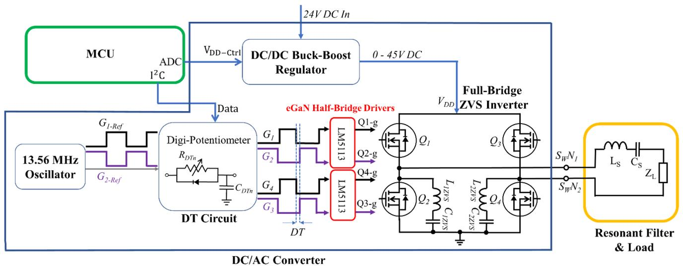
Figure 4-4: DDTC hardware block diagram
