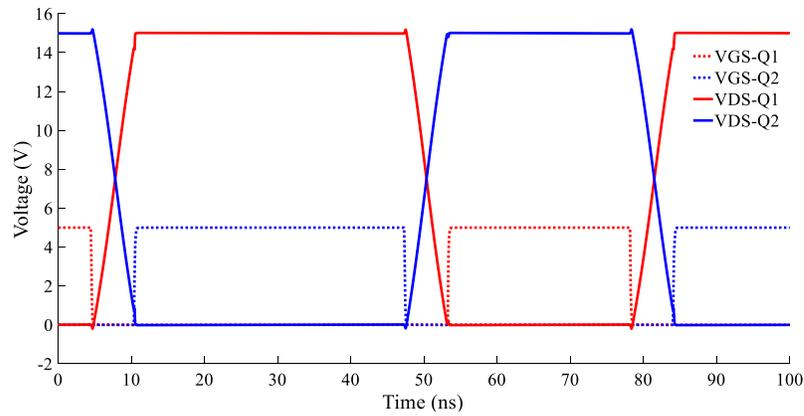
**Figure 5-5: Gate and drain-source voltages of  $Q_1$  and  $Q_2$**
