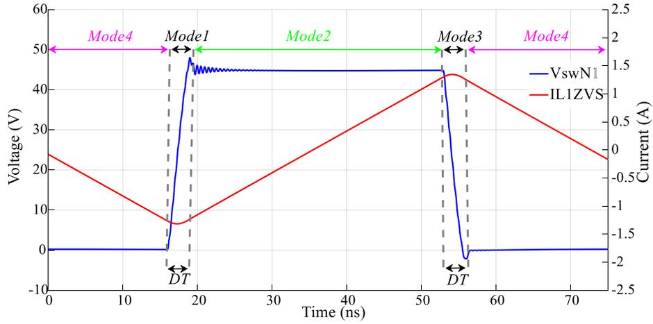
**Figure 3-4:  $v_{swN1}$  and  $i_{L1ZVS}$  waveforms**
