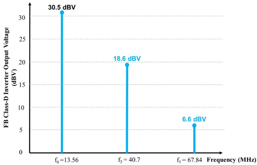
**Figure 4-14: Class-D inverter output voltage harmonic analysis**
