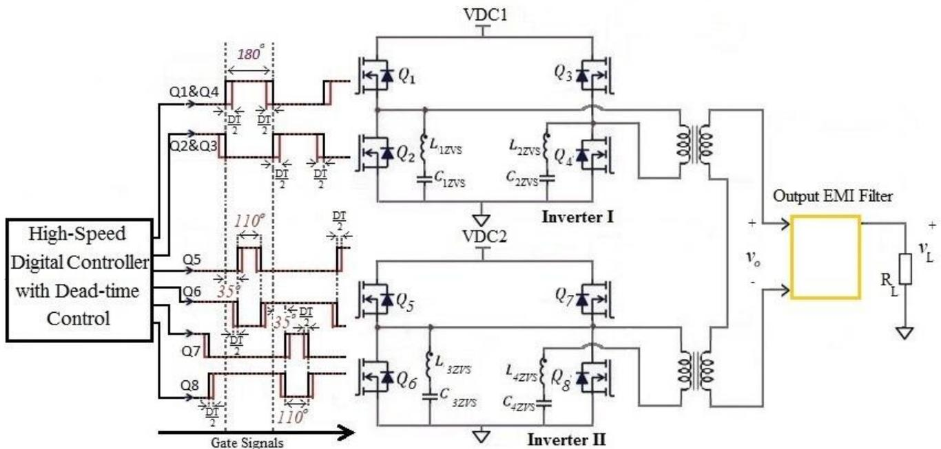
**Figure 5-4: Multi-level ZVS inverter with DDTC, Inverter II gate signals at  $\alpha = 35^\circ$**
