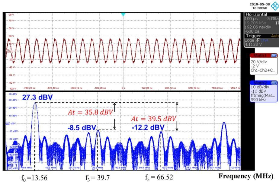
**Figure 5-18: Multi-level inverter output voltage waveform and harmonic analysis**
