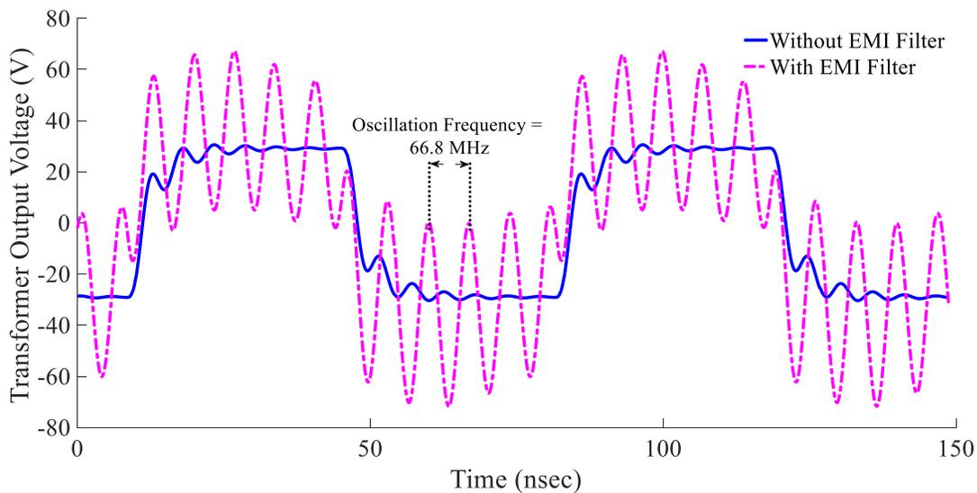
**Figure 5-23: Simulating EMI filter impact on the isolation transformer output voltage ( $v_o$ ) waveform using the transformer detailed model**
