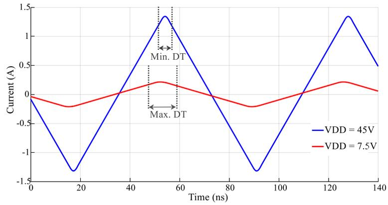
**Figure 3-7:  $L_{1ZVS}$  current at  $V_{DD} = 7.5V$  and  $45V$**
