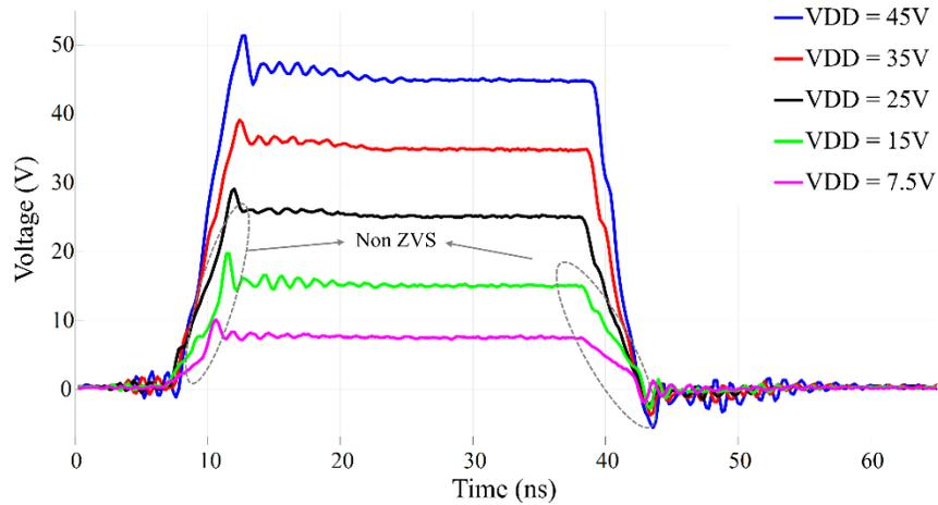
**Figure 4-9:**  $v_{swN1}$  waveform at different  $V_{DD}$  levels with fixed DT
