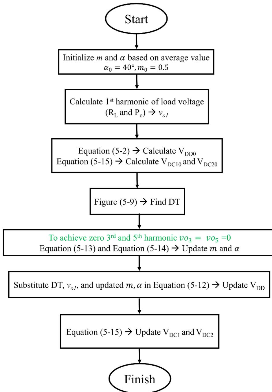
**Figure 5-10: Multi-level inverter output voltage regulation algorithm using DDTC**
