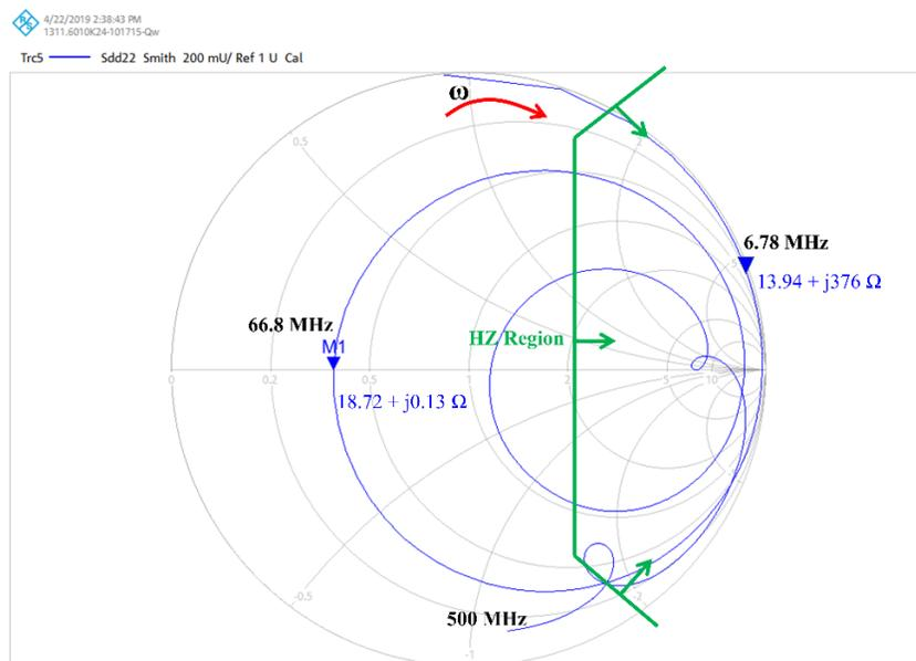
**Figure 5-21: Transformer input impedance on Smith Chart, secondary winding open-circuited**
