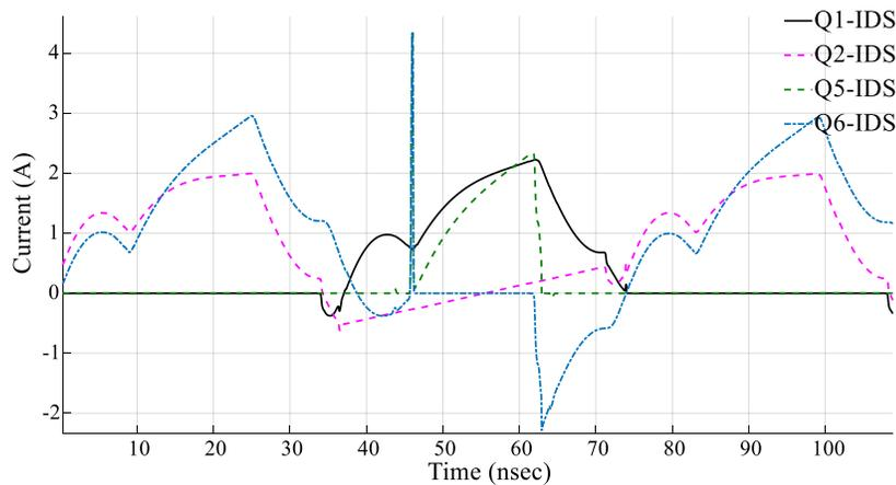
**Figure 5-13: Drain-source currents of the switches at full load ( $P_{o-Nom}$ )**
