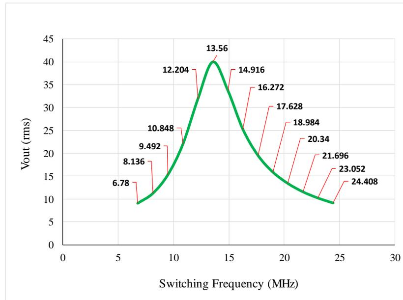
**Figure 4-1: Class-D inverter output voltage regulation with switching frequency modulation, 13.56 MHz center frequency**
