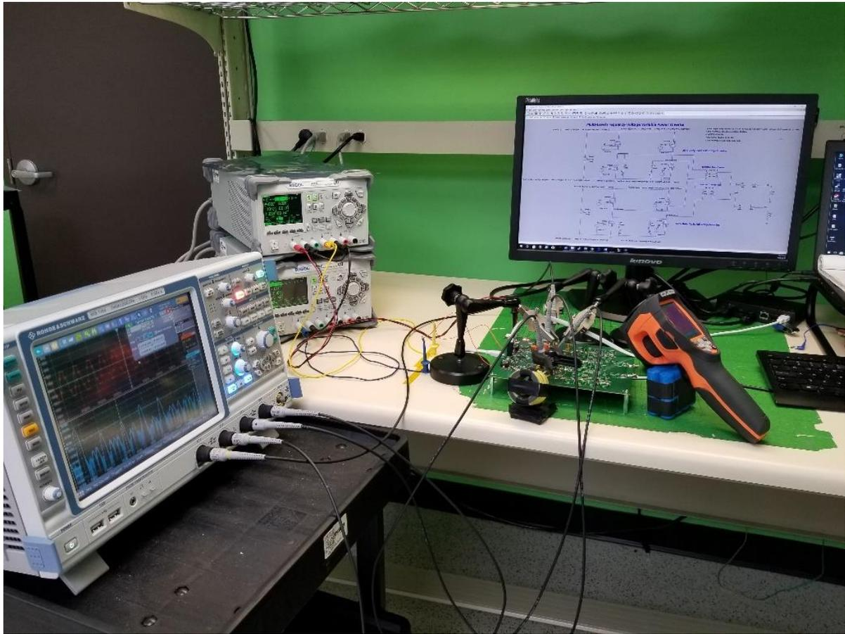
**Figure 5-16: Multi-level inverter experimental setup**
