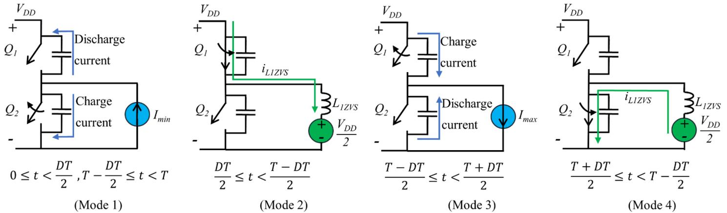
**Figure 3-3: Operation modes of the half-bridge inverter with ZVS tank**
