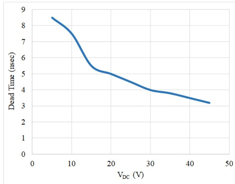
**Figure 5-9: DT variation at different  $V_{DC}$  levels for soft-switching**
