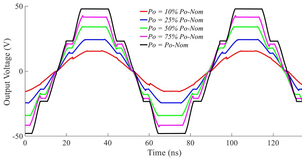
Figure 5-11: Multi-level inverter output voltage regulation with DDTc
