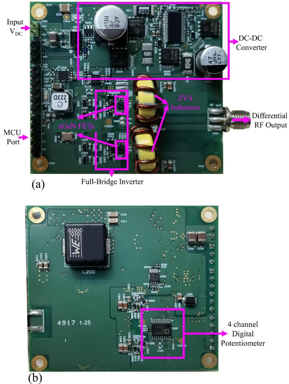
Figure 4-5: Experimental prototype of the DC/AC converter, 61 mm  $\times$  54 mm: (a) top layer, (b) bottom layer
