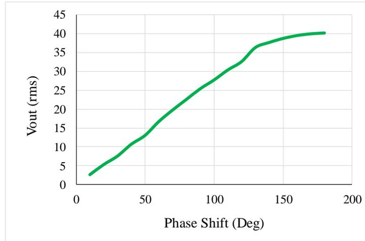
**Figure 4-3: FB Class-D inverter output voltage control with phase-shift**
