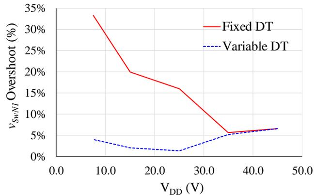
**Figure 3-13: Switch-node 1 voltage ( $v_{SwN1}$ ) overshoot at different V<sub>DD</sub> levels**
