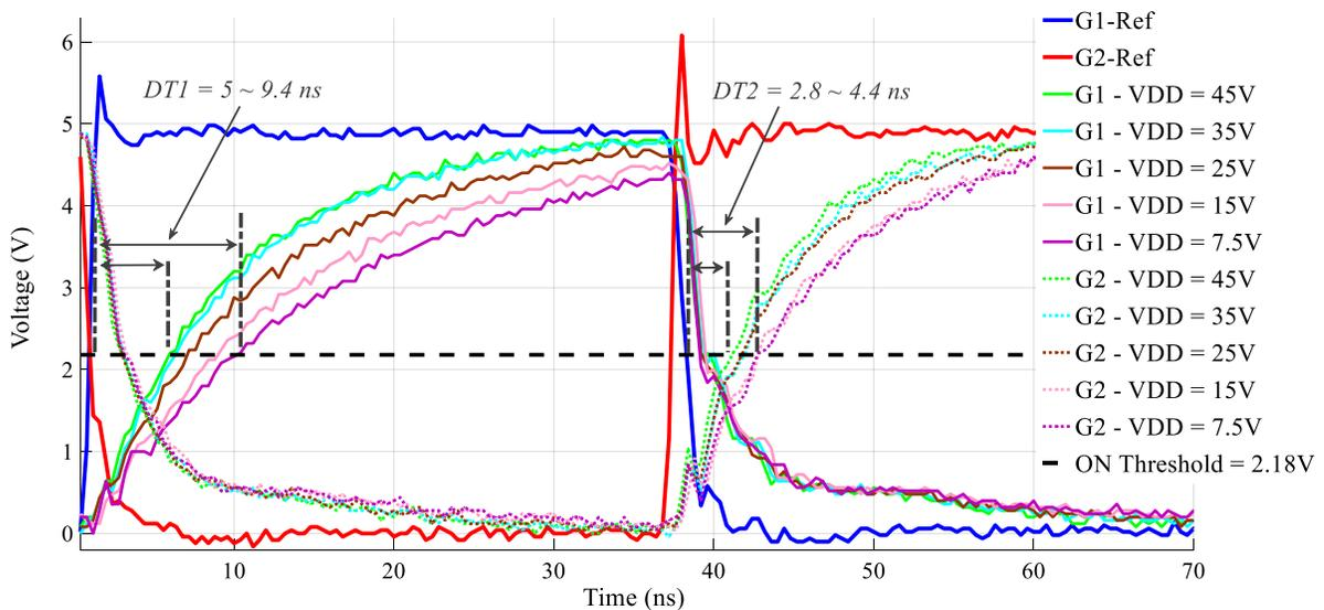
**Figure 4-8:**  $G_{1-Ref}$ ,  $G_{2-Ref}$ ,  $G_1$ , and  $G_2$  references and gate signals at different  $V_{DD}$  levels
