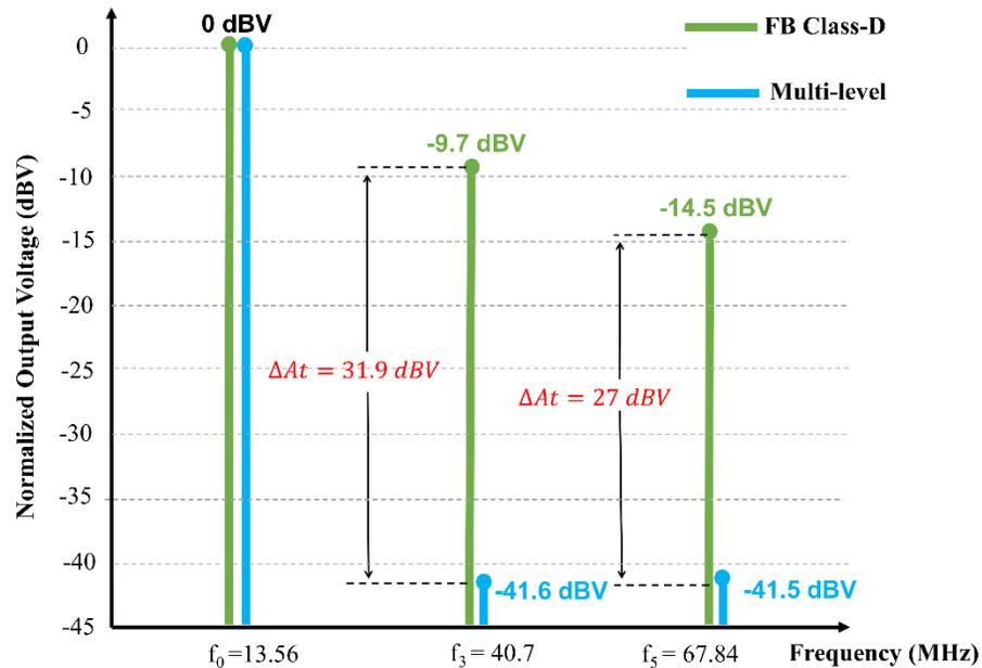
**Figure 5-8: Comparing normalized harmonic analysis on the output voltage between multi-level and FB Class-D inverters**
