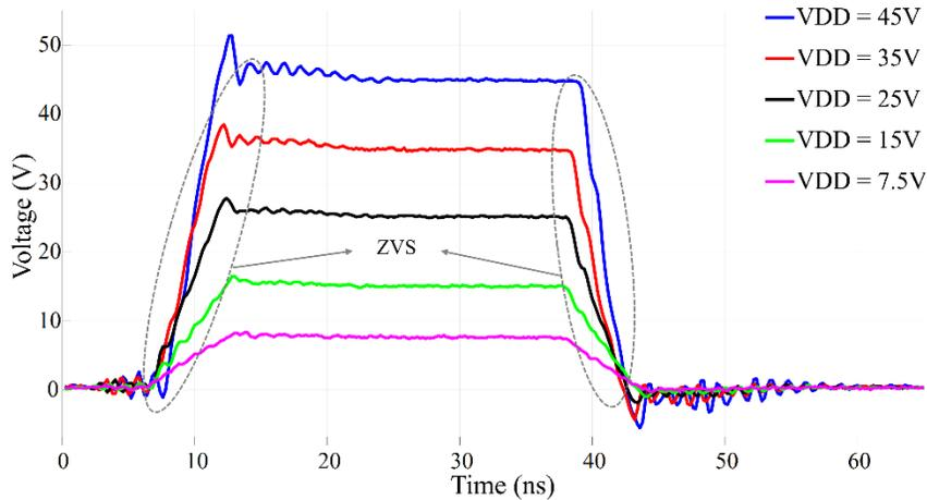
**Figure 4-10:**  $v_{SW/NL}$  waveform at different  $V_{DD}$  levels with DDTC
