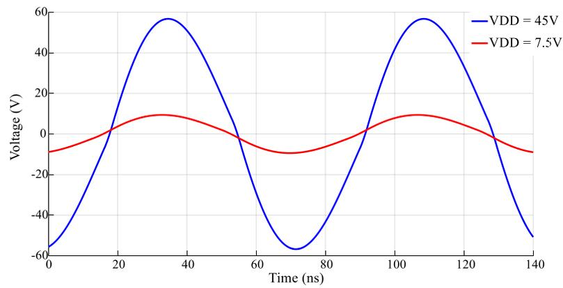
**Figure 3-9: Load voltage at  $V_{DD} = 7.5V$  and  $45V$**
