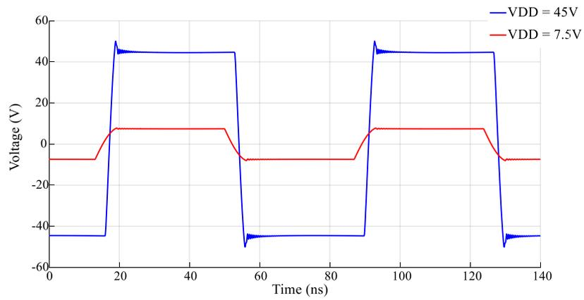
**Figure 3-8: Switch-node differential voltage ( $v_{Sw}$ ) at  $V_{DD} = 7.5V$  and  $45V$**
