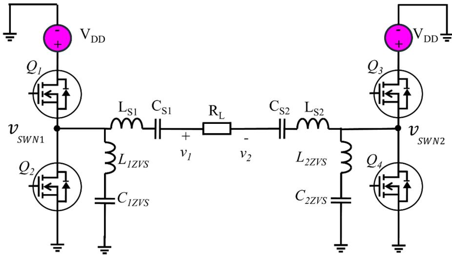
Figure 4-2: ZVS FB Class-D inverter with phase-shift control
