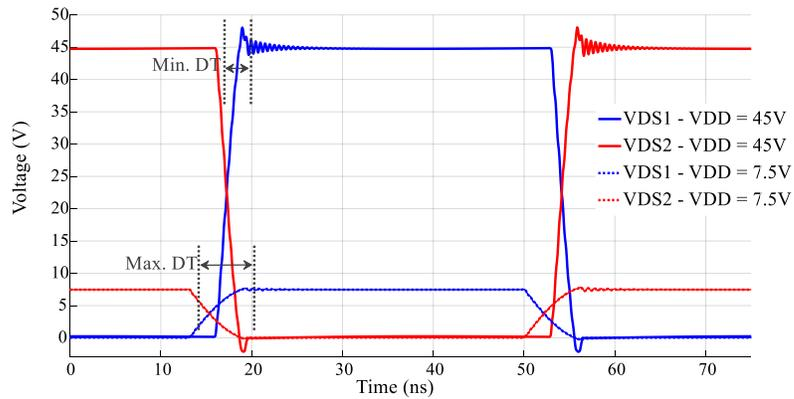
**Figure 3-6: Q<sub>1</sub> and Q<sub>2</sub> drain-source voltage at V<sub>DD</sub> = 7.5V and 45V**
