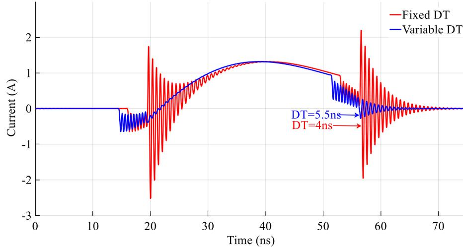
**Figure 3-11: Q<sub>1</sub> drain-source current at  $V_{DD} = 25V$  with fixed and variable DT**
