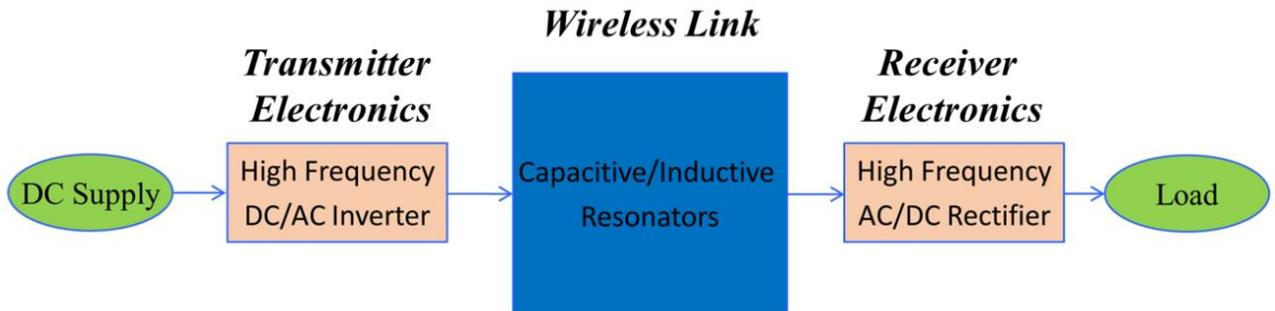
**Figure 1-1: Typical wireless power system block diagram**
