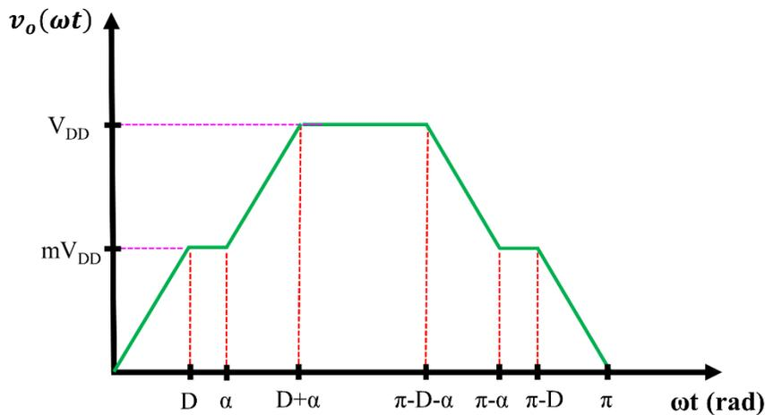
**Figure 5-2: Half cycle of the stepped waveform with the possibility of zero 3<sup>rd</sup> and 5<sup>th</sup> harmonics**
