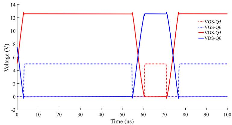
**Figure 5-6: Gate and drain-source voltages of  $Q_5$  and  $Q_6$**
