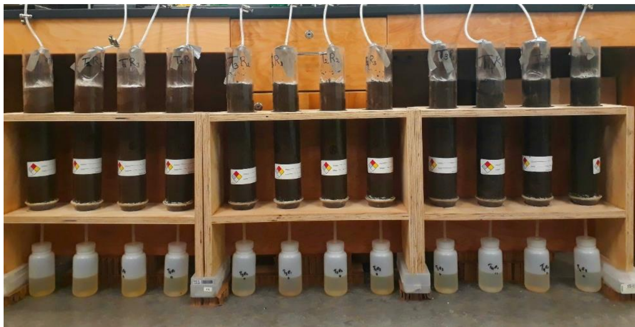
Figure 2.3: The front view of the experimental setup showing the leaching columns and the leachate collecting system
