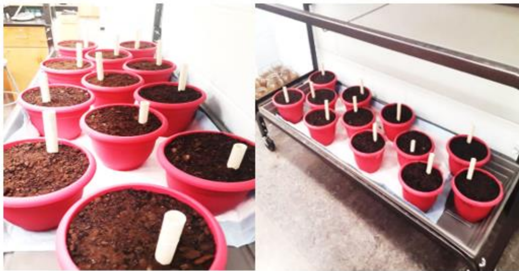
Figure 2.6: Pot experiment showing each pot filled with fly-ash amended soil with different % of biochar
