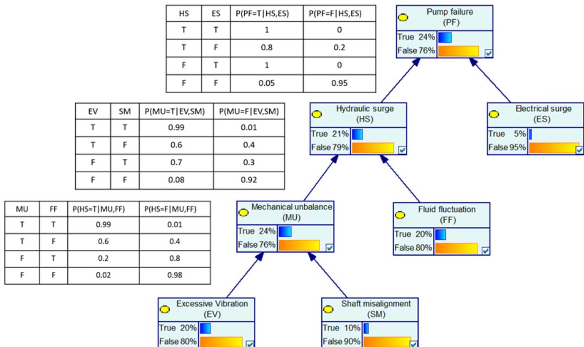
**Figure 3. 12 Bayesian network for pump failure scenario.**
