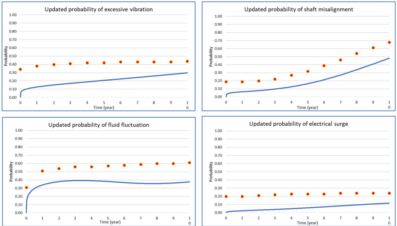
**Figure 3. 14 Temporal evolution of updated probabilities using DBN (red dots) and BSPN (blue line)**
