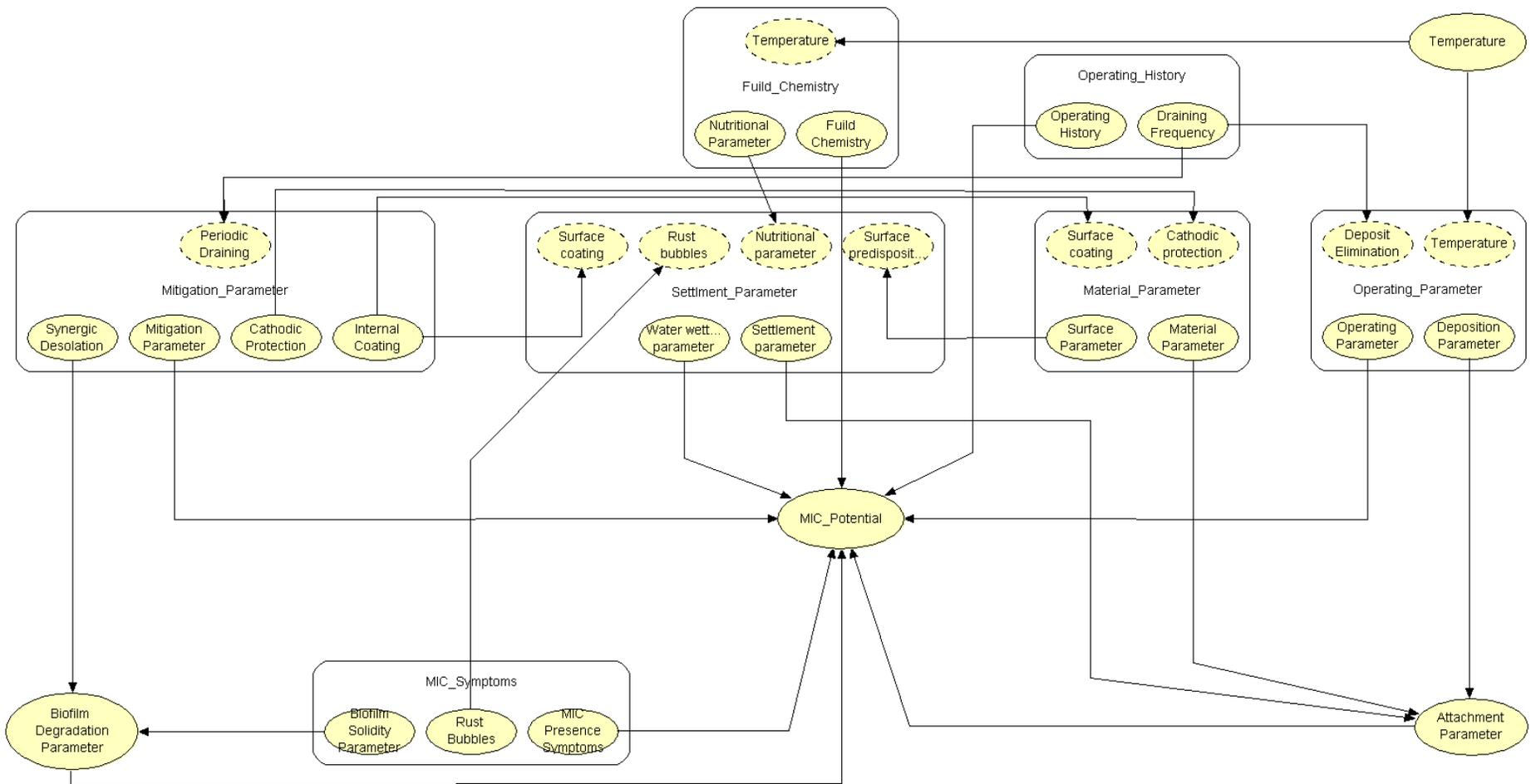
**Figure 2. 9 The overall OOBN model for the MIC potential assessment showing the interactions among the sub-network**
