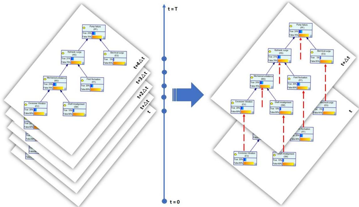
Figure 3. 13 Dynamic Bayesian network for pump failure scenario
