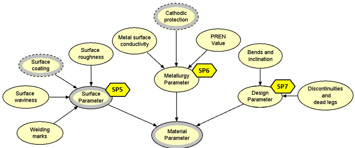
**Figure 2. 4 OOBN sub-network of the metallurgy and the surface factors that influence the MIC potential and their interactions**
