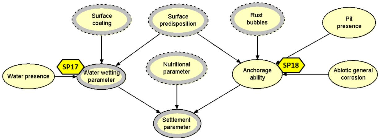
**Figure 2. 8 OOBN sub-network of the settlement factors that influence the MIC potential and their interactions**
