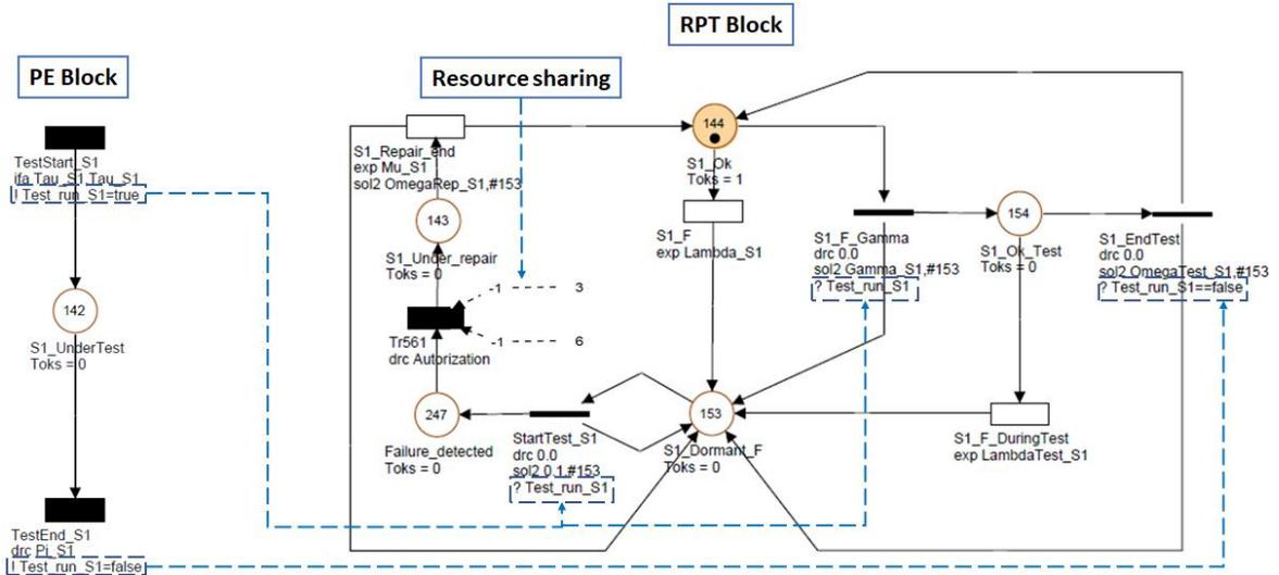
**Figure 5.1. 2 RPT and PE bocks and their virtual connections through the Boolean functions**
