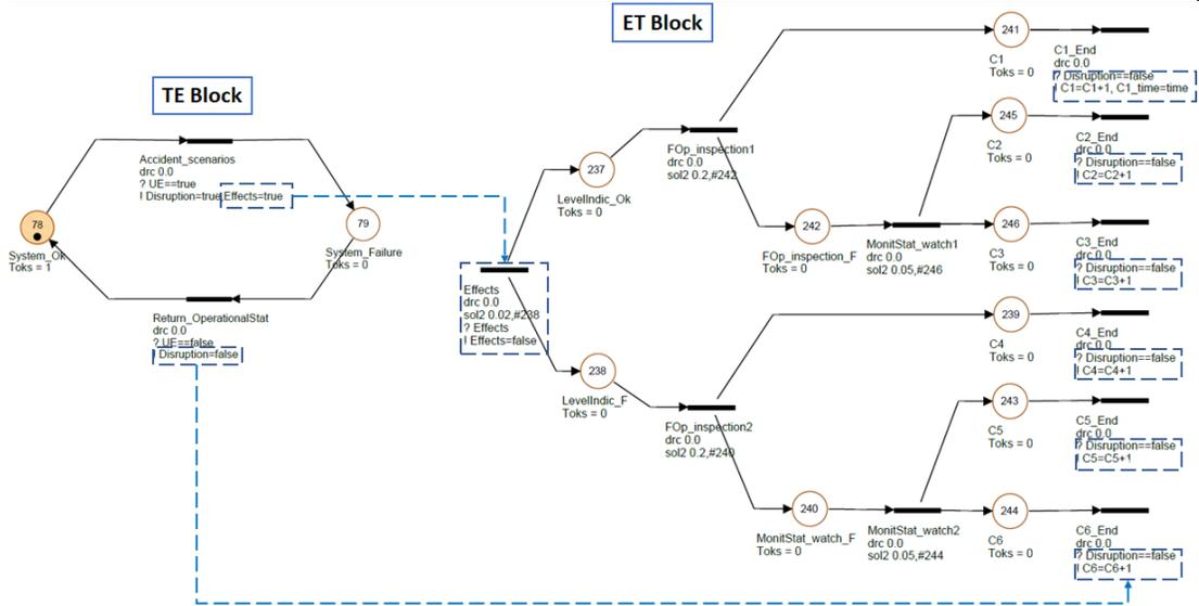
Figure 5.1. 3 TE and ET blocks and their virtual connections through the Boolean functions
