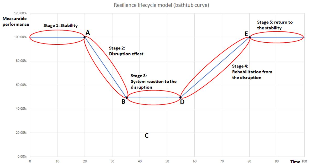
**Figure 5.2. 1 The proposed resilience lifecycle model (bathtub curve)**
