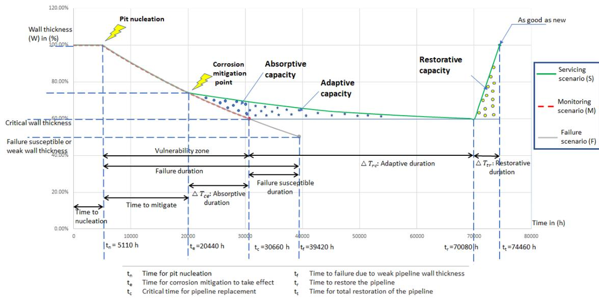
**Figure 5.2. 4 Resilience curve for pipeline corrosion control**
