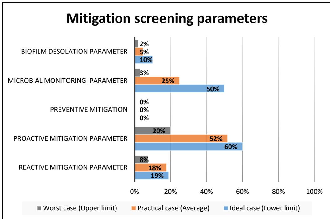
**Figure 2. 12 Efficiency of the mitigation practices for MIC attenuation**
