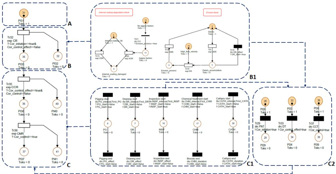
**Figure 5.2. 3 SPN overall network for the pipeline resilience modelling**
