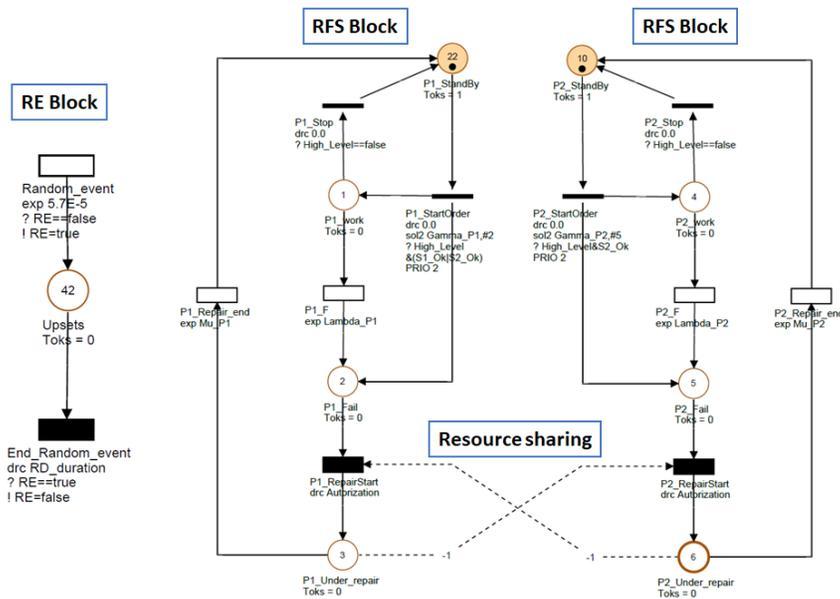
Figure 5.1. 4 RE and RFS blocks and the resource sharing between two RFS blocks (redundant system)
