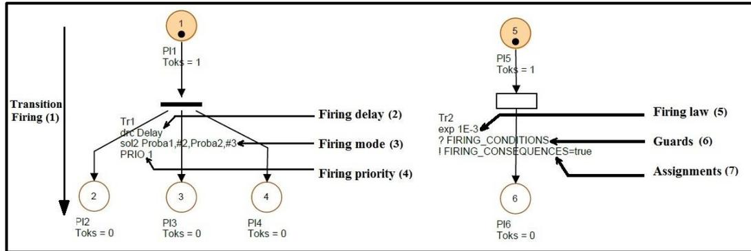
**Figure 3. 4 Display of the characteristics of the SPN with predicates and assertions**
