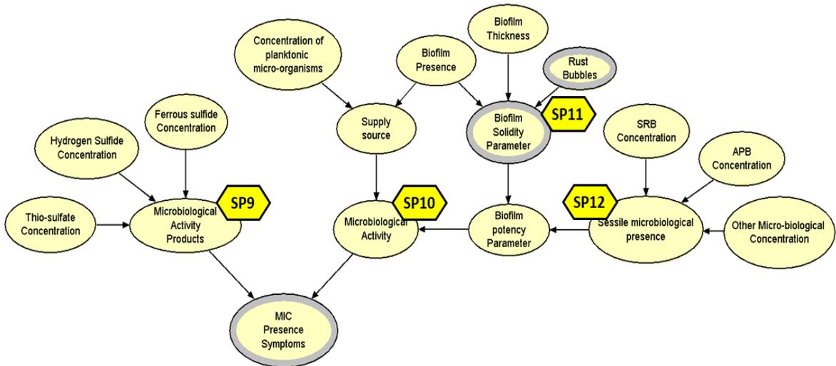
**Figure 2. 6 OOBN sub-network of the MIC presence symptoms and their interactions**
