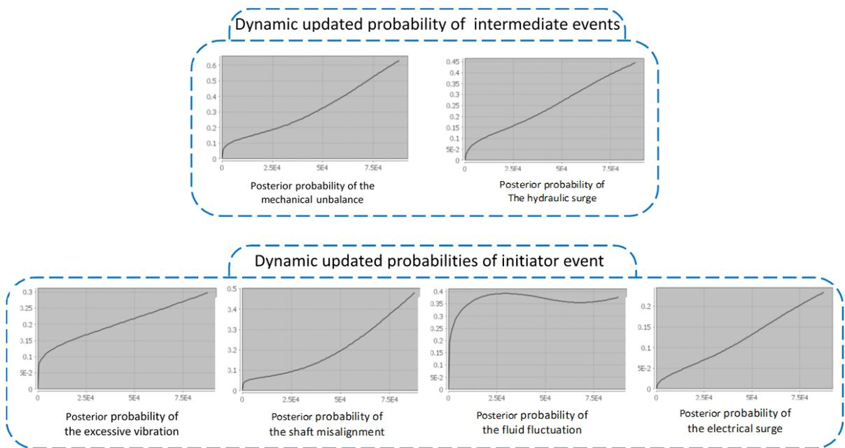
**Figure 3. 10 BSPN output data for the pump failure scenario**
