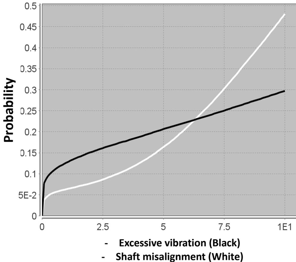
**Figure 3. 11 Trends of posterior probabilities of excessive vibrations versus shaft misalignment**
