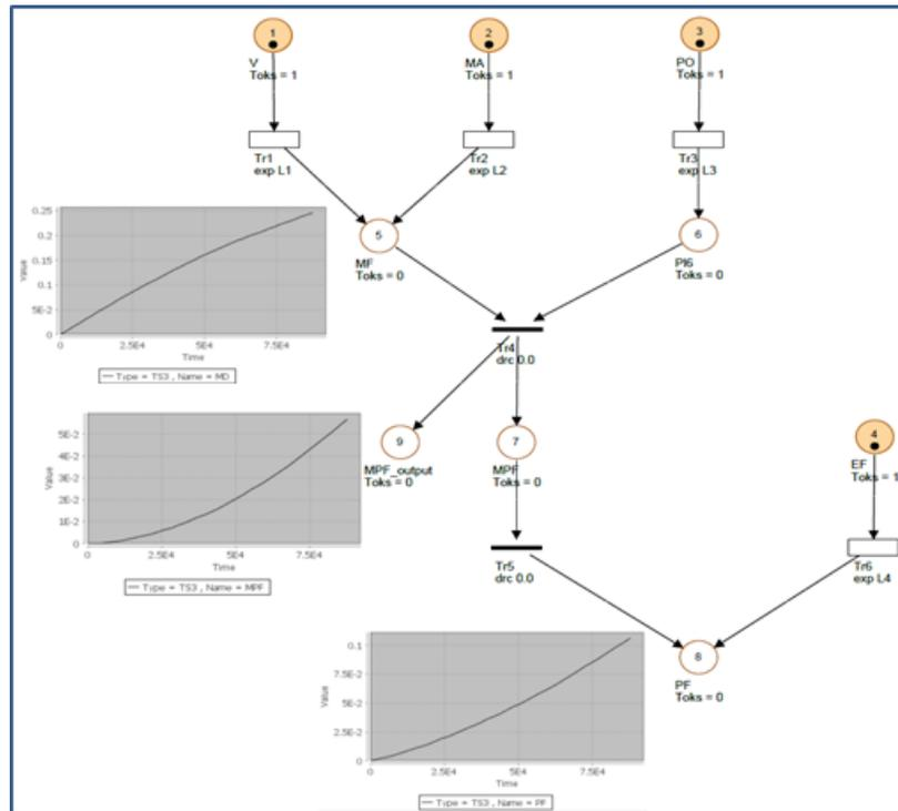
Figure 3. 13 SPN model for the pump failure scenario
