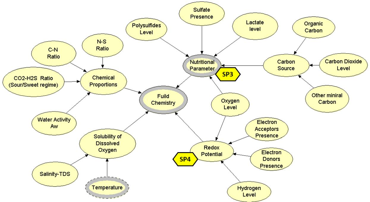
**Figure 2. 3 OOBN sub-network of the fluid chemical factors that influence the MIC potential and their interactions**
