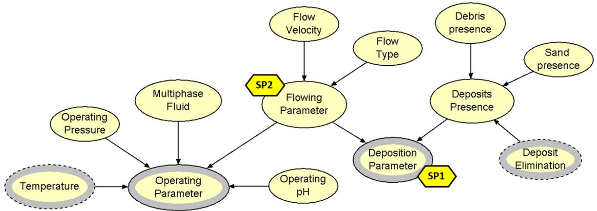
**Figure 2. 2 OOBN sub-network of the operating factors that influence the MIC potential and their interactions**
