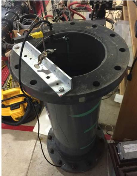
Figure 2.12: Wave Probe Calibration
