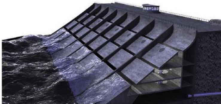
Figure 1.8: Seawave Slot-Cone Generator (Vicinanza et al., 2008)
