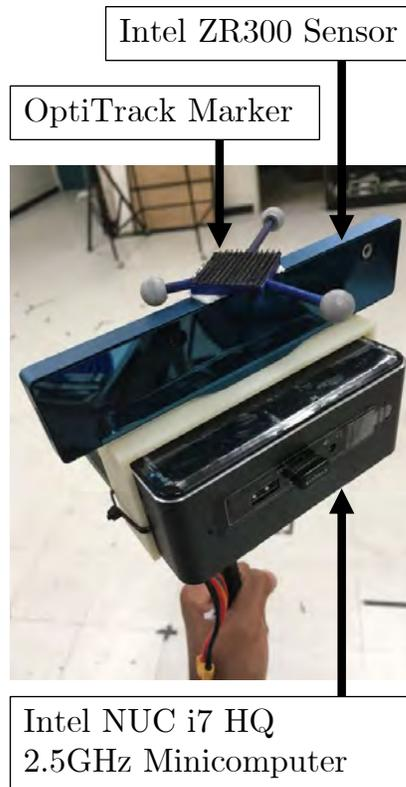
Figure 3.2: Hand-held sensor unit developed
