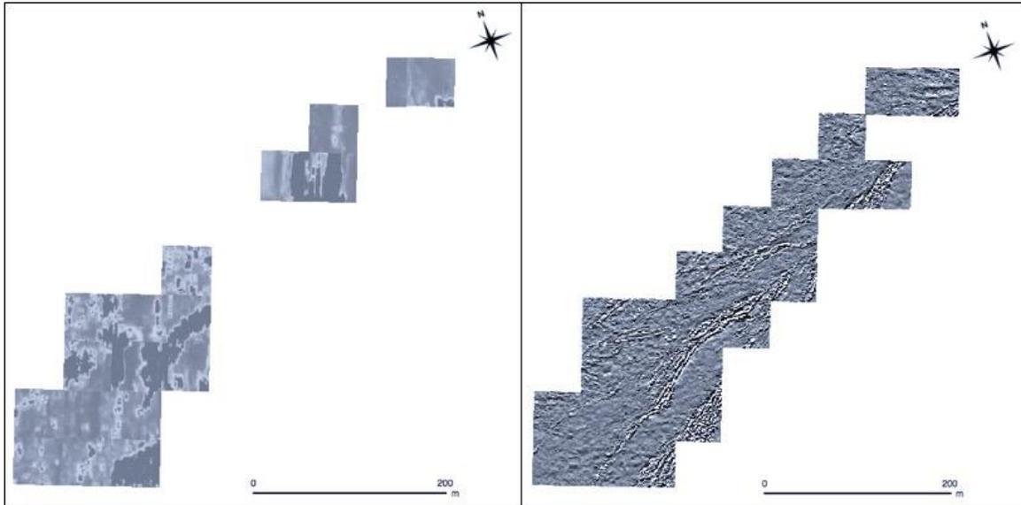
Figure 3.12: Magnetometry (right) and Magnetic Susceptibility (left) data.
