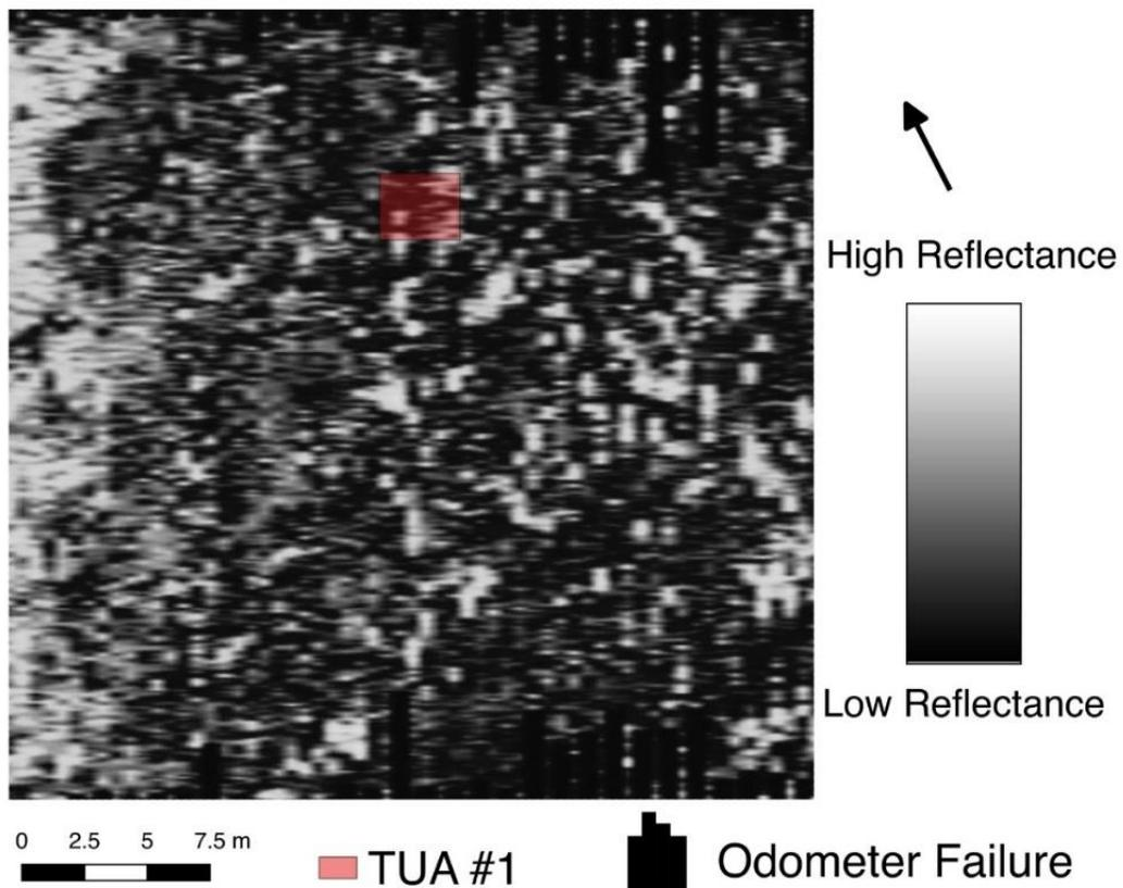
Figure 4.6: GPR plan view over TUA #1 at 10-15 cm below surface.
