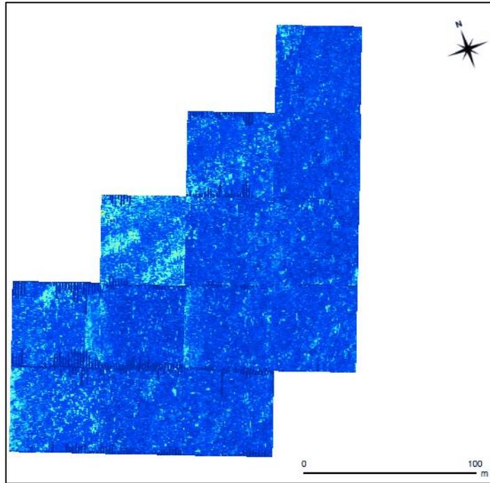
Figure 3.13: GPR plan view at 15 cm below surface. Dark blue lines indicate odometer failure.
