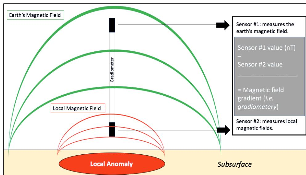
Figure 3.2: How gradiometry identifies buried features.
