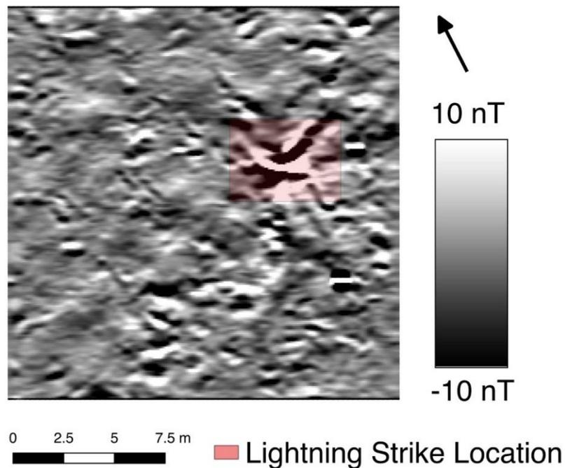
Figure 4.23: Likely lightning strike anomaly in magnetometer data.
