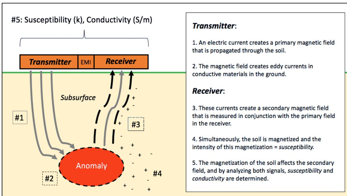
Figure 3.4: How EMI functions to find magnetically susceptible and/or conductive features.
