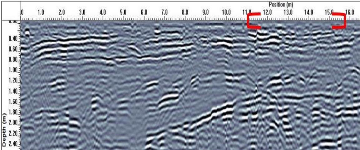
Figure 4.8: GPR profile of TUA #2. Red brackets mark the extent of the feature.
