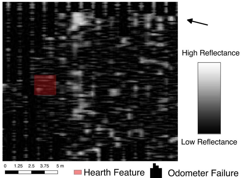
Figure 4.12: Plan view of GPR survey of known combustion feature at 10-15 cm below surface.
