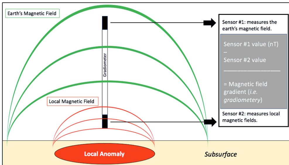
Figure 3.2: How gradiometry identifies buried features.
