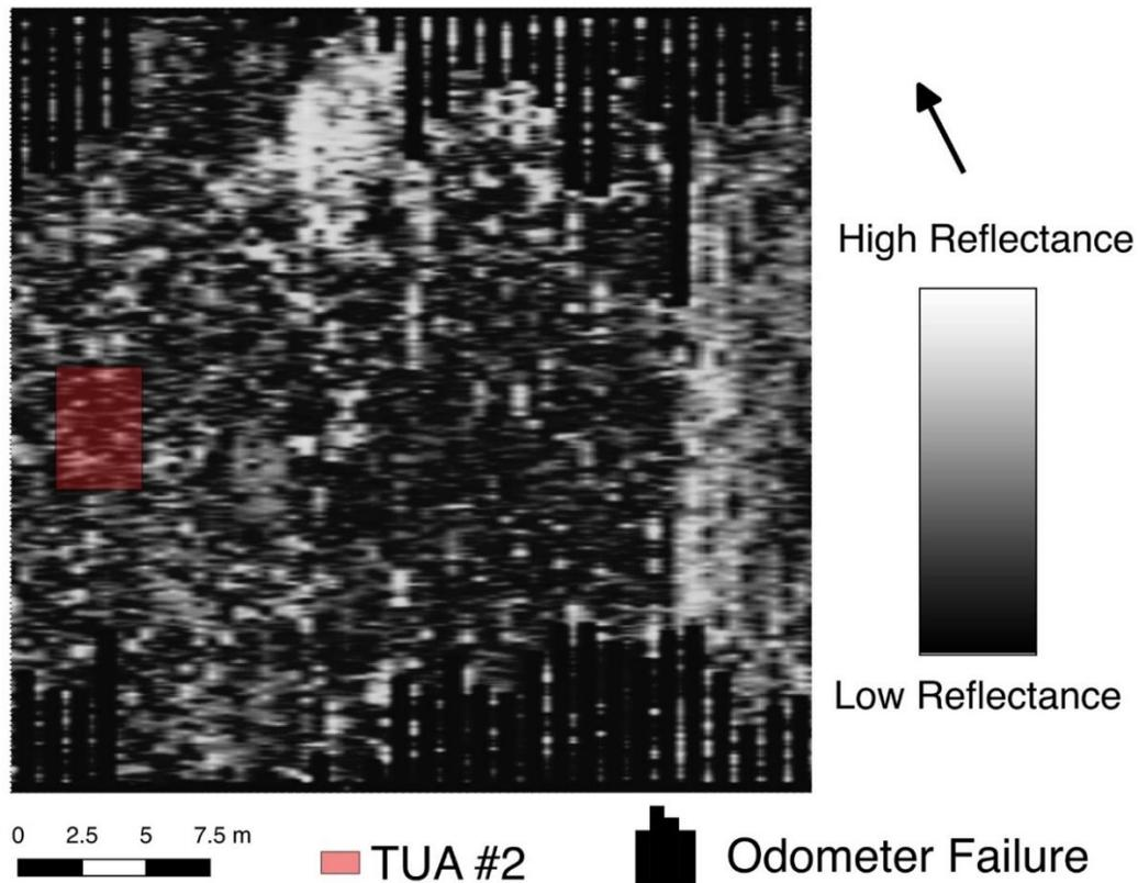
Figure 4.7: GPR plan view over TUA #2 at 10-15 cm below surface.
