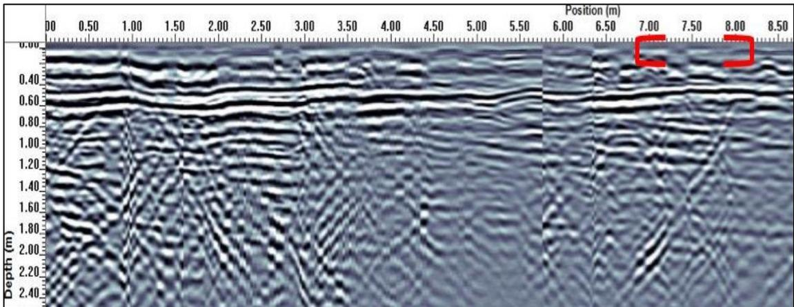
Figure 4.13: Transect profile of the known combustion feature. Feature location marked in red brackets.
