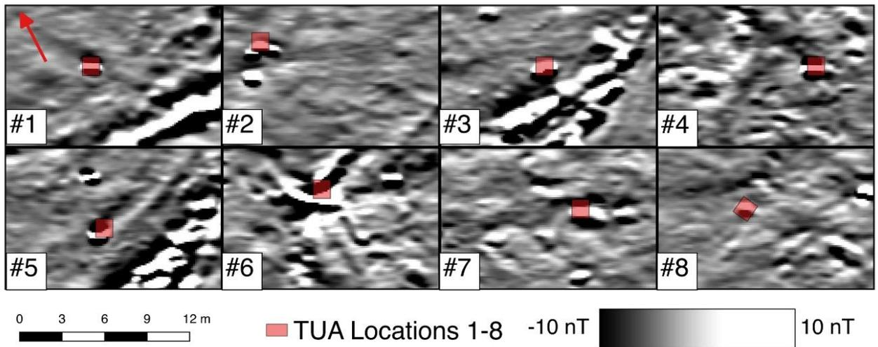
Figure 4.2: TUA magnetometry data showing location of excavated units (TUA # 1-8). TUA #8 was marked without using the arbitrary grid and was therefore oriented roughly due north.
