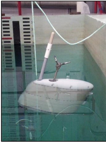
Figure 25 Sensor float stable equilibrium position with cable tension
