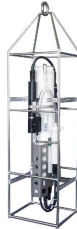
SBE 43 voltage output sensor integrated with SBE 19plus V2 CTD
