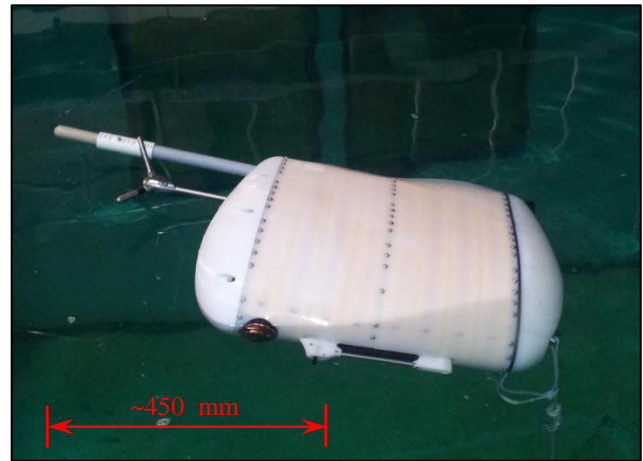
Figure 26 Sensor float stable equilibrium position with no cable tension
