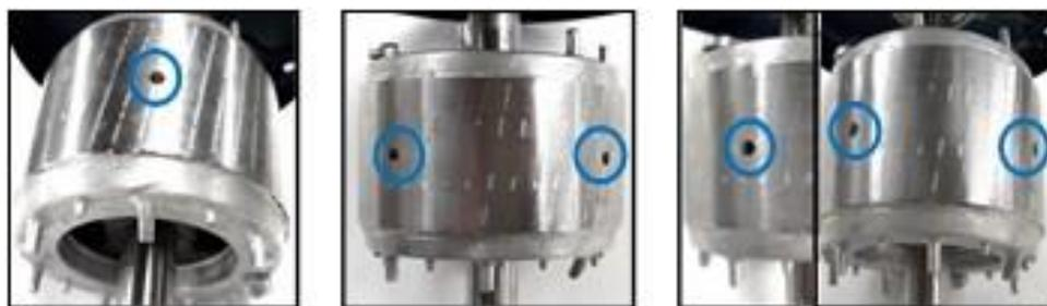
Fig. 4. 3. Motors with BRB faults: (a) 1 BRB, (b) 2 BRB, and (c) 3 BRB.
