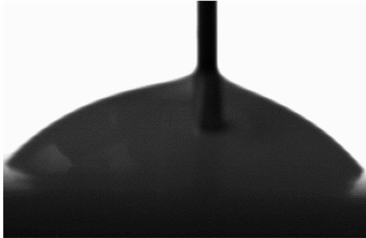
**Fig. 6.4** Sample of dynamic contact angle test of a salt water droplet.
