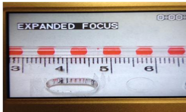
Fig. 6. 3 - Water / 1 cSt silicone oil slug flow ( \alpha_{L_c} = \alpha_{L_d} = 0.5 ) in mini-scale tubing.
