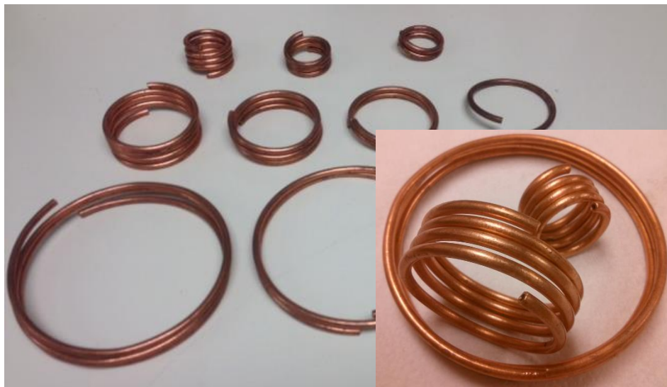
Fig. A. 6 - Some of the examined shapes for different lengths and radii of test heat sections.
