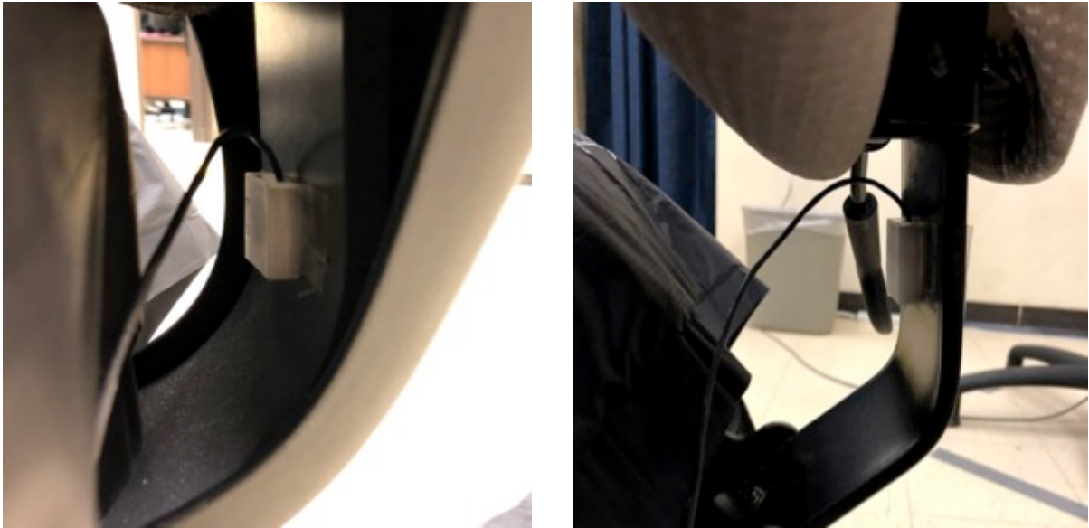
Figure 9: Location of the accelerometer on the rigid arm of the seatpan for both the dynamic chair and the control chair respectively.
