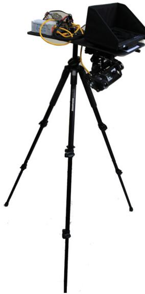
Figure A.3: Tripod with gimbal mounted and data monitoring system for remote data collection.
