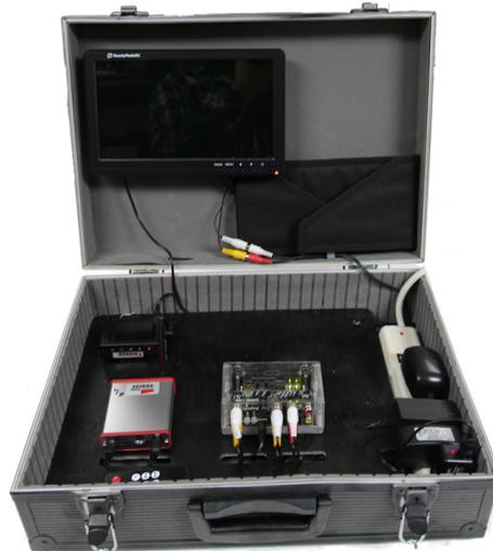
Figure A.2: Image of the ground control station used to monitor, record, and control the gimbal.
