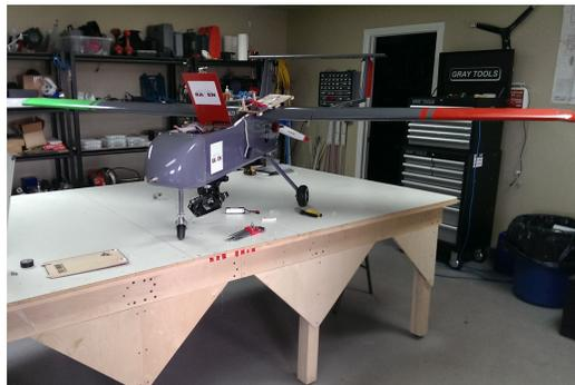
Figure A.4: Image of the customized gimbal containing the FLIR A65 LWIR camera and GoPro Hero2 EO imager mounted on the Mugins 3M H-Tail TBM.
