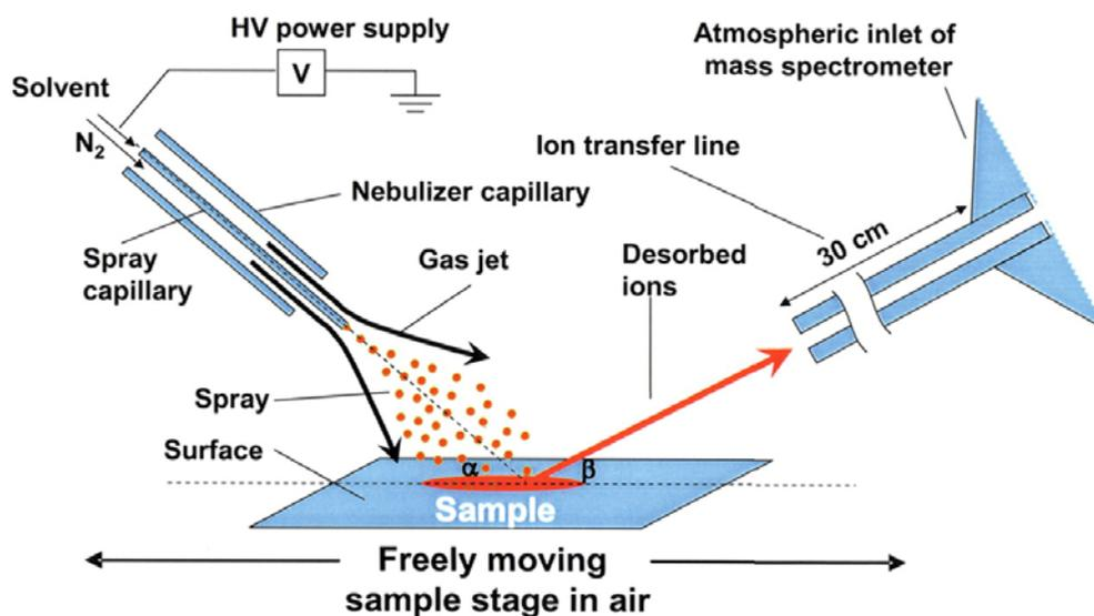
Figure 1.4. Diagram of the DESI system<sup>52</sup>
