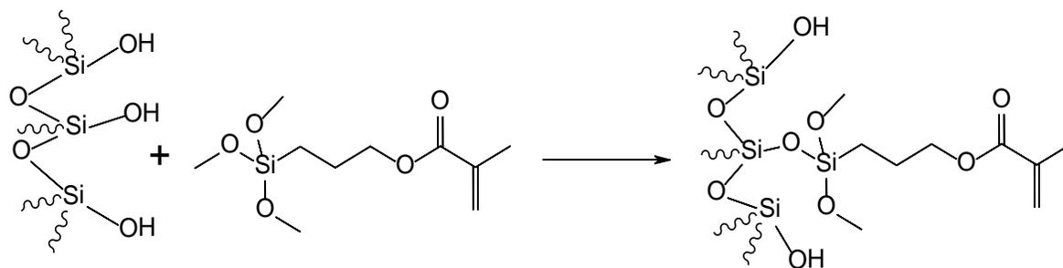
**Figure 2.1. Derivatization of glass surface with 3-(trimethoxysilyl) propylmethacrylate.**
