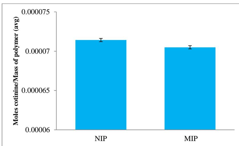
**Figure 3.10. Comparison of MIP and NIP after uptake of cotinine when myosmine is used as a pseudo-template. (n=4)**
