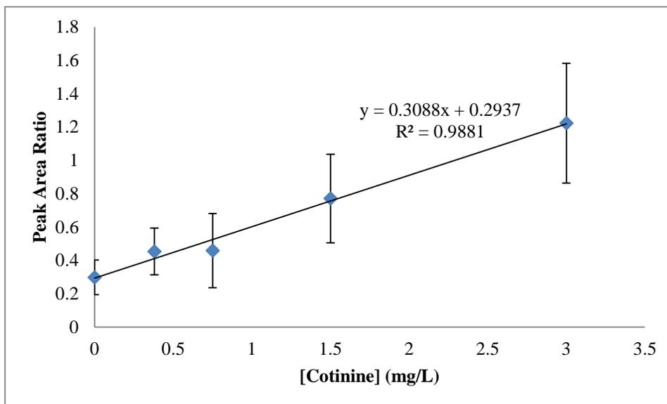
**Figure 4.4.** Calibration curve for the analysis of cotinine in human urine using MIPs (n=2).
