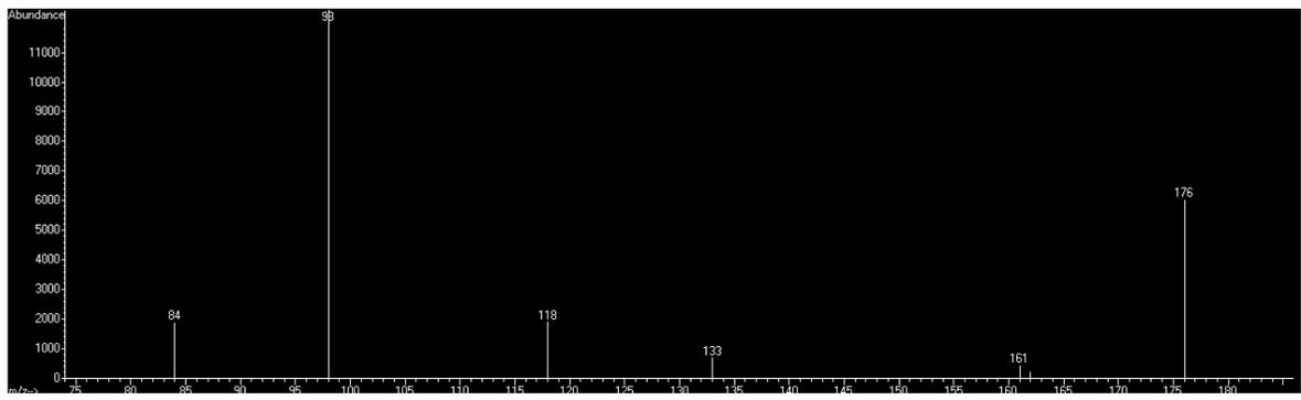
**Figure 2.3. GC-MS spectrum of a Cotinine MIP extract.**
