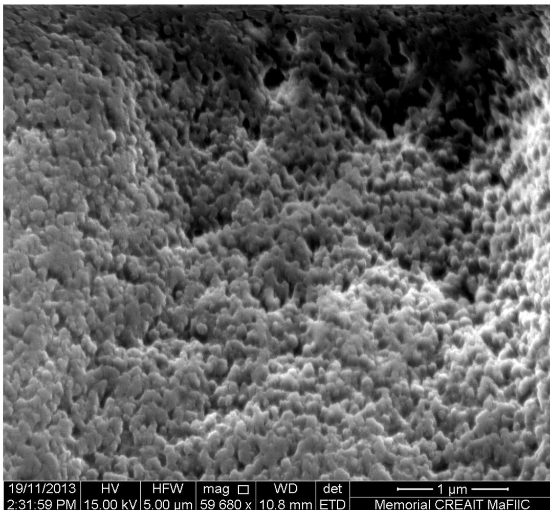
**Figure 4.2. SEM image of cotinine MIP showing pores**
