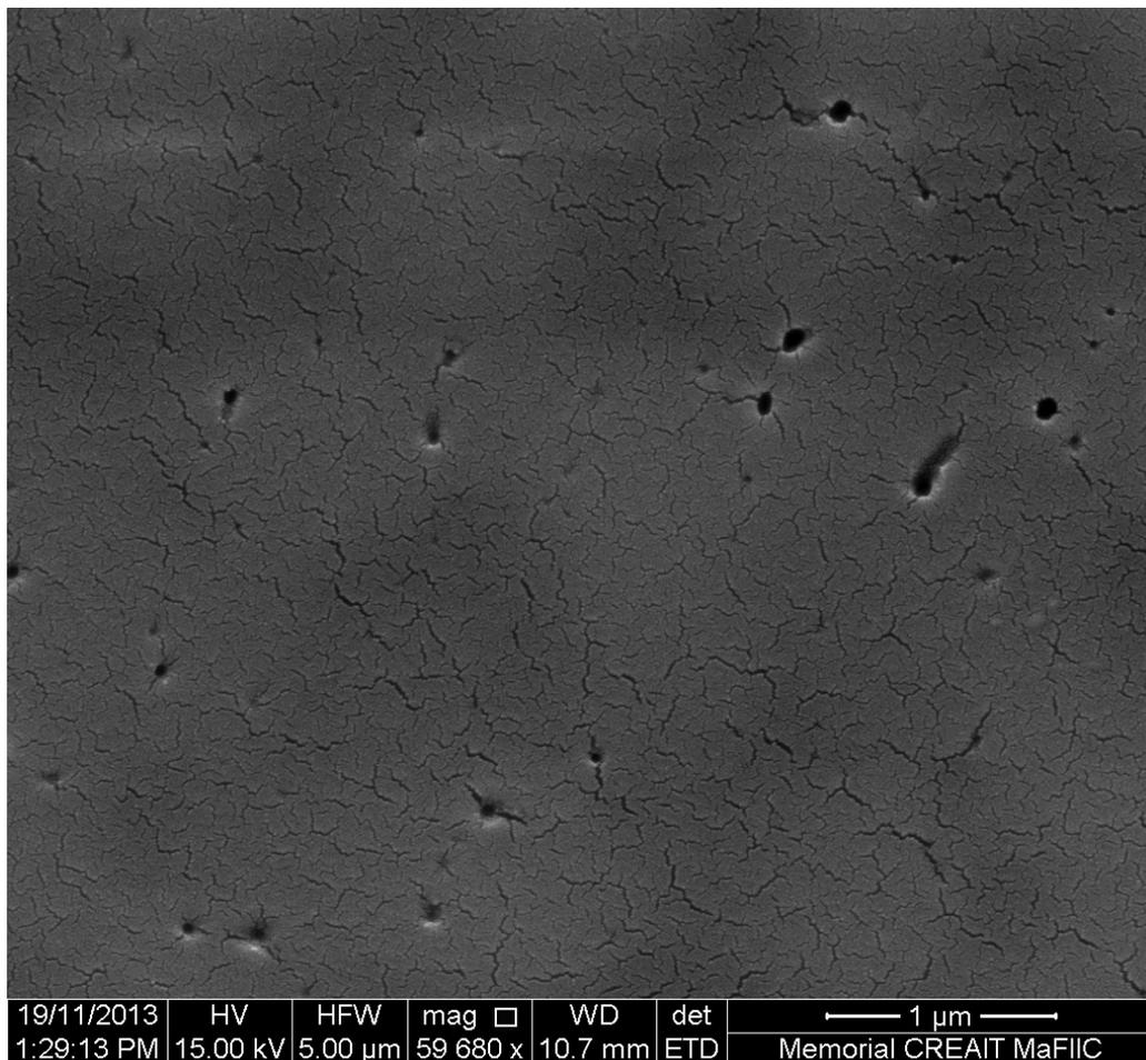
**Figure 4.3. SEM image of NIP showing lack of pores.**
