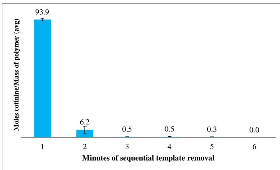
**Figure 3.6. Template removal study, change in cotinine over 100 min intervals with 9:1 MeOH:AcOH as extraction solvent (n=2)**
