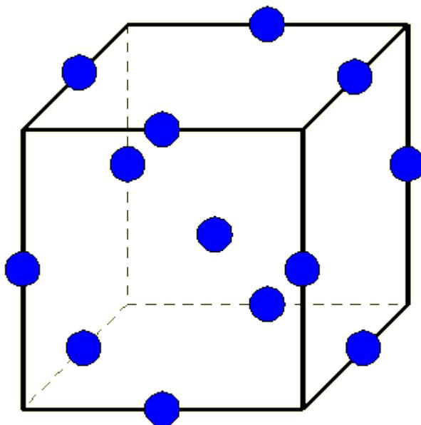
**Figure 3.3. 3-D cube plot of Box-Behnken design for 3 factors (blue balls are independent variables)**
