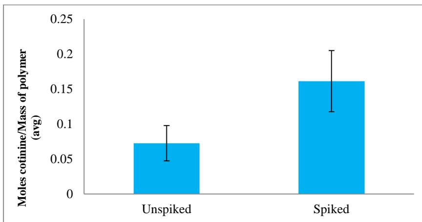
**Figure 3.8. Assessment of template bleeding in cotinine MIPs by comparison of uptake from spiked and unspiked solutions (n=4).**
