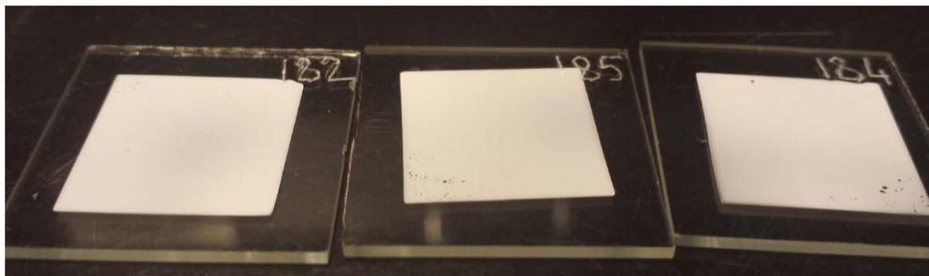
**Figure 2.2.** Image of MIPs in thin-film format.
