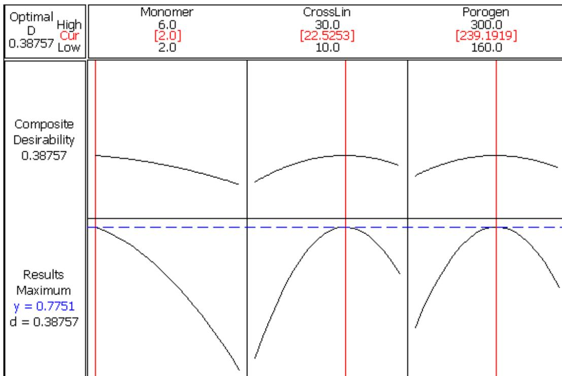
**Figure 3.4. Optimization plot from Minitab to determine the optimal ratios in the pre-polymerization solution.**
