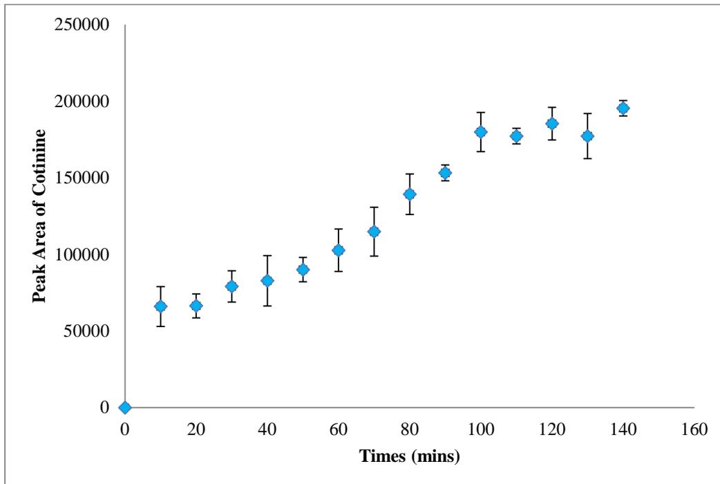
**Figure 3.5. Template removal equilibrium study at 10 min intervals, analysis carried out by GC-MS in SIM mode (n=2).**
