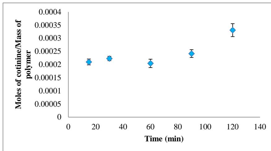
**Figure 3.12. Study of the optimal length of uptake time for cotinine MIPs**
