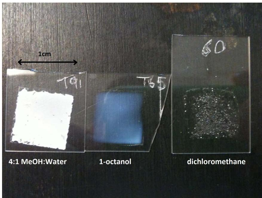
**Figure 3.2.** Thin-film MIP surface appearance using various solvents
