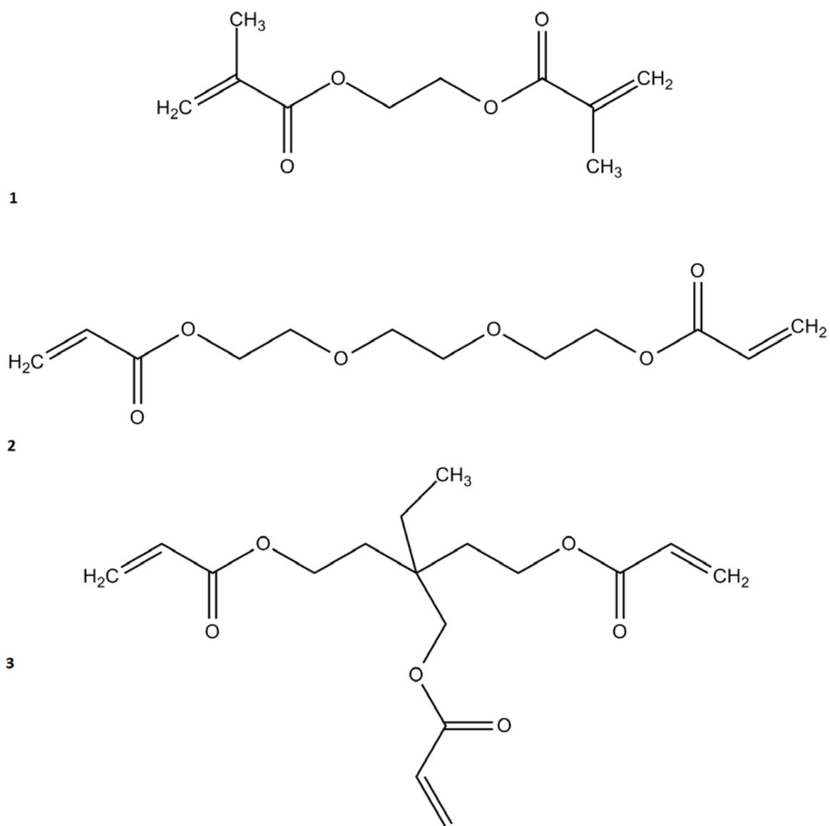
**Figure 4.6. Graphical representation of cross-linkers tested(1:EGDMA, 2:TEGDMA, 3:TRIM).**
