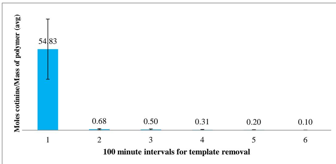
**Figure 3.7. Sonication template removal at 100 min intervals**
