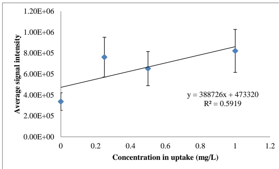
**Figure 4.5.** Analysis of cotinine in human urine by way of DESI-MS (n=2)
