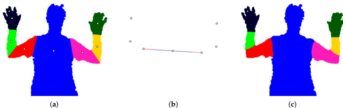
**Figure 6.** Segmenting with line seed pixels. (a) Ground truth image and part positions. (b) A line of seed pixels is drawn from the torso to each upper arm position. The first 2/3 of the line is labelled torso, and the remaining pixels are labelled L/R upper arm. Each other part  $i$  receives a single seed pixel. (c) Final segmentation.
