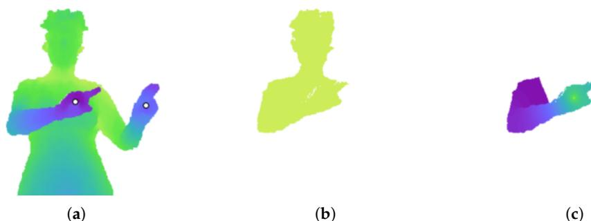
**Figure 1.** Effect of adding a dummy node. (a) Depth image. The white dots indicate the annotated hand pixels. (b) Probability values for the right hand, using the two hand pixels as seeds for the RW algorithm. The values are close to either zero or one. (c) Probability values after adding a dummy node to the graph. There is now a greater variance in the values.
