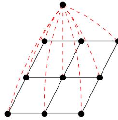
**Figure 2.** Diagram of a dummy node being added to the grid graph. Each node in the grid represents a pixel in the depth image. The dummy node is connected to each grid node by a single edge (dashed line).
