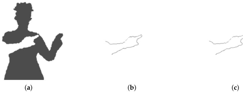
**Figure 4.** Relevant binary images. (a)  $F_{other}$  is the set of foreground pixels outside the arm segment (in this case, the right arm). (b)  $B_{inner}$  is the set of pixels inside the arm and neighbouring  $F_{other}$ . (c)  $B_{outer}$  is the set of pixels inside  $F_{other}$  and neighbouring the arm.
