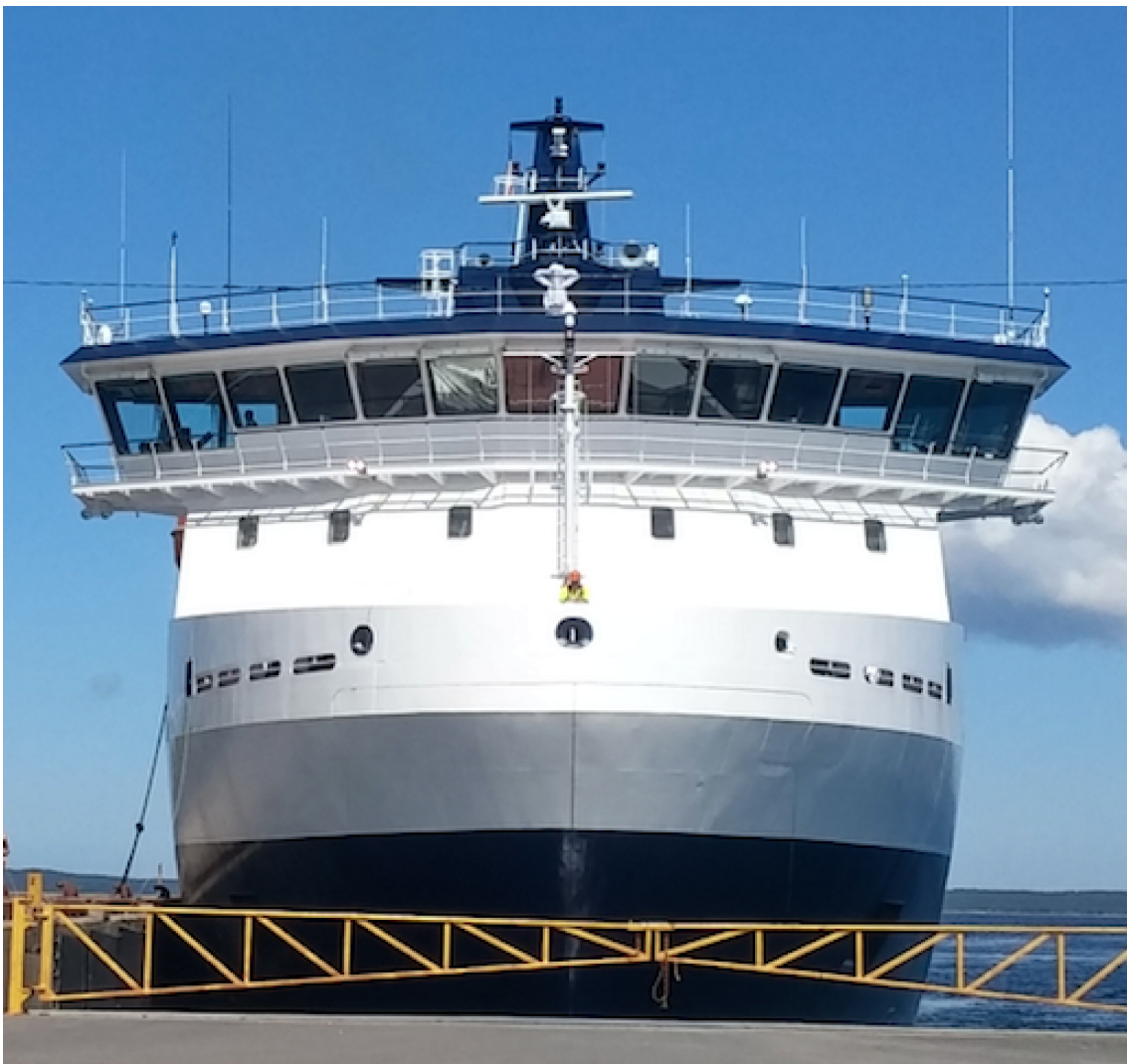
Figure 9: Slightly curved bow of the MV Veteran designed for ice-breaking (Source: Author's Photo)
