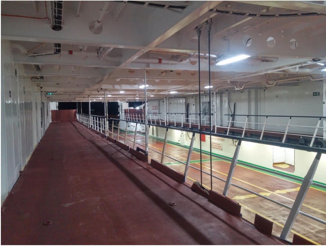
Figure 6: Hoistable hydraulic ramps on the MV Veteran's vehicle deck which were the subject of warranty claim 80 (Source: Author's Photo)
