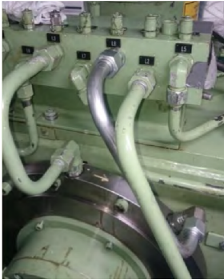
Figure 5: Additional oil lubrication channel (silver coloured pipe from centre to bottom right of image) added to bearings two and three taken from the Damen Shipyards Report presented to DTW on June 10, 2016 (DTW, 2016c: 664)
