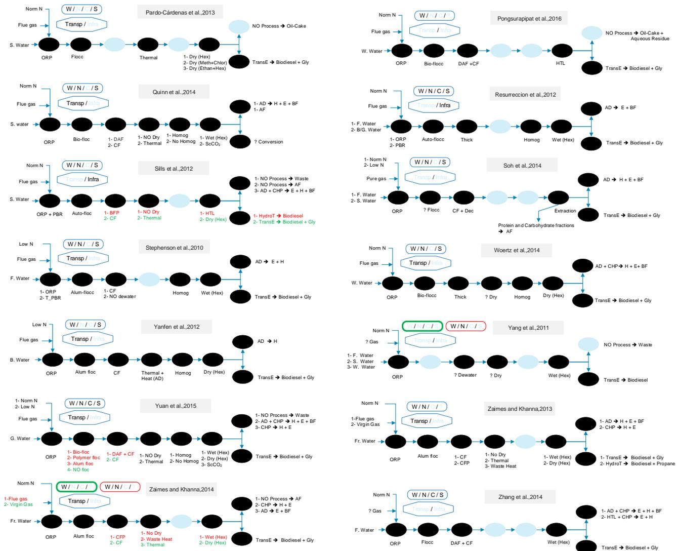
**Figure 2-9: A summary of process pathways used for the conversion of algae to biodiesel in literature**
