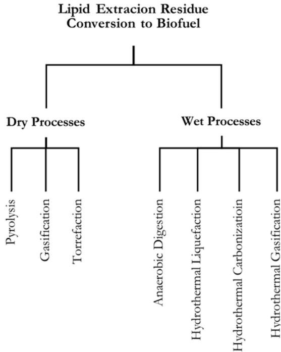
**Figure 2-7: Possible processes to convert algae biomass (from lipid extraction residue) to biofuel**
