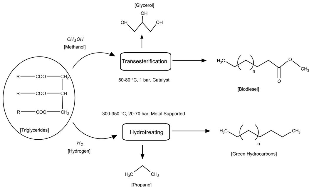
**Figure 2-6: Comparison of reaction pathways and operating conditions for transesterification and hydrotreating (Adopted from Serrano-Ruiz et al., 2016)**
