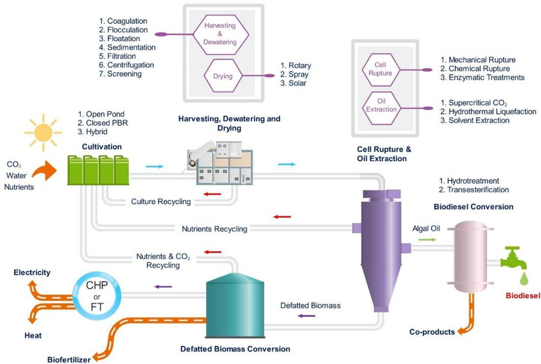
**Figure 2-3: Process flowchart for production of microalgal biodiesel**
