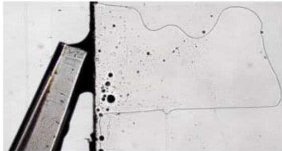
Figure 2-2 Schematic view of the connection of the pipette to EWOD system (taken from [18]).
