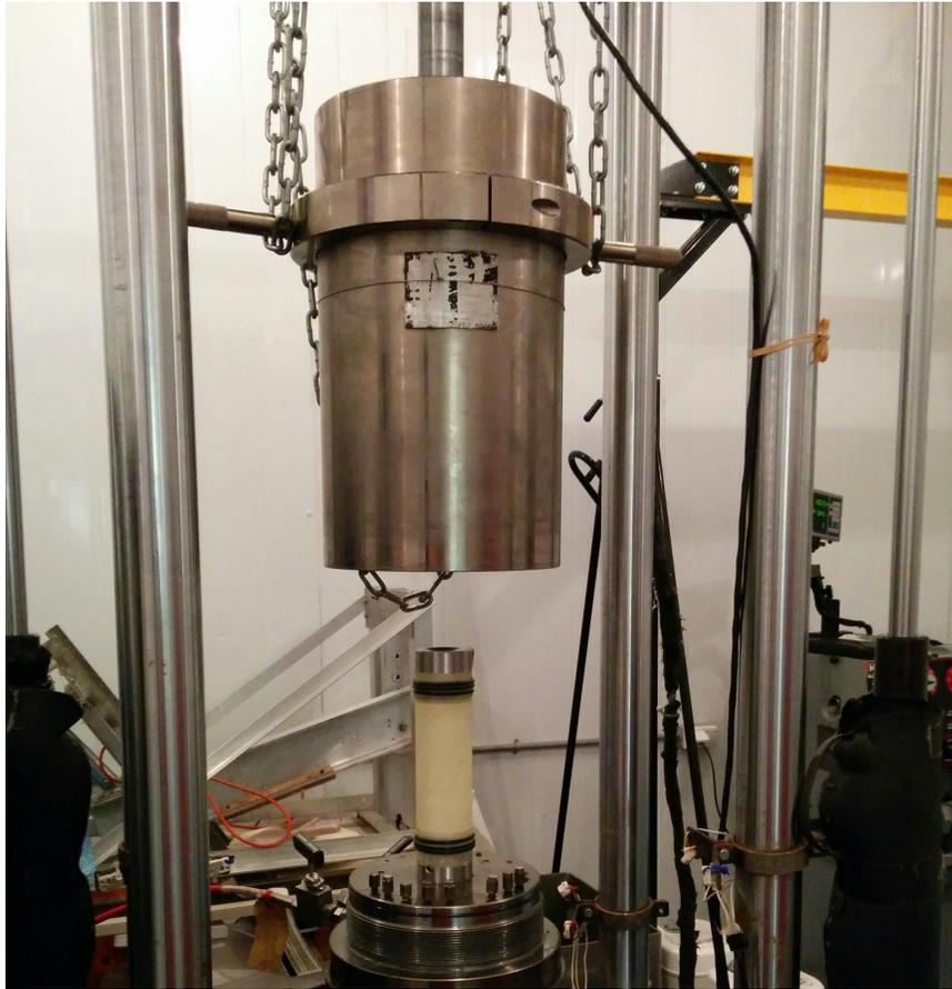
Figure 3.1: Triaxial equipment prior to testing.
