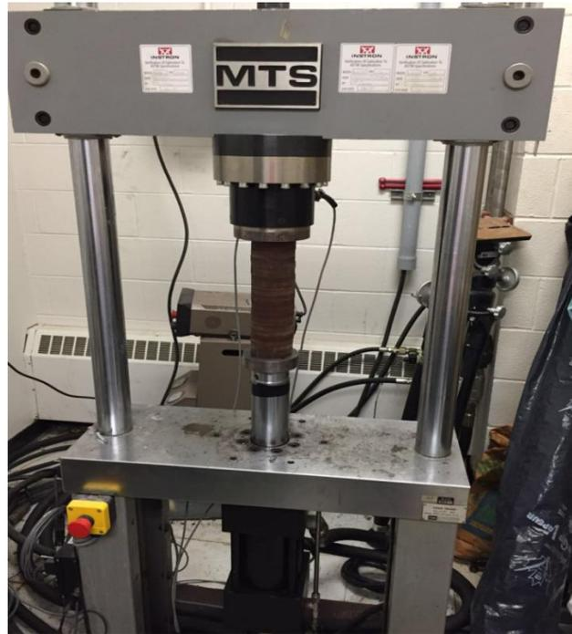
**Figure 30 Testing equipment set up with two parts of isolator and load is control by a hydraulic actuator**
