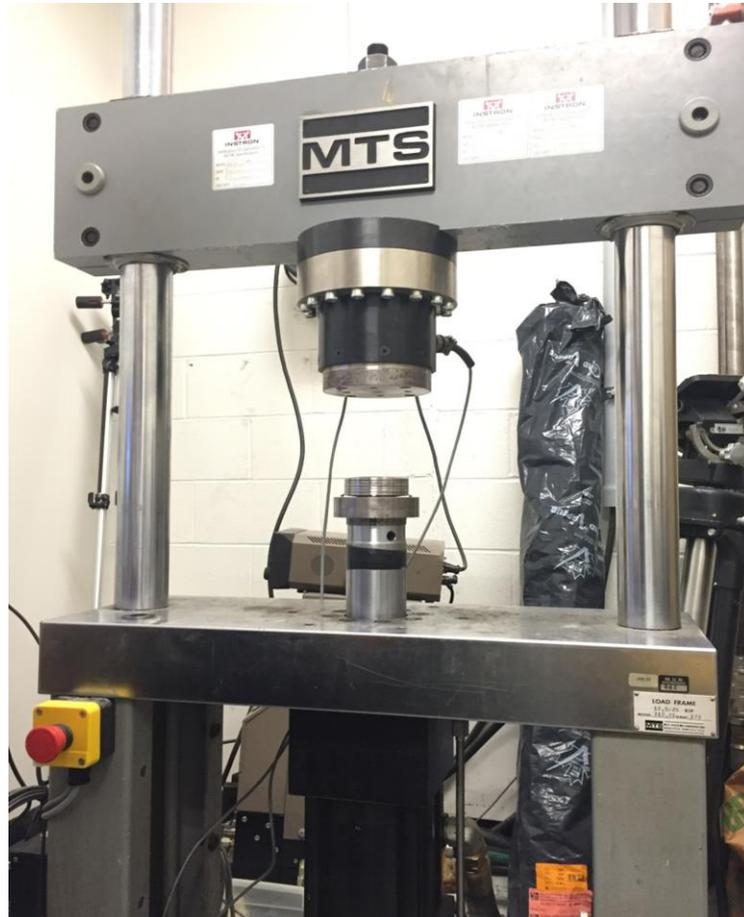
**Figure 32 Rings of high-carbon steel Belleville dis springs are under tests**
