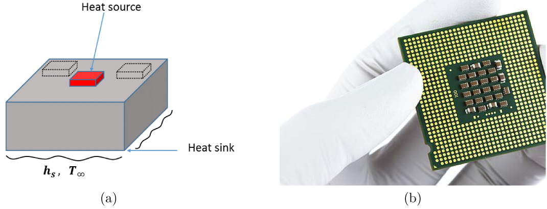
Figure 1.1: (a) Schematic layout of a 3D flux channel. (b) A sample of a microelectronic device [4].
