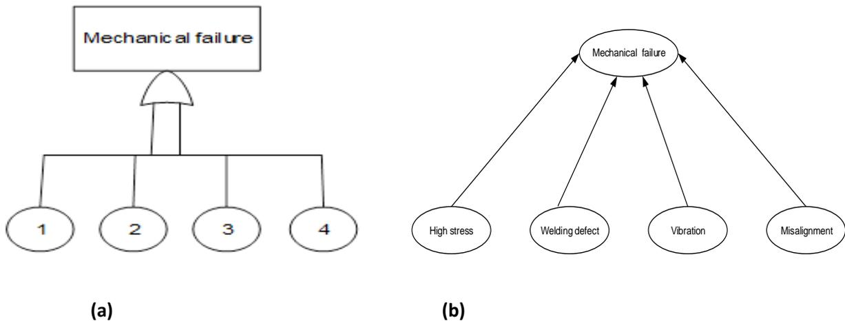
**Figure 4. 3. Fault tree and Bayesian network for causes of mechanical failure.**
