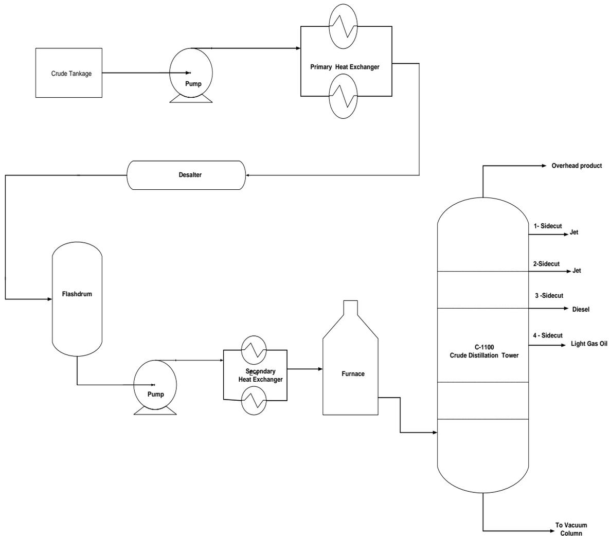
**Figure 8.2. The process flow diagram of Richmond refinery crude unit and its associated up stream equipment( Adedigba et al. 2016; CSB 2015).**
