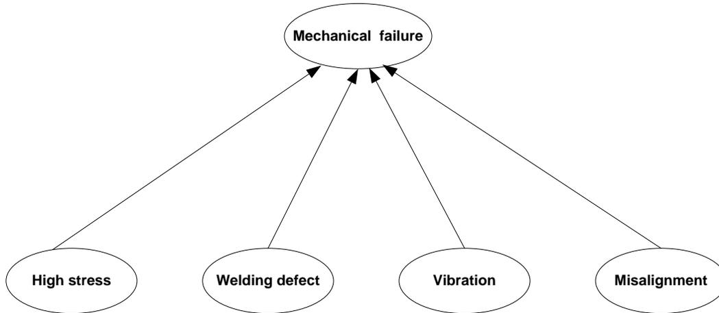
**Figure 5.3. Bayesian network for causes of mechanical failure.**
