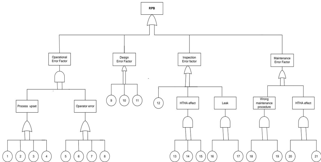
**Figure 5.1. Fault tree analysis of Release prevention barrier.**
