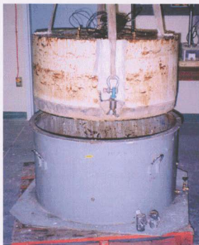
Figure 4.13. Extrusion of clay from strongbox
