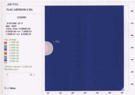
Figure A5.44. Change in vertical effective stress (2FRAC2a: 0.28 ml/s)
