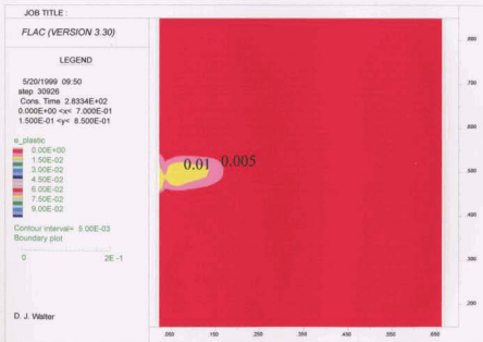
Figure A5.102. Plastic strain contours at end of injection (2FRAC3b: 3.0 ml/s)
