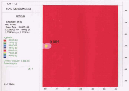
Figure A5.72. Plastic strain contours at end of injection (2FRAC2d: 0.25 ml/s)
