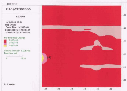
Figure A5.323. Change in horizontal effective stress at t = 1420 s (CCFS03I)
