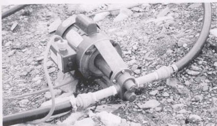
Figure 3.5. Injection pump for field tests
