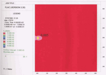
Figure A5.62. Plastic strain contours at end of injection (2FRAC2c: 1.00 ml/s)
