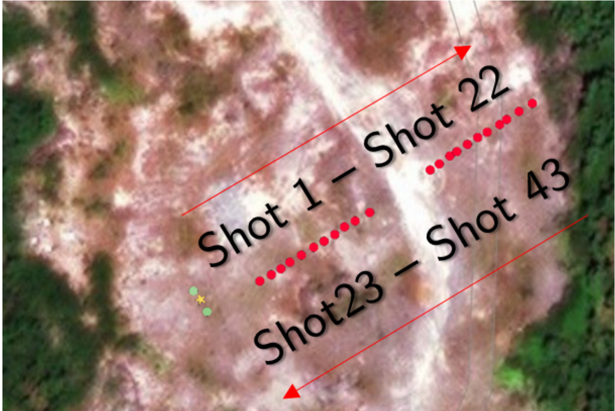
Fig. 5.4: Satellite photo of the Collier Point interferometry experiment site demonstrating location of shot points, borehole and shooting directions.
