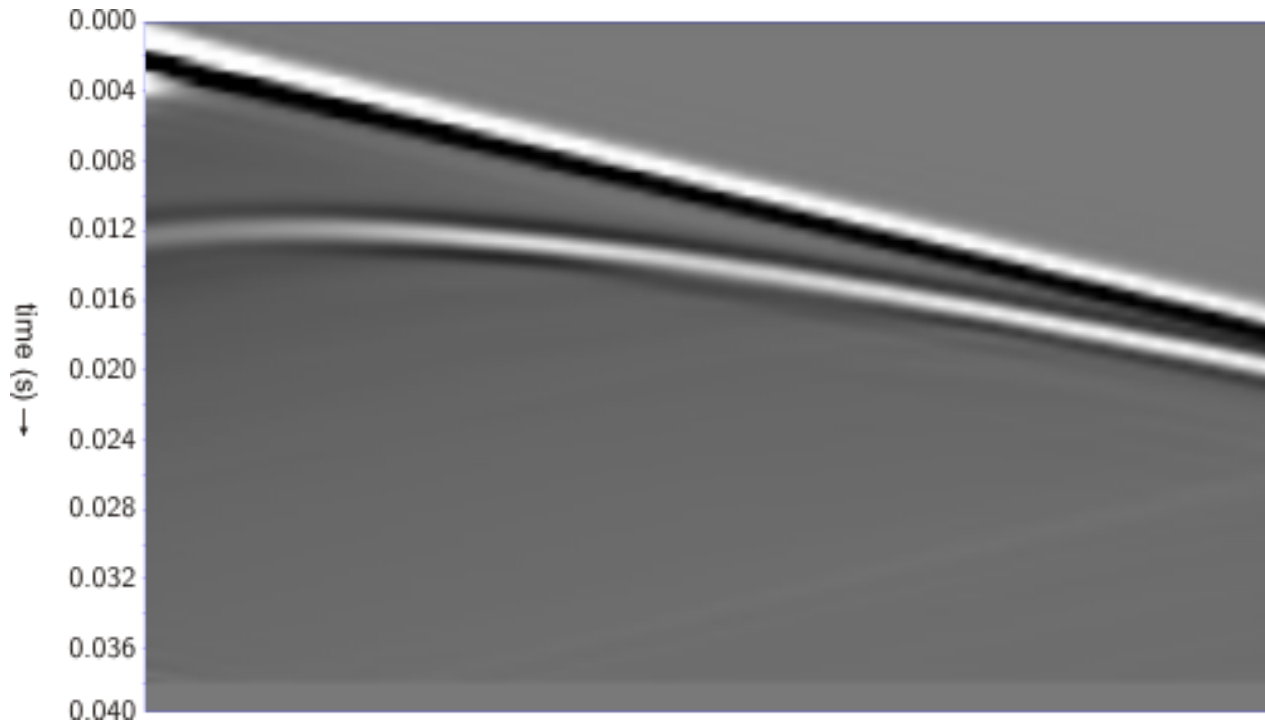
(a) Shot 1 - The seismogram represents a VSP from the first surface source location
