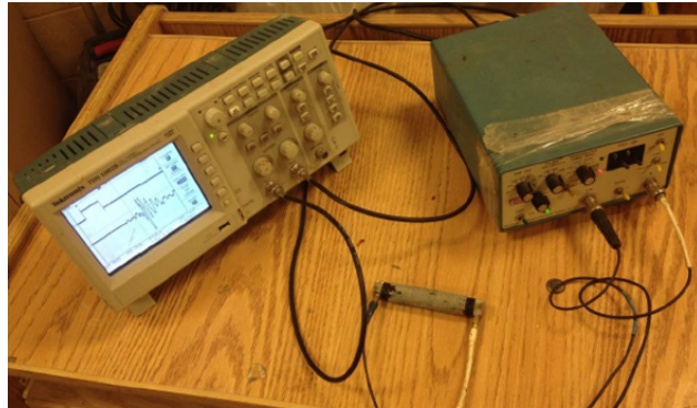
(b) Photograph demonstrating acoustic testing on arkosic bedrock core
