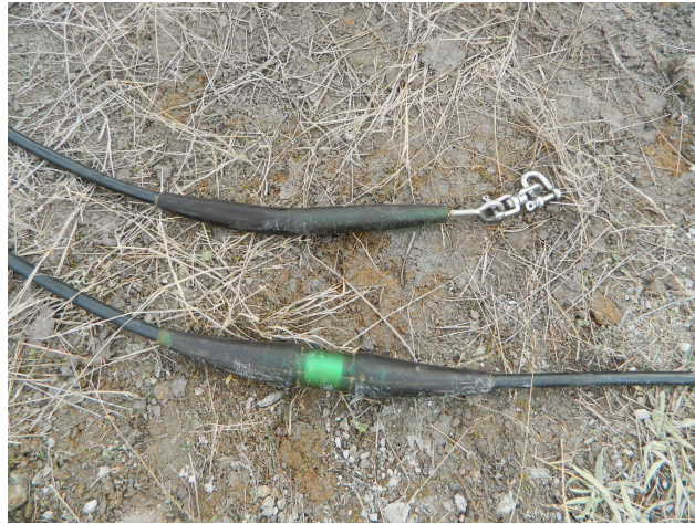
Fig. 5.2: A receiver on the bottom of hydrophone cable used in the experiment
