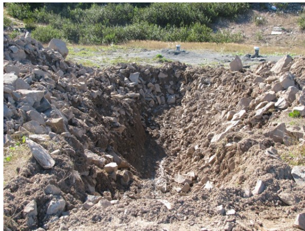
Fig. 5.3: Photo of trench dug for placing shot points during the Collier Point Interferometry Experiment
