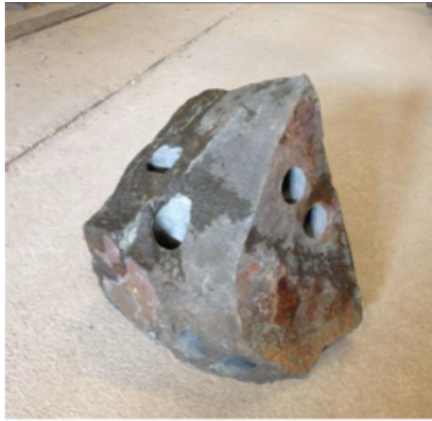
(a) Arkosic bedrock sample used for drilling cores
