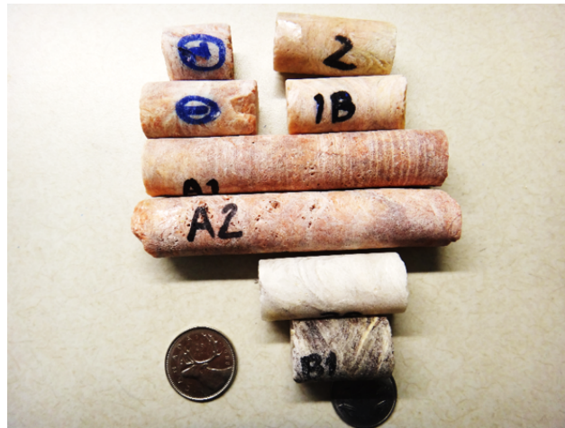
(b) Barite cores used for acoustic velocity testing - note wide variation in colour
