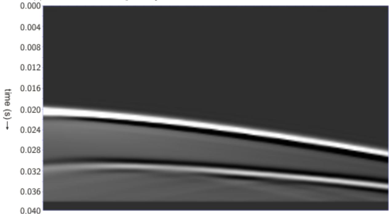
(b) Shot 51 - The seismogram represents a VSP from the last surface source location
