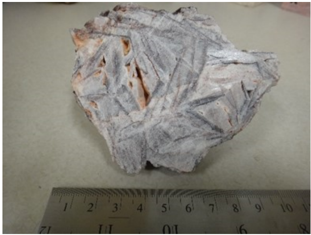
(a) Barite hand samples - note large porosity
