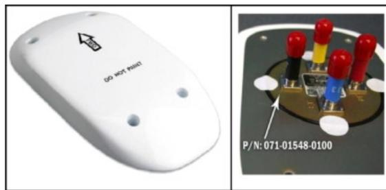
Figure 2.2: TCAS direction antenna [5].
