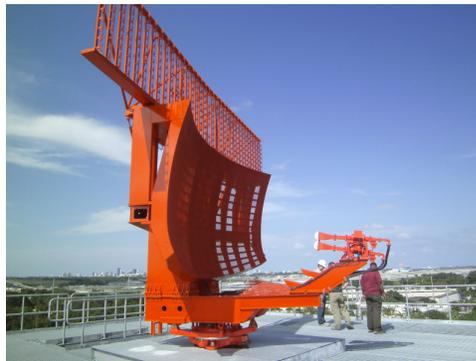
Figure 2.1: Antennas of a typical ground surveillance radar system for ATC [4].
