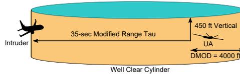
Figure 4.4: WC cylinder diagram.
