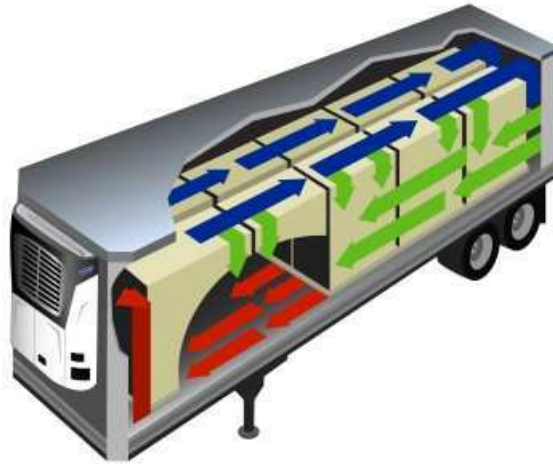
Figure 2.4: Top-down air delivery in a semi-trailer
