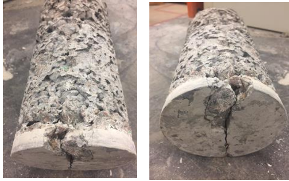
Figure 4.3: Splitting tensile strength test failures.
