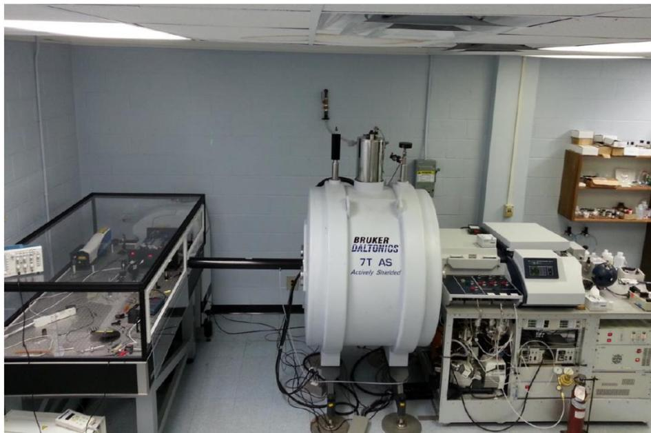
**Figure 2.1.** Bruker Apex-Qe7.0 T Fourier transform ion cyclotron mass spectrometer FT-ICR MS coupled to OPO laser located at Memorial University.
