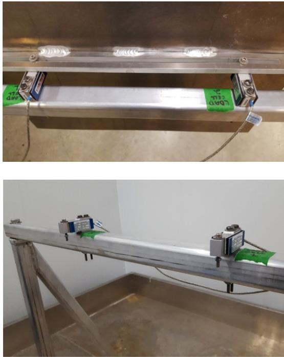
Fig. 6.3: Installation of the load cells for measuring ice accretion rates on a vertical plate
