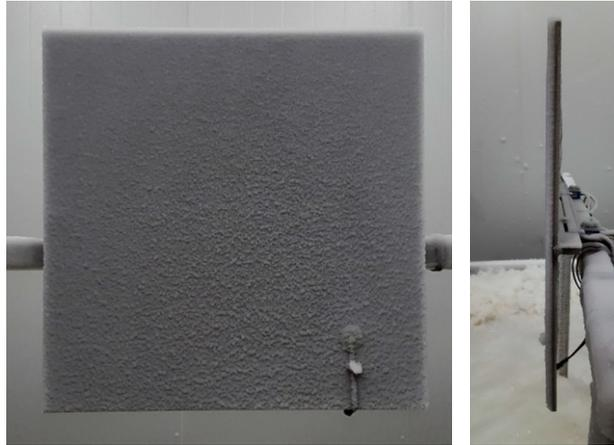
Fig. 7.2: Two views of ice accretion on the vertical plate at  $V_{ave,3} \approx 2.65$  m/s,  $T_C = -10^\circ\text{C}$ ,
