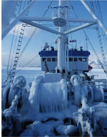
Fig. 1.1: View of ice accumulation on deck of a marine vessel (Cammaert, 2013)
