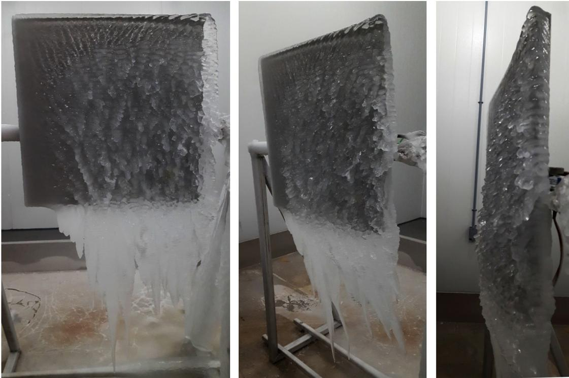
Fig. 7.1: Views of ice formation on the vertical plate at  $V_{ave,l} \approx 7.85$  m/s,  $T_C = -10^\circ\text{C}$ ,  $S_w = 0\%$ ,  $RH_{ave} = 72.2\%$ , and the distance of 1.65 m between the fan and the plate
