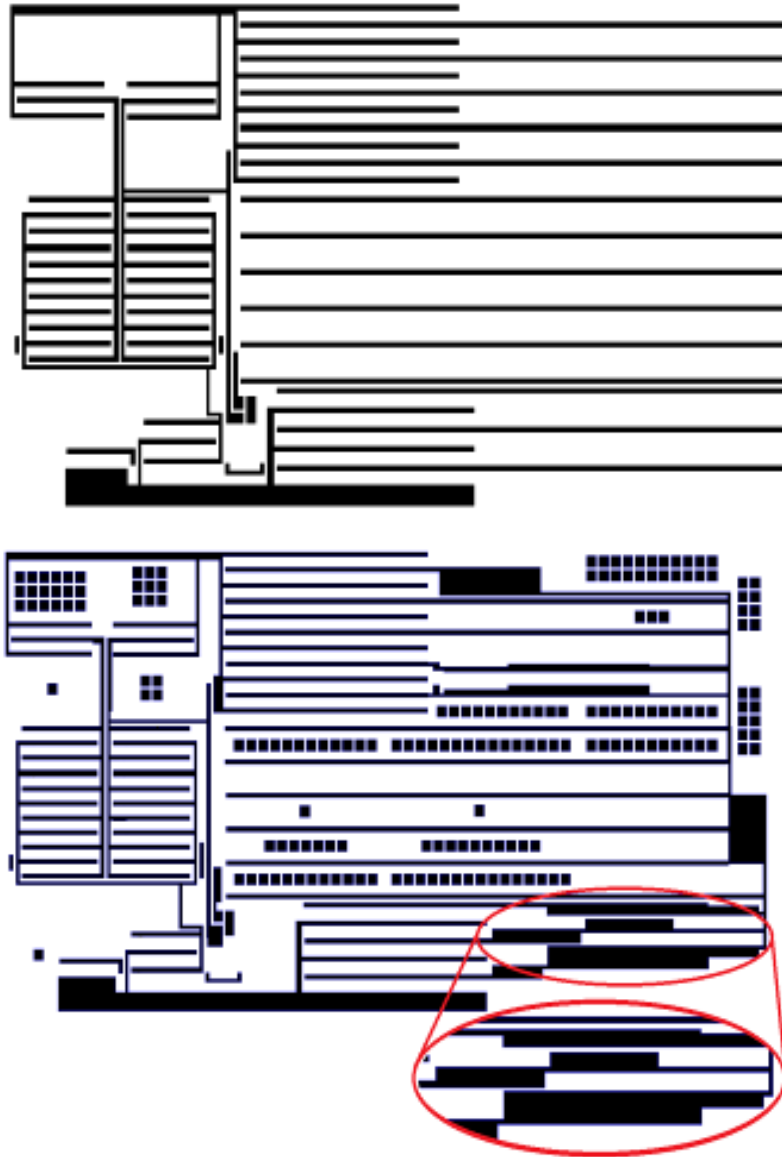
Figure 37 – Two-stage Opamp layouts before (top) and after (bottom) the AS+IW+DF operations in CMOS 180 nm technology. The splitting and widening operation is also shown in the red ellipse.
