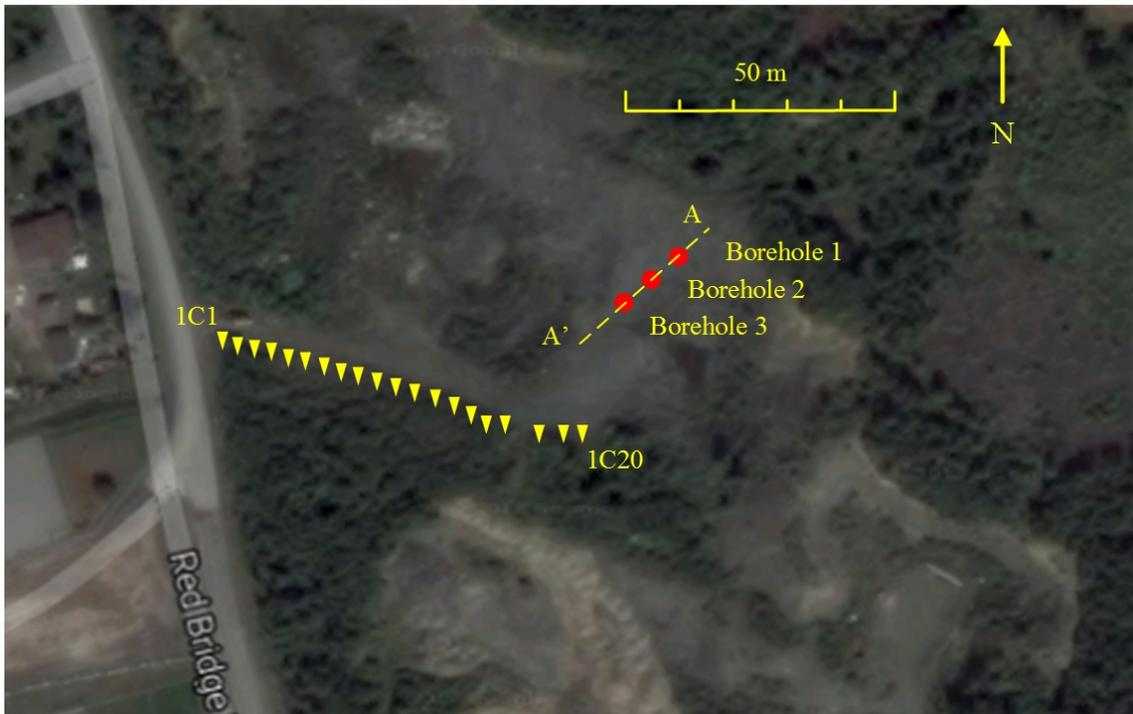
Figure 4.1: Spread of 1C geophones array (20) with three seismic source boreholes in Greenslades Construction Quarry of east Newfoundland (based on Google map)
