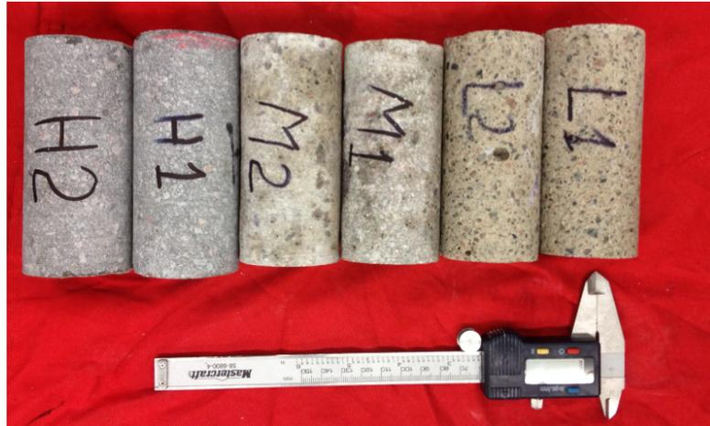
Figure 2.2: Tested concrete cores (low, medium and high strength)
