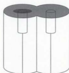
C: Gold film coating via vapour deposition
