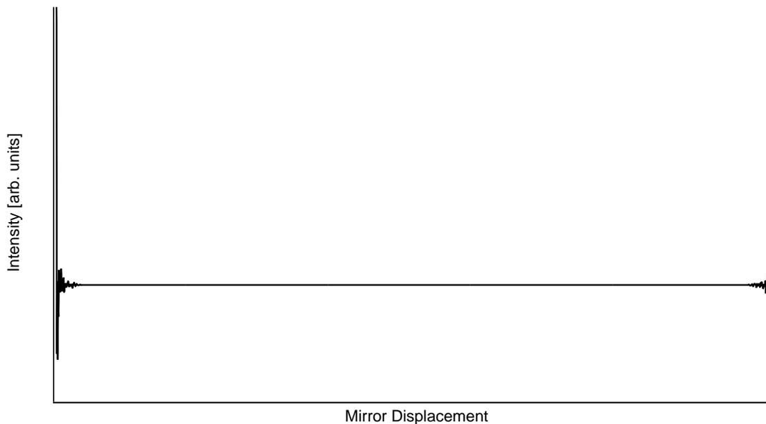
Figure 2.14: The apodized, zero-filled centerburst data is rotated such that the data prior to the centerburst are placed at the end.
