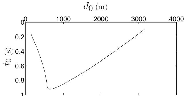
FIGURE 8: Constant velocity medium DMO impulse response, scattering angle 0.7 radians,  $c_0 = 1.7$  km/s,  $t = 2$  s.
