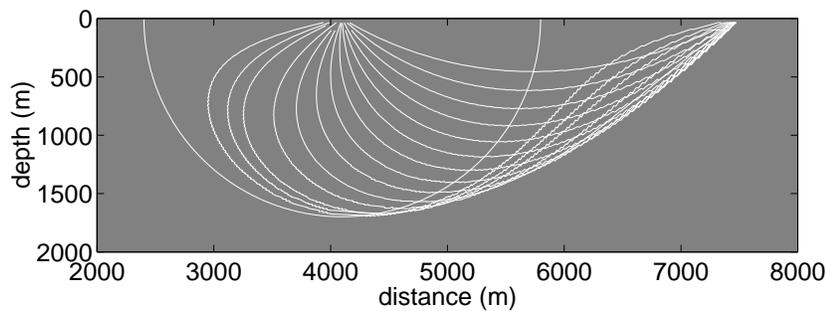
FIGURE 7: Constant velocity medium ( $c_0 = 1.7$  km/s) the lines are the locations of the scattering points. Each line represents a different scattering angle, the circular line is  $e = 0$ , and the other lines are at increments of 0.1 radians from 0.1 radians (leftmost line) to 2.6 radians (shallowest line). All other parameters are the same as Figure 6.
