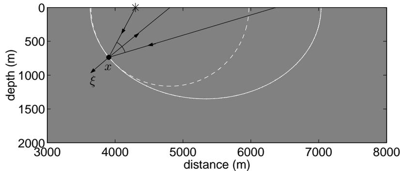
FIGURE 5: Constant velocity medium ( $c_0 = 1.7$  km/s) the solid curve is the finite offset isochron, the dashed curve the zero-offset isochron, the black lines are the rays and the dot shows the location of the scattering point, which is the same as that marked by a dot in Figure 6.
