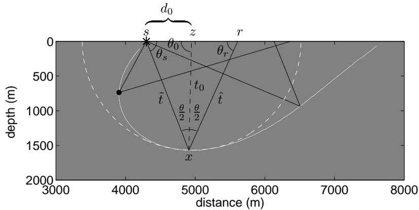
FIGURE 6: Notation for the derivation of the constant medium impulse response (cf. Appendix A). Black lines are rays, the dashed white curve is the zero-offset isochron, the solid white curve is the  $e$  'isochron' and the black dot is the location of the scattering point for the rays shown in Figure 5.
