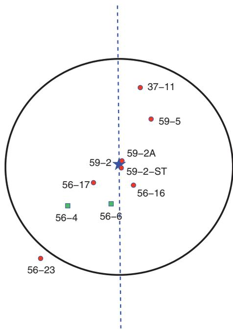
Figure 1. Schematic illustration of walkaway VSP surveys and CO<sub>2</sub> injection and monitoring wells at the SACROC EOR field. The red dots denote the wells with logging records. The green squares denote the two CO<sub>2</sub> injection wells. The blue star marks the VSP monitoring well where downhole receivers are installed. The black circle has a radius of 1 km. The blue dashed line is the walkaway VSP source line.
