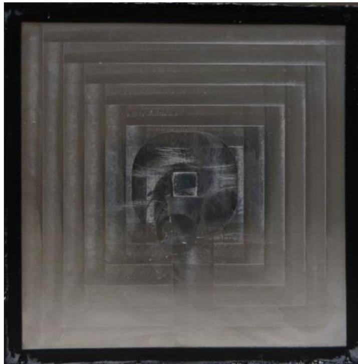
**Figure 4.5: 0.5 cm<sup>2</sup> central clad spot panel with corrosion resistant tape**
