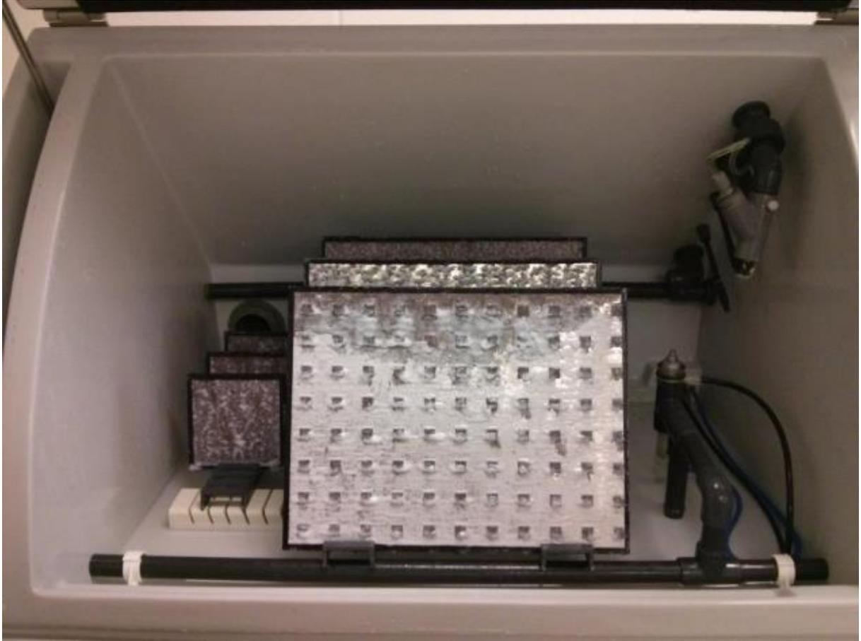
**Figure 4.1: Inside of the salt spray chamber**
