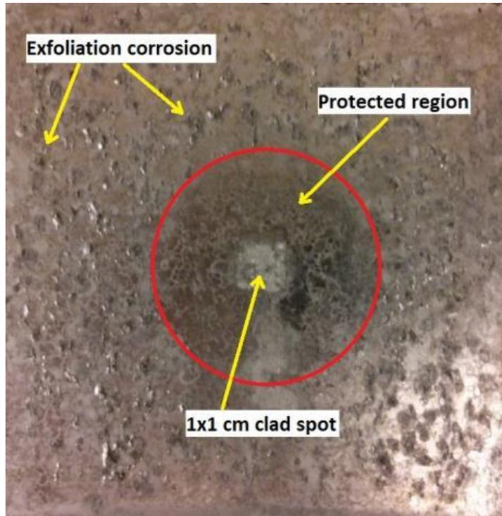
Figure 5.1: Cleaned central clad spot panel
