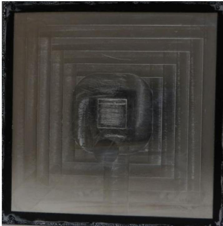
Figure 4.7: 2 cm<sup>2</sup> central clad spot panel with corrosion resistant tape
