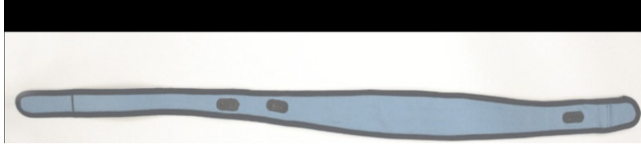
Figure 2.4: Wearable belt approach with three integrated dry electrodes for monitoring patient's ECG and activity [45]
