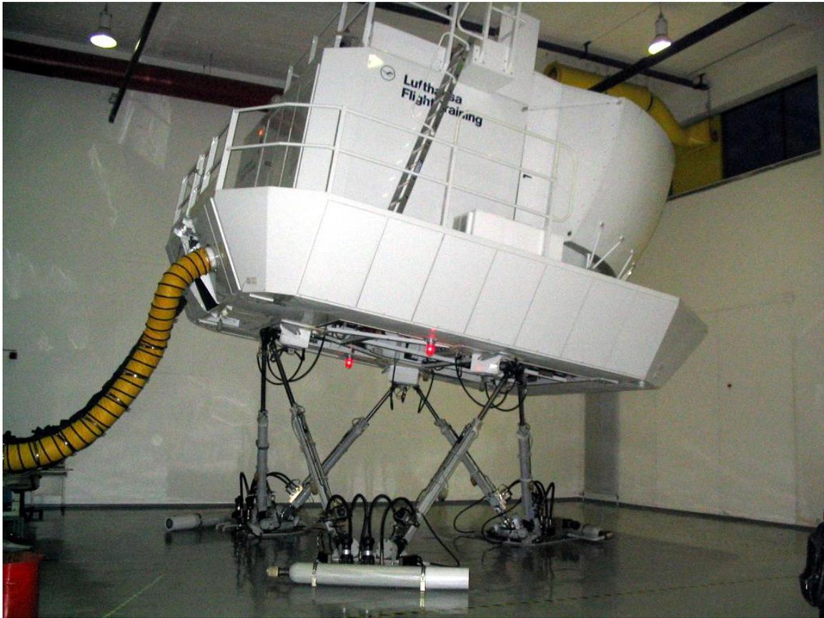
*Figure 2-13 Lufthansa flight simulator on 6-axis platform based on Stewart platform (courtesy of Lufthansa) [49]*
