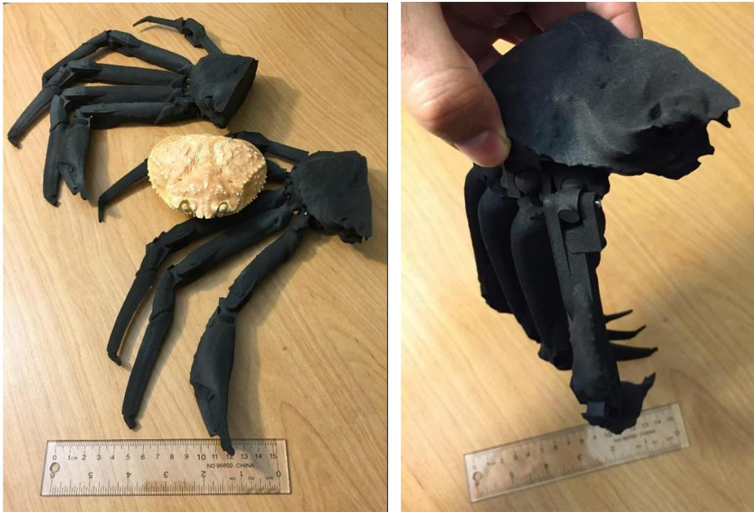
**Figure 3-10** *The fully articulated snow crab produced by SLS*
