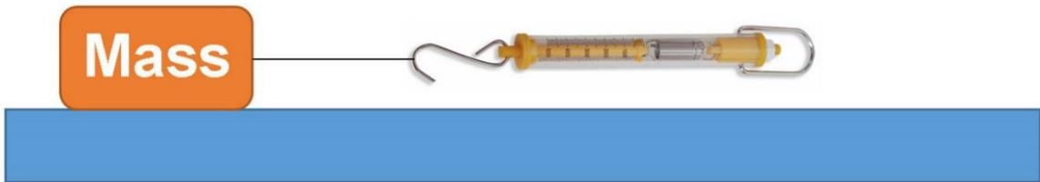
*Figure 6-2 Schematic diagram of static frictional test setup - spring balance method*
