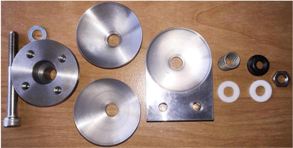
*Figure 5-2 The conical joint parts*
