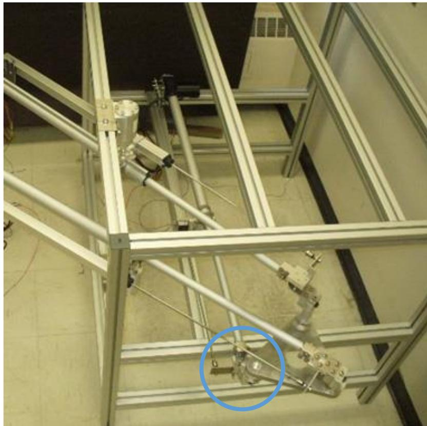
*Figure 5-3 The fabricated conical joint installed on the 3-RPR planar parallel robot at the High Performance Robot Lab at Memorial University*
