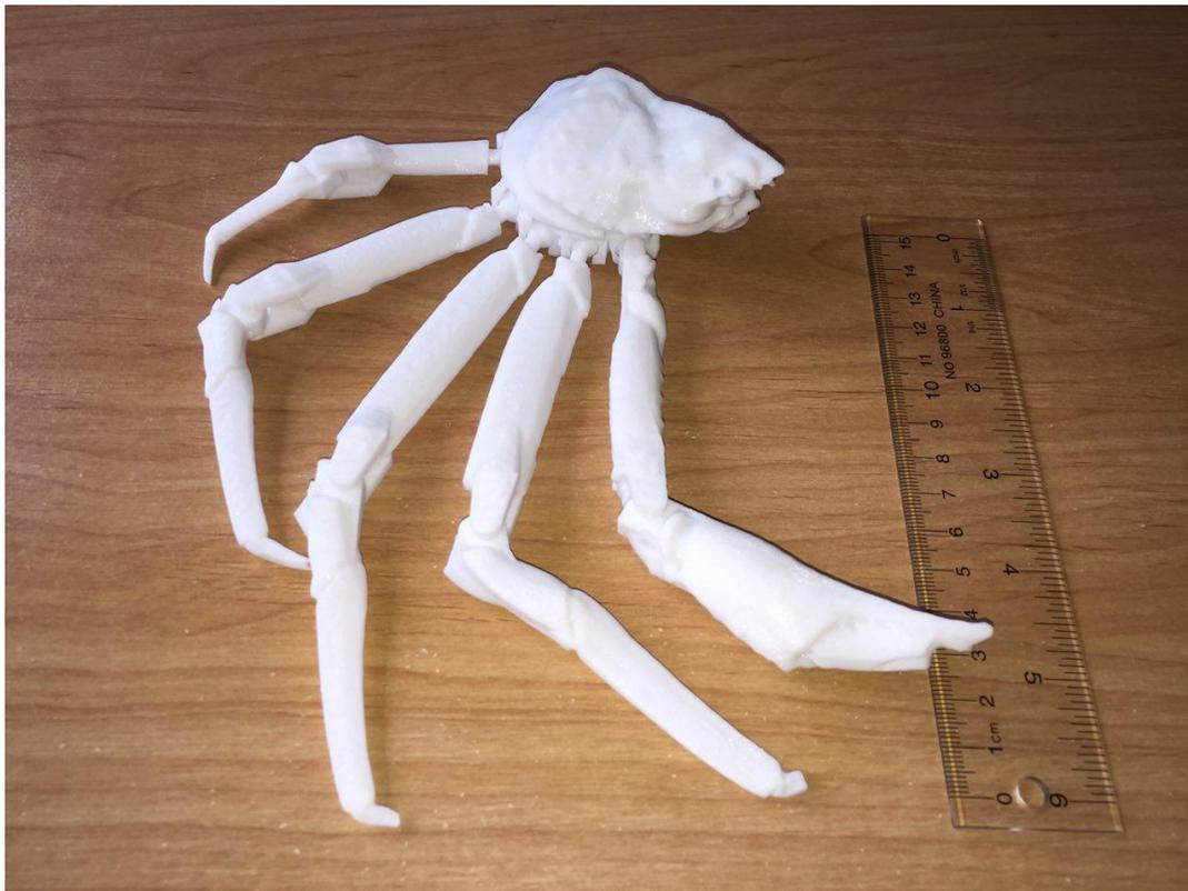
*Figure 3-9 The fully articulated snow crab produced by FDM (the scale factor 0.7:1)*
