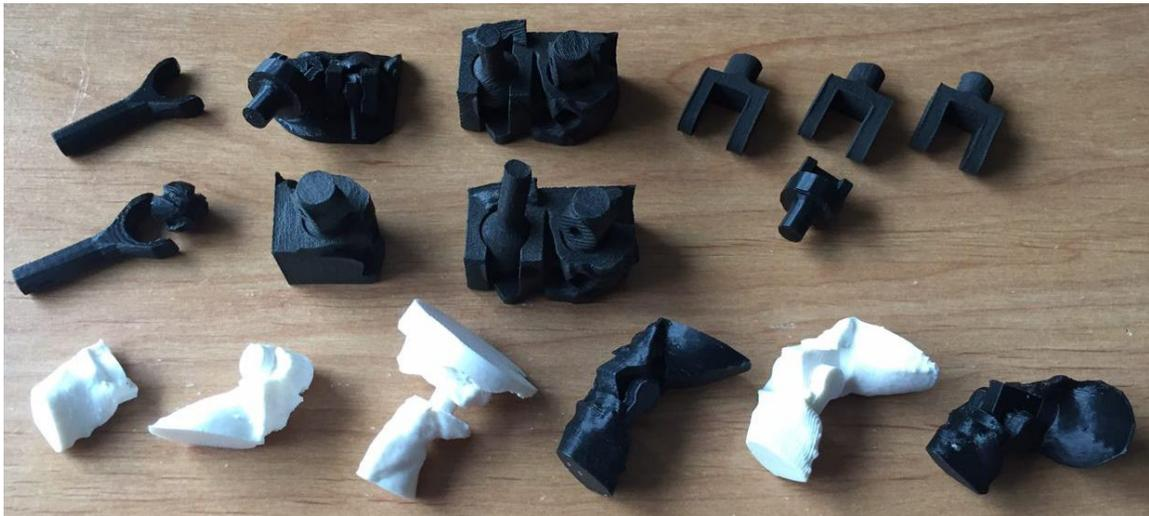
*Figure 3-8 Different trials with various tolerances*
