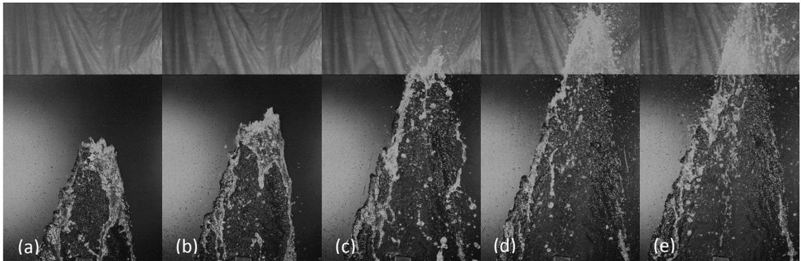
Figure 4.11: Change in water sheet area ( $A$ ) on a vertical surface at  $\theta = 20^\circ$  and  $V$  for (a) 2.4 m/s, (b) 3.2 m/s, (c) 4.8 m/s, (d) 6.4 m/s, and (e) 8 m/s.
