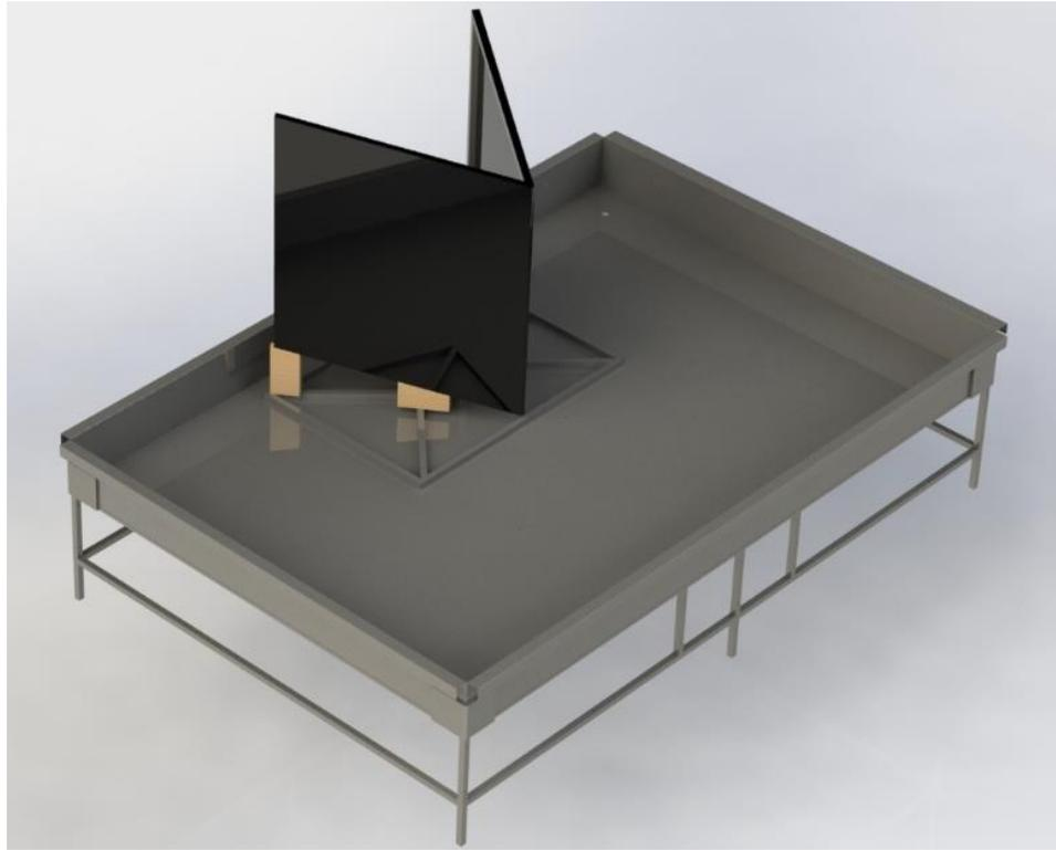
Figure 3.5: CAD drawing of the target surface and water enclosure assembly.
