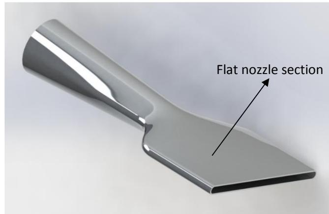
Figure 3.6: CAD drawing of customized flat nozzle, machine pressed from a circular Stainless steel tube.
