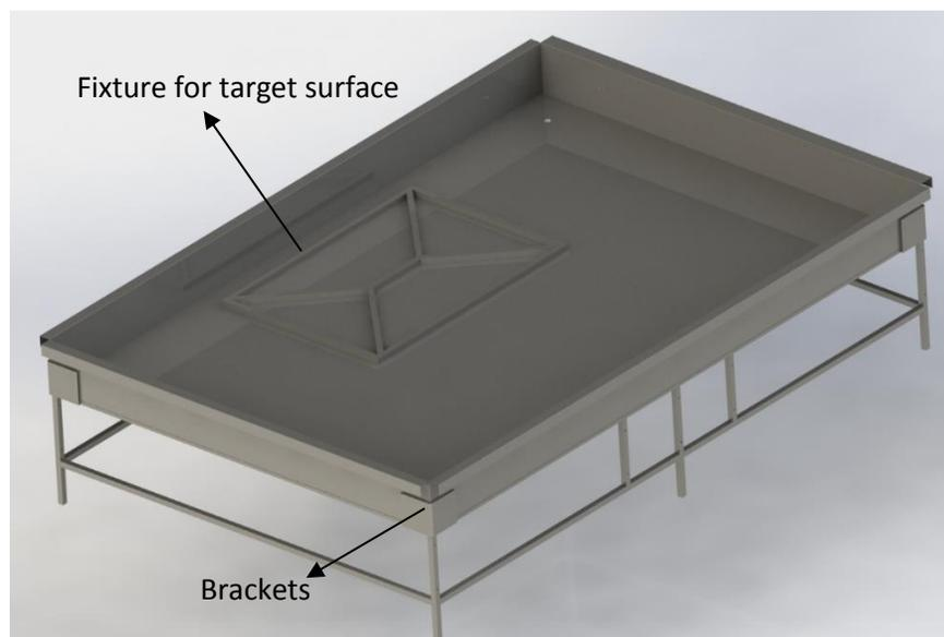
Figure 3.2: CAD drawing of the water enclosure with a fixture for target surface.
