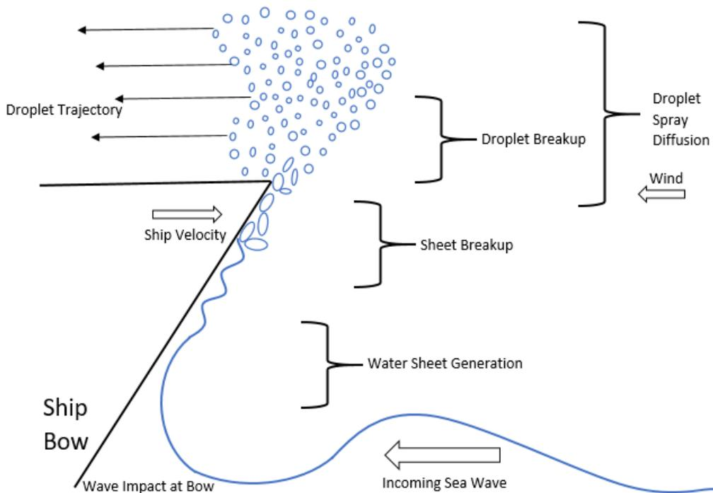
Figure 2.1: A typical wave impact and breakup stages.
