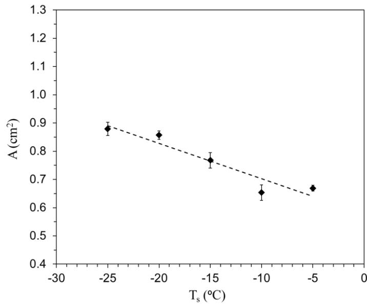
Figure 4.18: Variation of splash area ( $A$ ) upon impact for  $d = 2$  mm saline droplet falling from  $h = 130$  cm at various surface temperature. Linear regression of the experimental data points is also shown.
