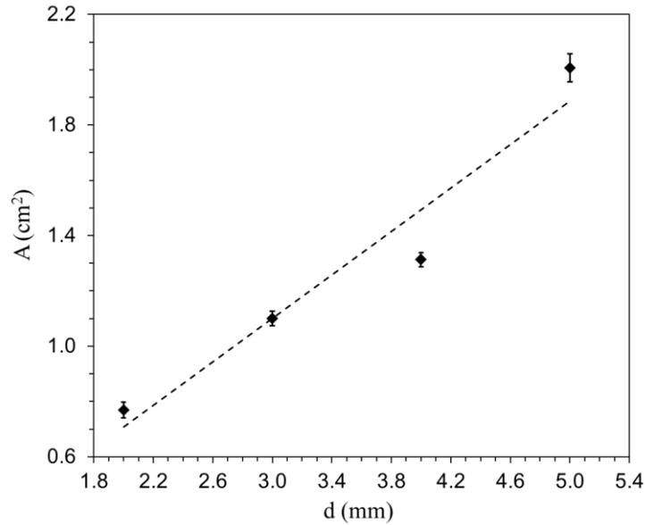
Figure 4.15: Splash area ( $A$ ) for droplets upon impact on a cold surface at  $T_s = -25^{\circ}\text{C}$  and  $h = 130$  cm. Linear regression of the experimental data points is also shown.
