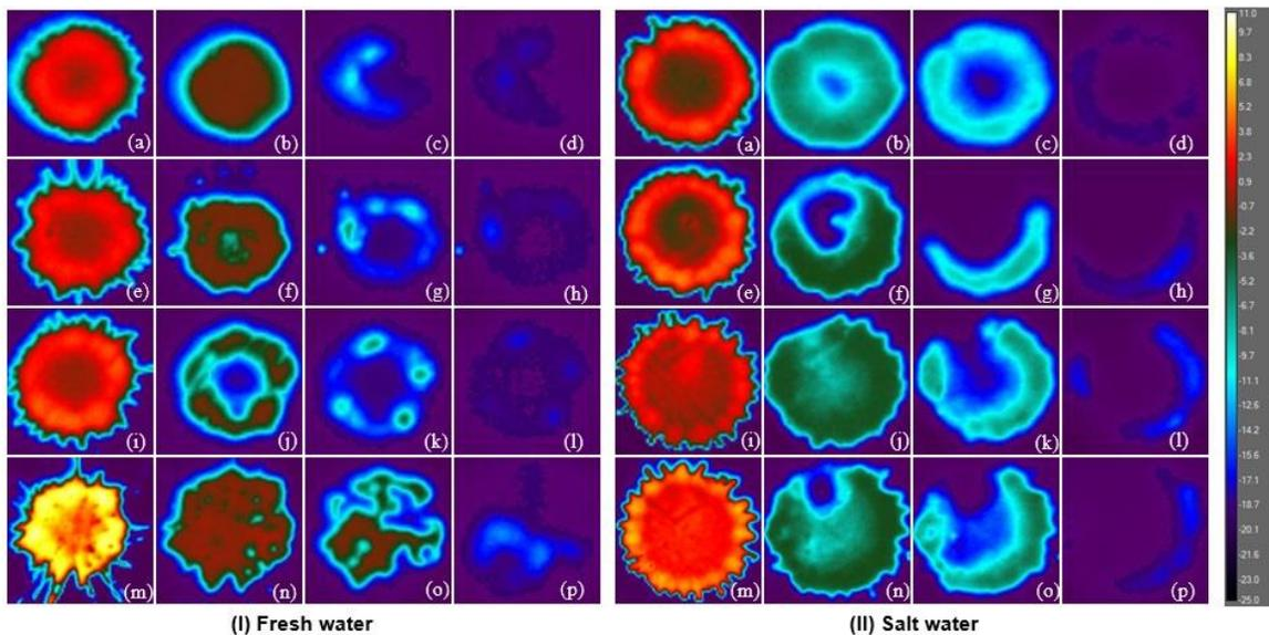
Figure 4.19: Thermal images in sequence for  $d = 2$  mm (a to d), 3 mm (e to h), 4 mm (i to l) and 5 mm (m to p) droplet falling from  $h = 130$  cm (I) Fresh water (II) Salt water.
