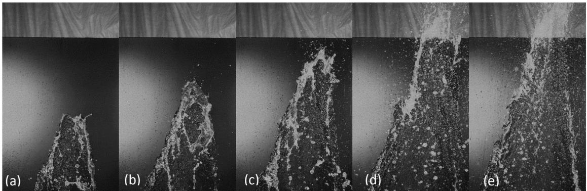
Figure 4.9: Change in water sheet area ( $A$ ) on a vertical surface at  $\theta = 10^\circ$  and  $V$  for (a) 2.4 m/s, (b) 3.2 m/s, (c) 4.8 m/s, (d) 6.4 m/s, and (e) 8 m/s.
