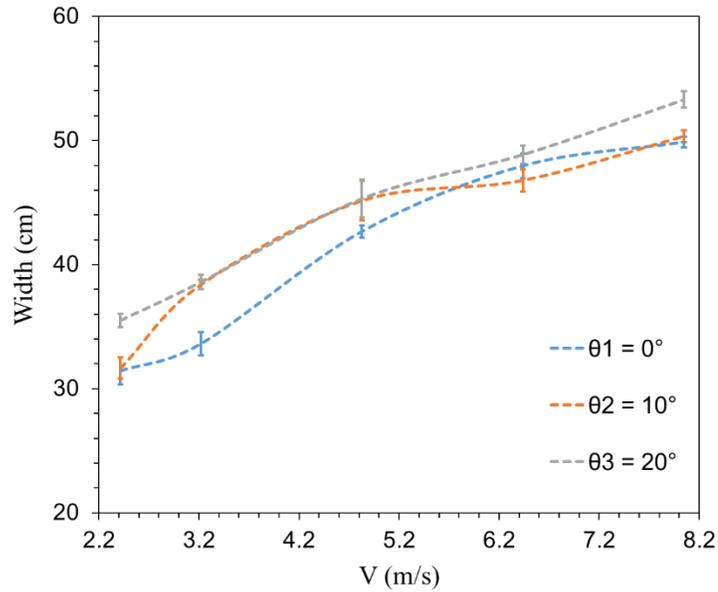
Figure 4.2: Variation of water sheet width ( $W$ ) for resulting fluid impact on a vertical surface ( $\theta = 0^\circ \sim 20^\circ$ ,  $V = 2.4$  to  $8$  m/s).
