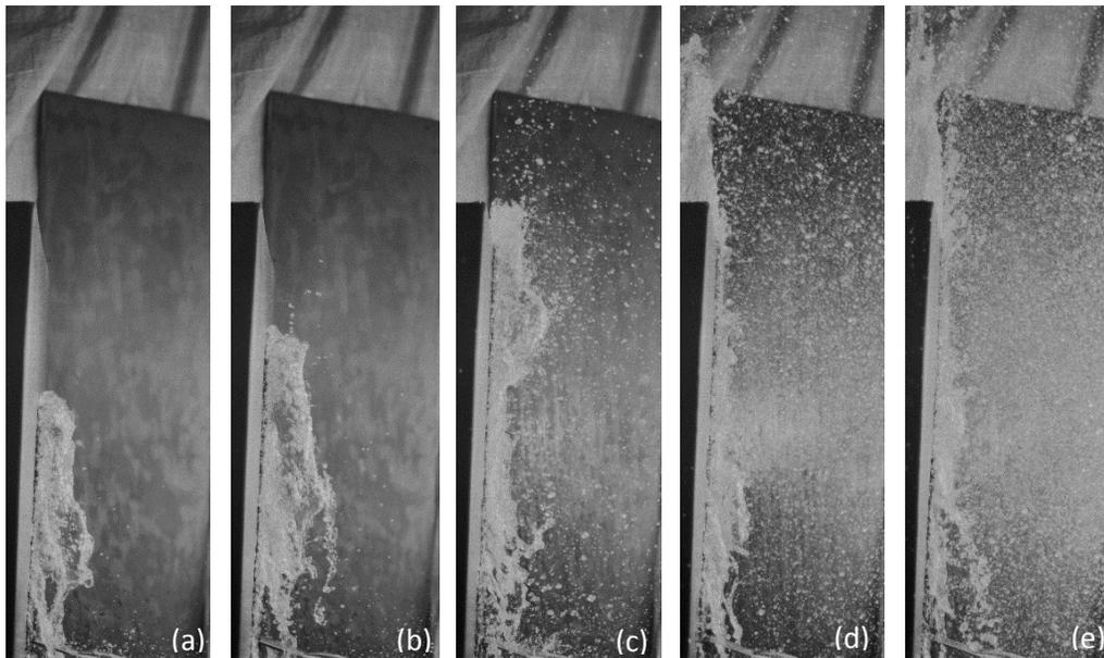
Figure 4.8: Variation of water sheet height ( $H$ ) at  $\theta = 20^\circ$  and  $V$  for (a) 2.4 m/s, (b) 3.2 m/s, (c) 4.8 m/s, (d) 6.4 m/s, and (e) 8 m/s.
