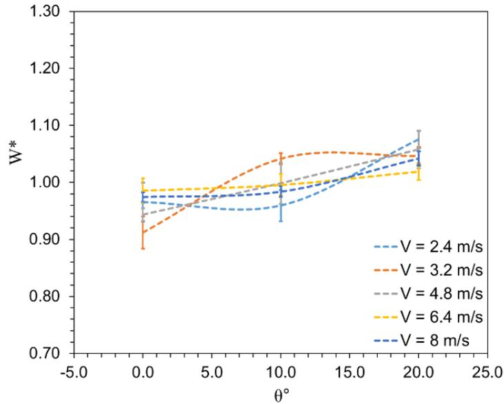
Figure 4.4: Variation of dimensionless width ( $W^*$ ) upon impact on a vertical surface ( $\theta = 0^\circ \sim 20^\circ$ ,  $V = 2.4$  to  $8$  m/s).
