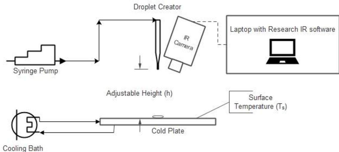
Figure 3.9: Schematic of the experimental setup.
