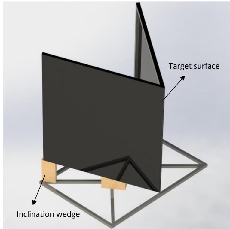
Figure 3.4: Target surface on adjustable inclination-wedge and tank fixture.
