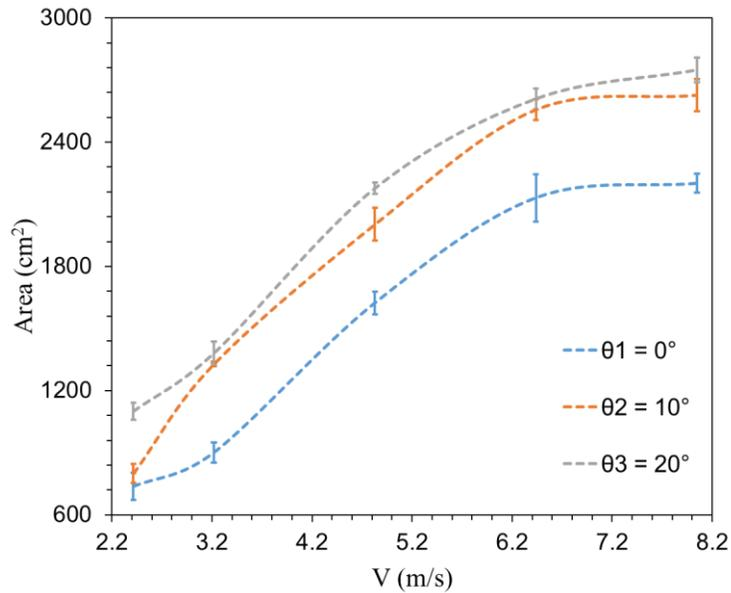
Figure 4.10: Change in water sheet area (A) for resulting fluid impact on a vertical surface ( $\theta = 0^\circ \sim 20^\circ$ ,  $V = 2.4$  to  $8$  m/s).
