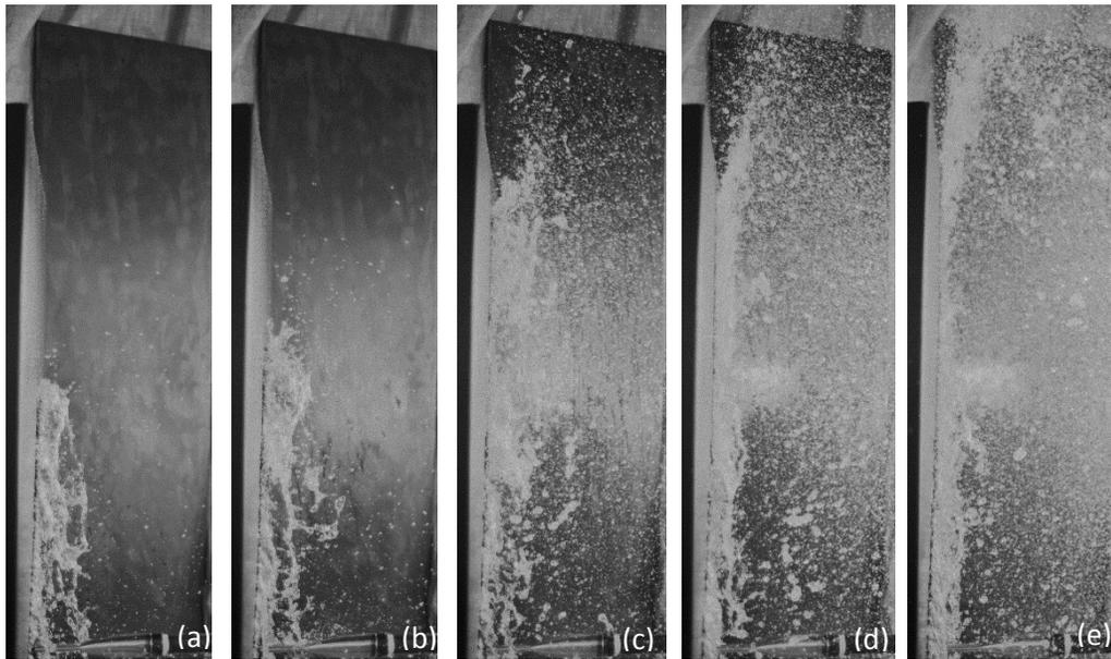
Figure 4.3: Variation of water sheet height ( $H$ ) at  $\theta = 0^\circ$  and  $V$  for (a) 2.4 m/s, (b) 3.2 m/s, (c) 4.8 m/s, (d) 6.4 m/s, and (e) 8 m/s.
