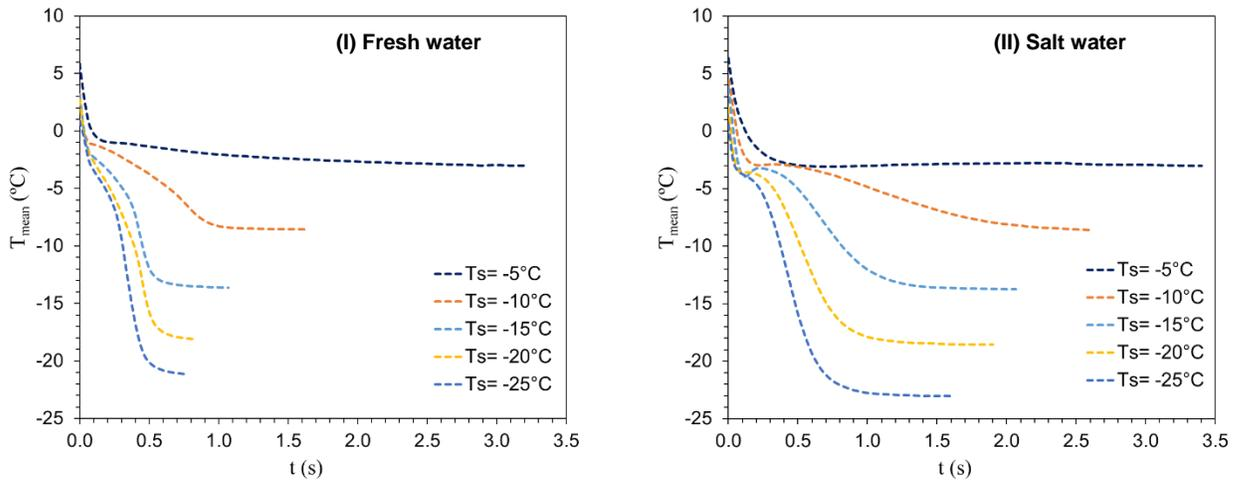
Figure 4.22: Variation of mean temperature for  $d = 2$  mm droplet falling from  $h = 130$  cm at various surface temperature (I) Fresh water (II) Salt water.
