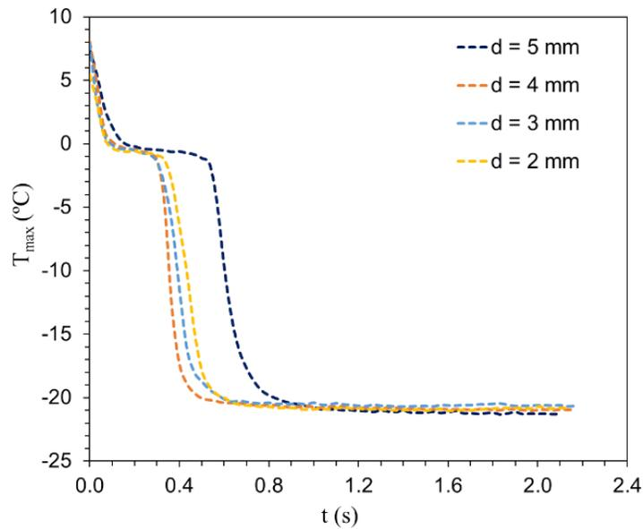
Figure 4.13: Variation of maximum temperature of droplet splash on a cold surface ( $T_s = -25^\circ\text{C}$ ,  $h = 130$  cm).
