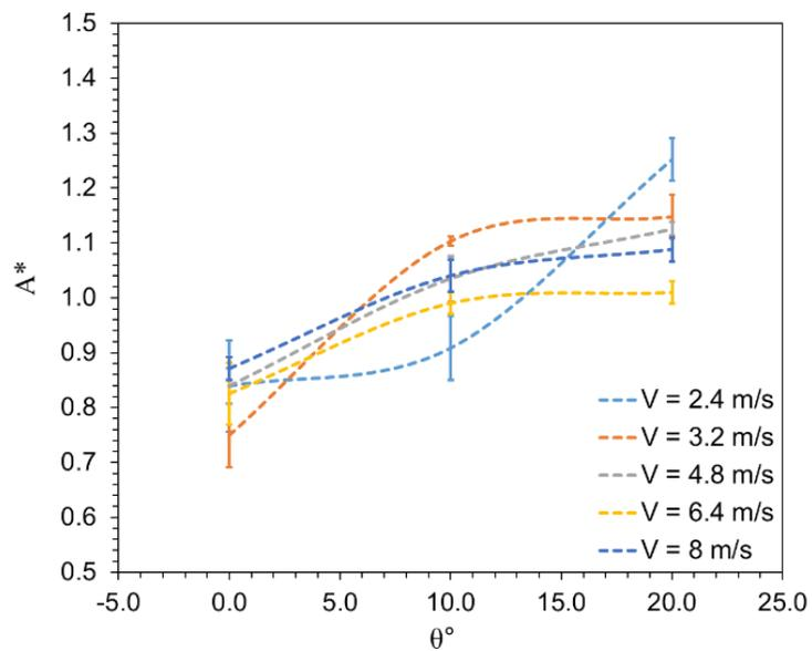
Figure 4.12: Variation of dimensionless area ( $A^*$ ) upon impact on a vertical surface ( $\theta = 0^\circ \sim 20^\circ$ ,  $V = 2.4$  to 8 m/s).
