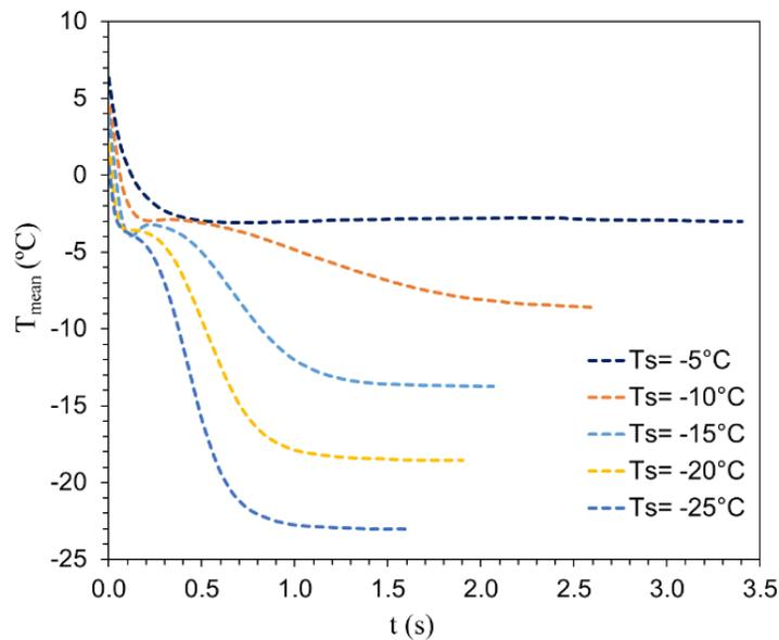
Figure 4.16: Variation of mean temperature for  $d = 2$  mm droplet falling from  $h = 130$  cm at various surface temperature.
