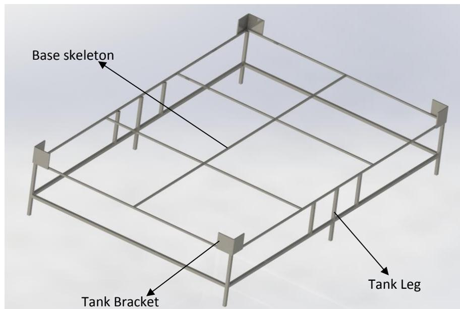
Figure 3.3: CAD drawing of the tank base
