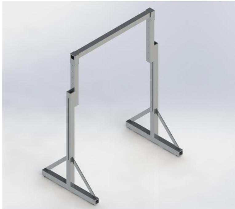
Figure 3.10: Customized support stand for IR/High-speed camera.
