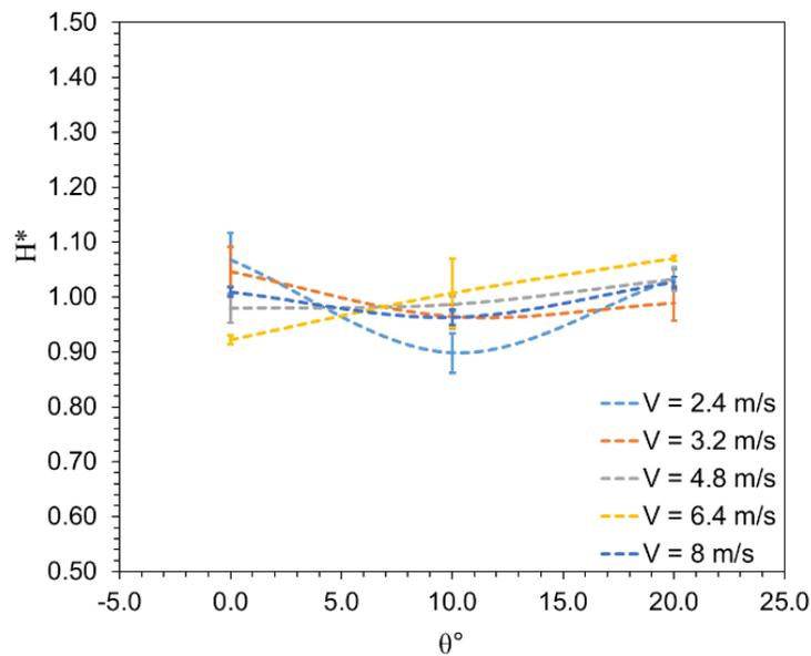
Figure 4.7: Variation of dimensionless height ( $H^*$ ) upon impact on a vertical surface ( $\theta = 0^\circ \sim 20^\circ$ ,  $V = 2.4$  to 8 m/s).
