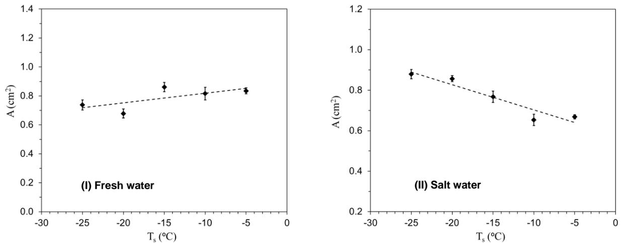
Figure 4.23: Variation of splash area ( $A$ ) upon impact for  $d = 2$  mm saline droplet falling from  $h = 130$  cm at various surface temperature.
