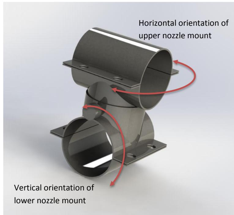
Figure 3.7: CAD drawing of customized nozzle mount, allowing vertical and horizontal orientation of the nozzle.
