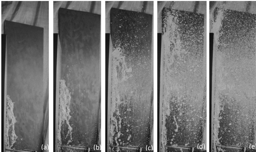
Figure 4.6: Variation of water sheet height (H) at  $\theta = 10^\circ$  and V for (a)  $2.4$  m/s, (b)  $3.2$  m/s, (c)  $4.8$  m/s, (d)  $6.4$  m/s, and (e)  $8$  m/s.
