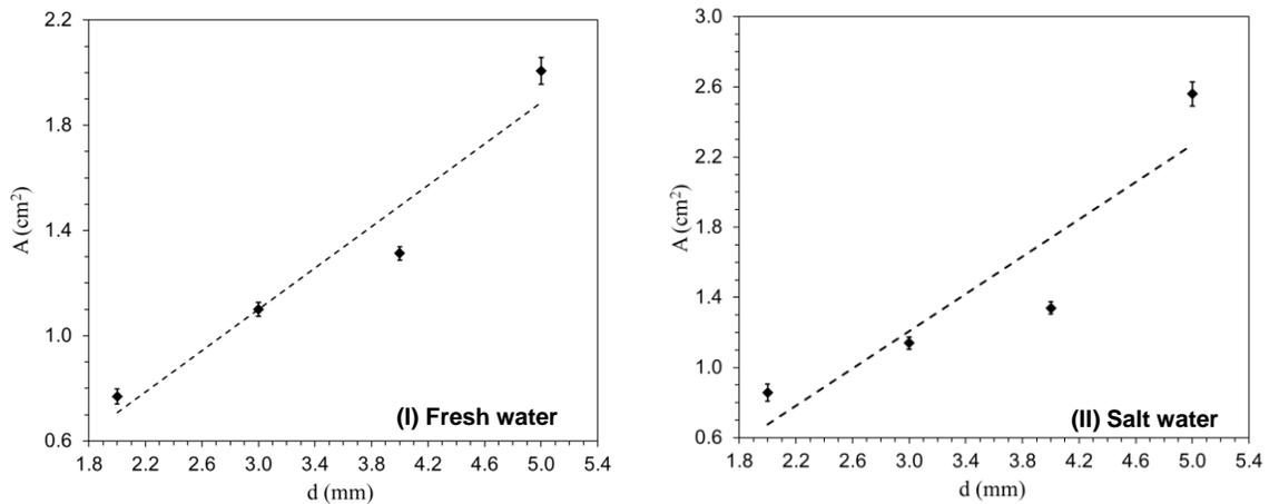
Figure 4.20: Splash area ( $A$ ) for  $d = 2, 3, 4, 5$  mm droplet upon impact on a cold surface at  $T_s = -25^\circ\text{C}$  and  $h = 130$  cm. (I) Fresh water (II) Salt water.
