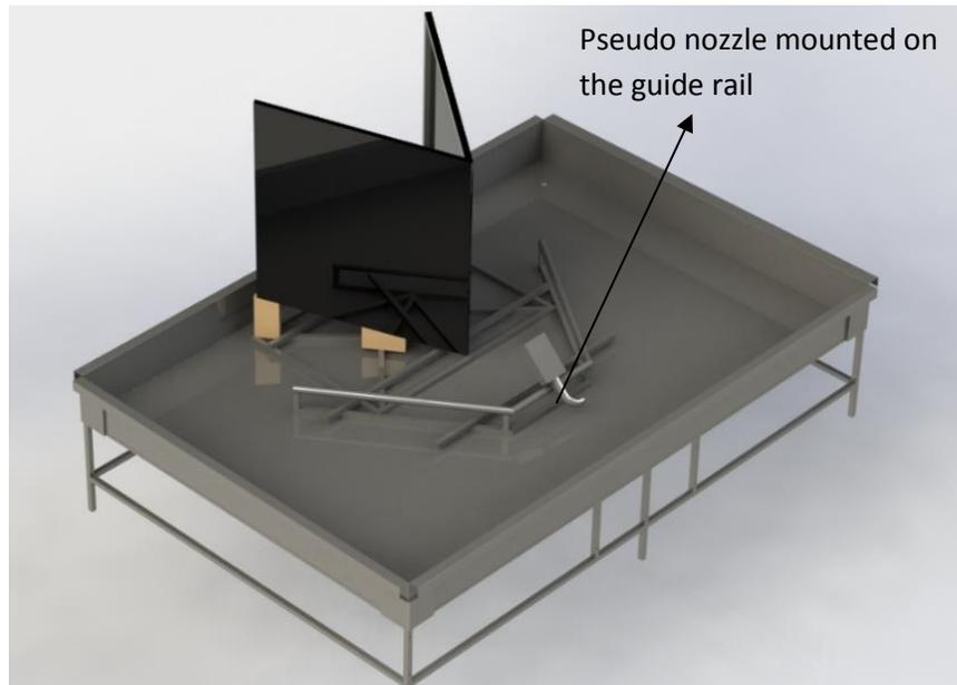
Figure 3.8: Fluid impact and breakup setup with nozzle mount targeted at the test subject.
