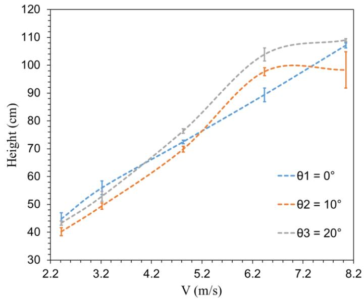
Figure 4.5: Variation of water sheet height (H) for resulting fluid impact on a vertical surface ( $\theta = 0^\circ \sim 20^\circ$ ,  $V = 2.4$  to  $8$  m/s).
