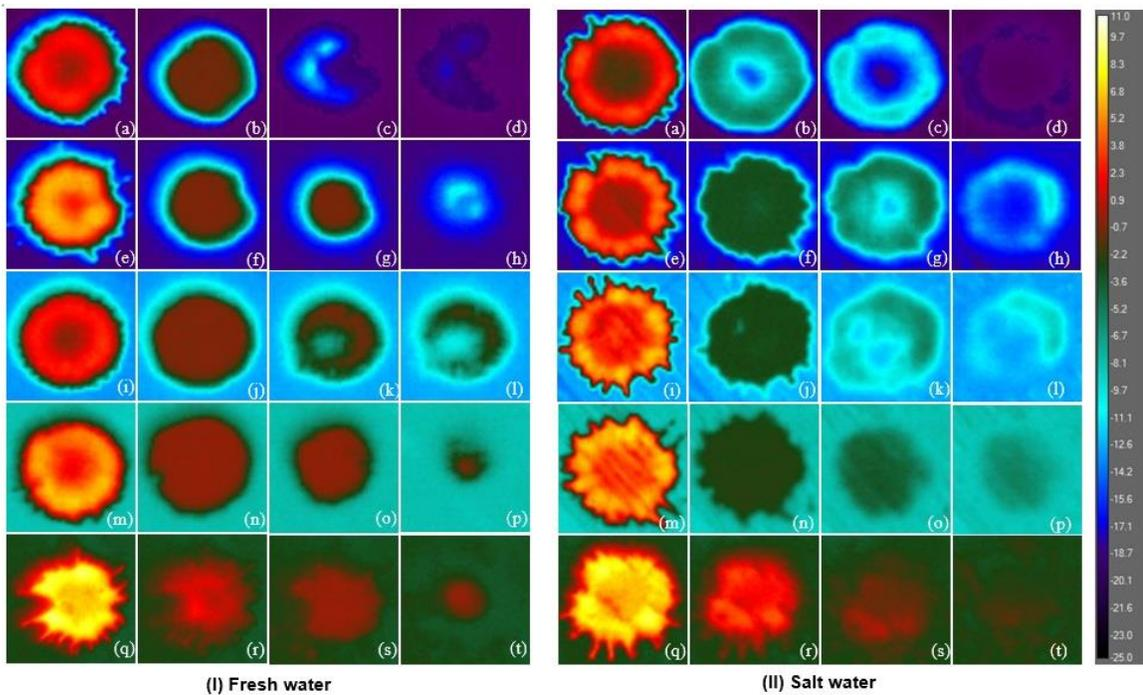
Figure 4.21: Thermal images on impact for  $d = 2$  mm saline droplet falling from  $h = 130$  cm at  $T_s = -25^\circ\text{C}$ ,  $-20^\circ\text{C}$ ,  $-15^\circ\text{C}$ ,  $-10^\circ\text{C}$  and  $-5^\circ\text{C}$  (I) Fresh water (II) Salt water.
