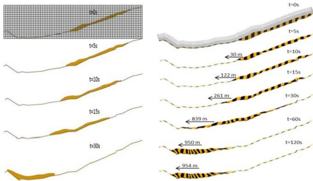
**Figure 2.3:** Progression of landslide: (left) CEL and (right) MPM
