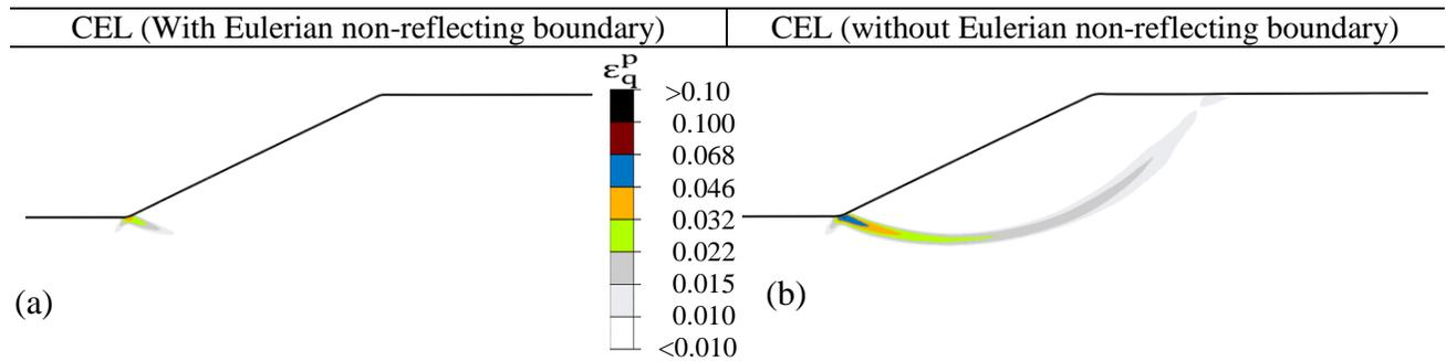
**Figure 3.8:** Effect of including non-reflecting outflow Eulerian boundary conditions in Abaqus/CEL analyses (shown for Parkfield earthquake input motion)
