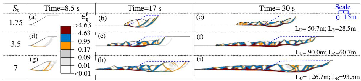
**Figure 4.7:** Effect of sensitivity on failure of Slope-I
