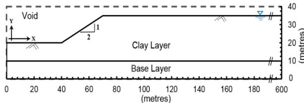
Figure 1. Geometry of the slope used in Finite Element (FE) modeling
