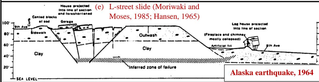
**Figure 1.1:** Some air photographs and interpreted shear zones for historical earthquake induced landslides in sensitive clay slopes
