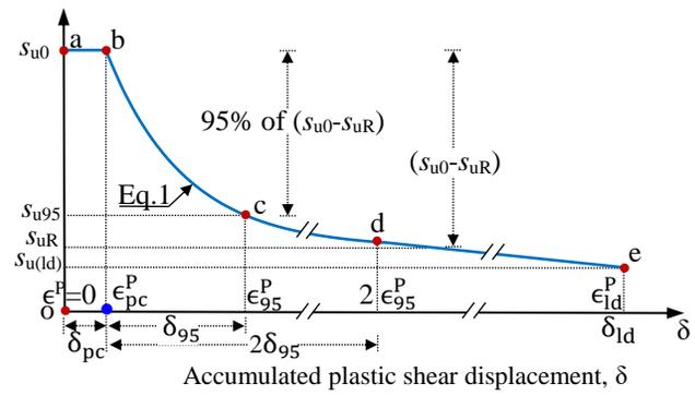
**Figure 4.3:** Stress strain behaviour used in FE modeling
