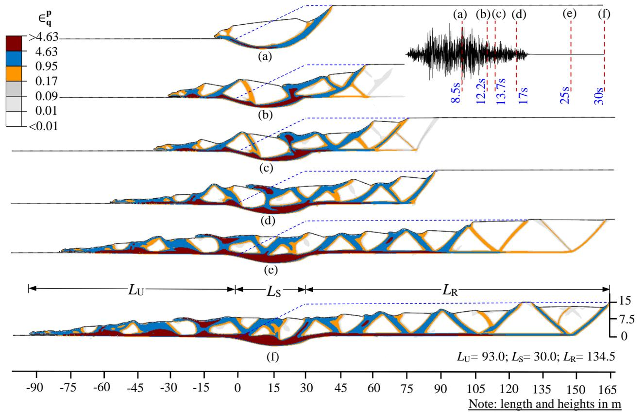
**Figure 4.13:** Slope-IV: Development of failure surfaces
