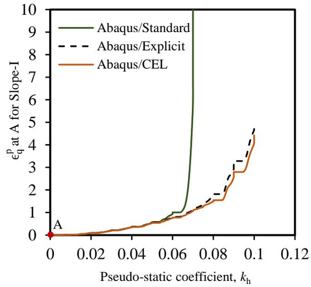
**Figure 3.3:** Comparison of  $\epsilon_q^p$  at the integration point A with variations of pseudostatic coefficients ( $k_h$ )
