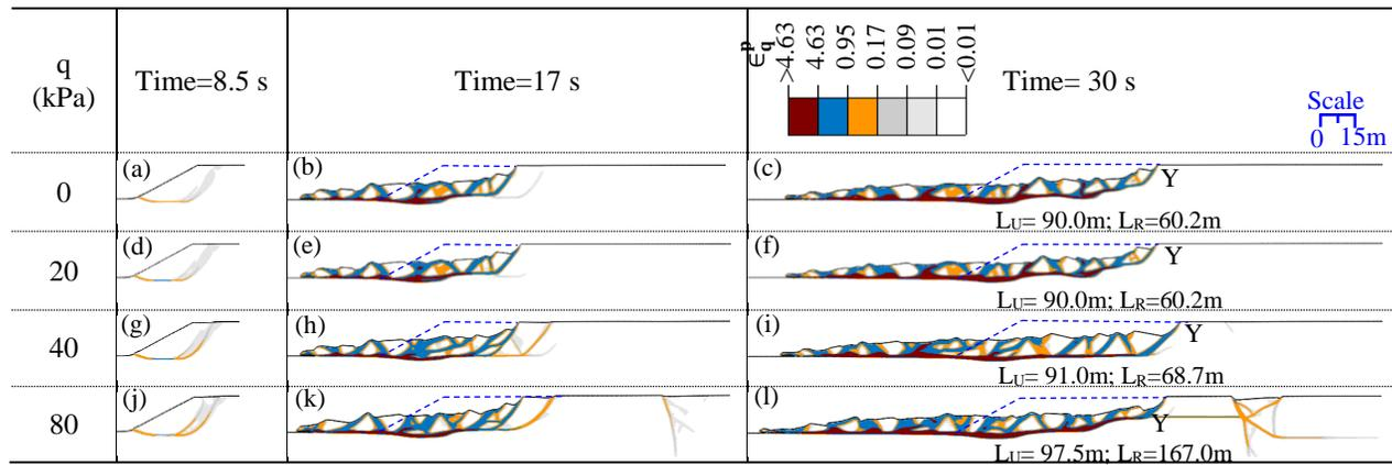
**Figure 4.12:** Slope-III: Effect of variation in distributed loads
