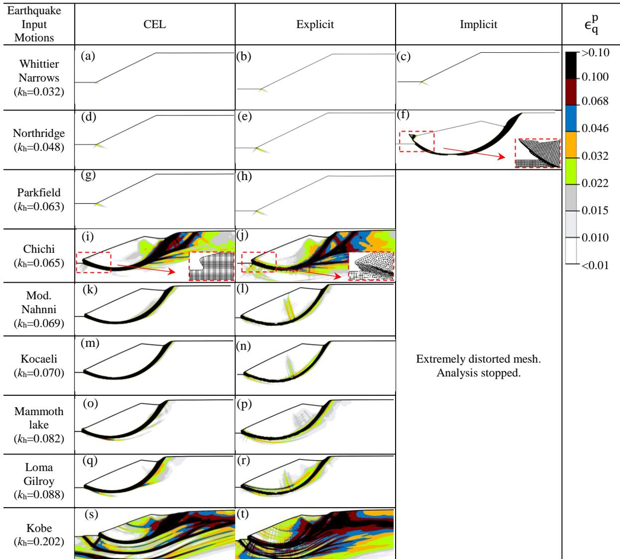
**Figure 3.10:** Dynamic analyses for post-peak softening soil condition by three FE modeling approaches.
