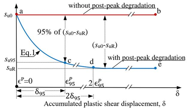
**Figure 3.6:** Stress strain behaviour used in FE modeling
