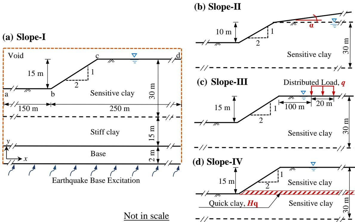
**Figure 4.1:** Model geometries of sensitive clay slopes (a) Slope-I:horizontal ground surface; (b) Slope- II: slightly inclined upslope ground surface; (c) Slope-III: with upslope distributed load and (d) Slope- IV: quick clay layer at toe depth
