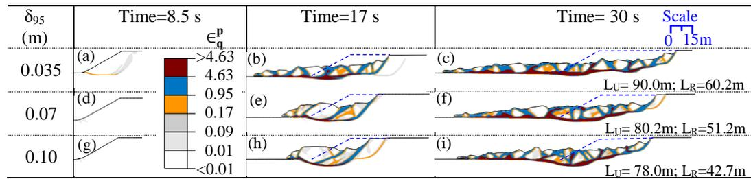
**Figure 4.6:** Effect of  $\delta_{95}$  on failure of Slope-I
