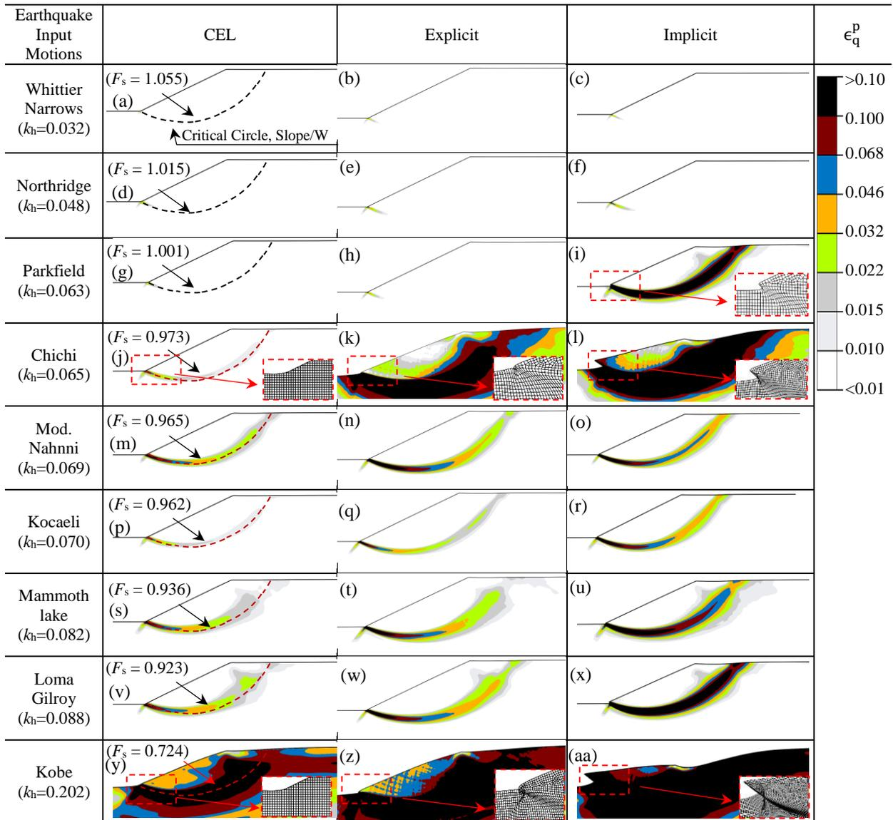
**Figure 3.9:** Dynamic analysis for perfectly plastic soil condition by three FE modeling approaches
