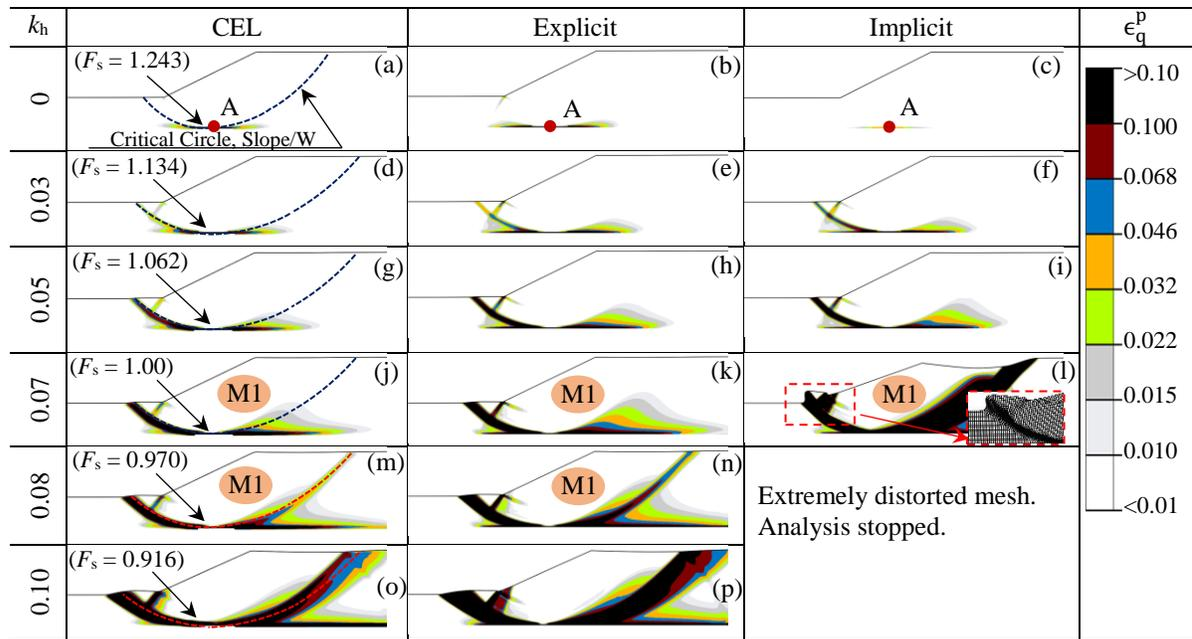
**Figure 3.2:** Pseudostatic analyses for Slope-I using three FE modeling approaches
