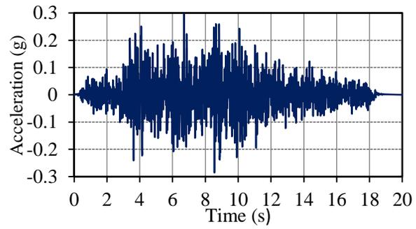
**Figure 4.2:** Reference acceleration time history modified from the 1985 Nahanni earthquake in Nahanni region, Northwest Territories, Canada
