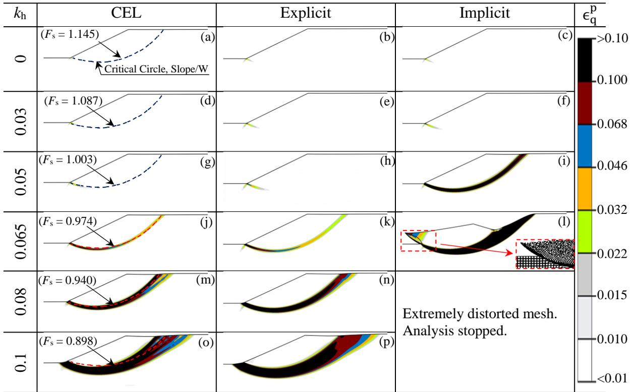
**Figure 3.4:** Pseudostatic analyses for Slope-II using three FE modeling approaches
