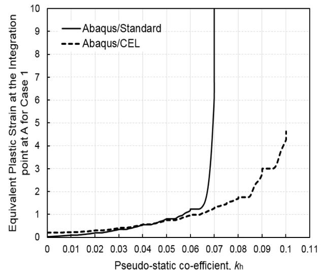
Figure 3. Comparison of Equivalent plastic strain at the Integration point near point A (in Fig. 2) with variations of pseudostatic coefficients ( $k_h$ ).
