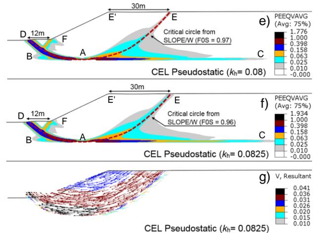
Figure 2. Formation of shear bands and failure planes for uniform undrained shear strength of clay (Case-1)
