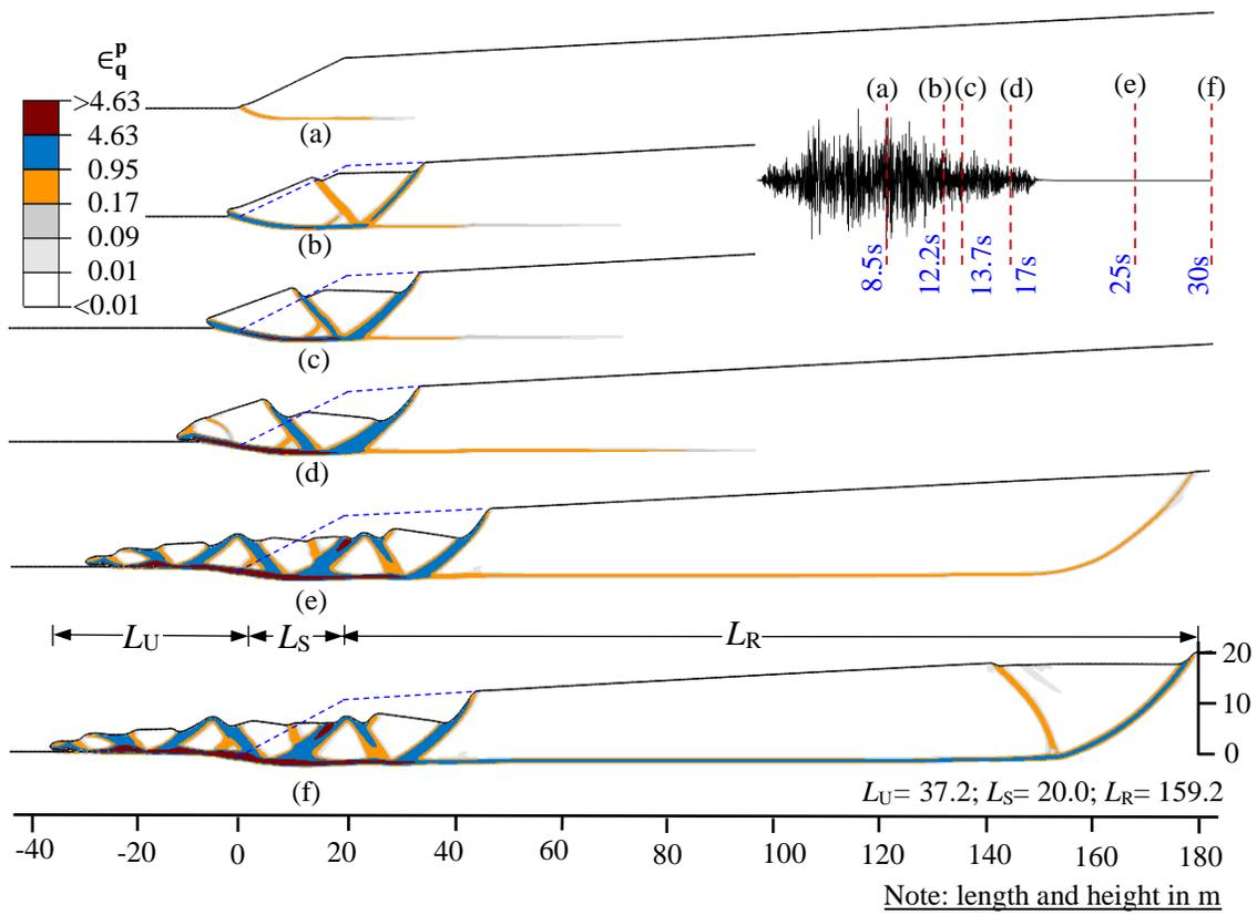
**Figure 4.9:** Slope-II: Development of failure surfaces
