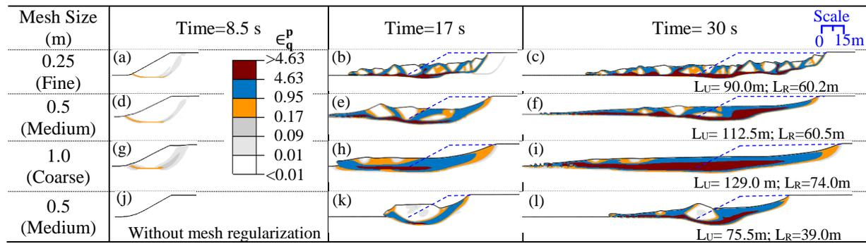
**Figure 4.5:** Effect of FE mesh size on the formation of failure surfaces (Slope-I)
