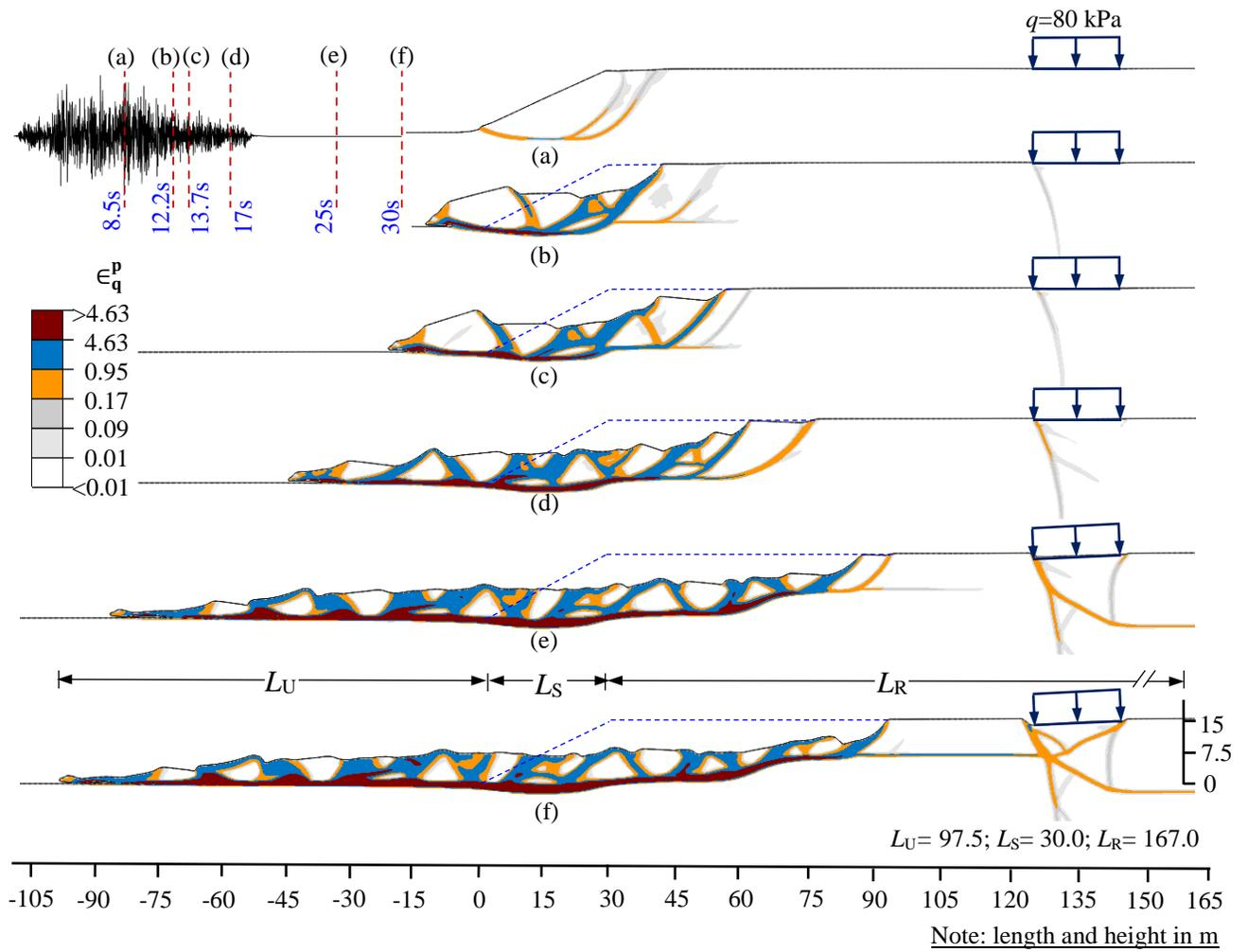
**Figure 4.11:** Slope-III: Development of failure surfaces
