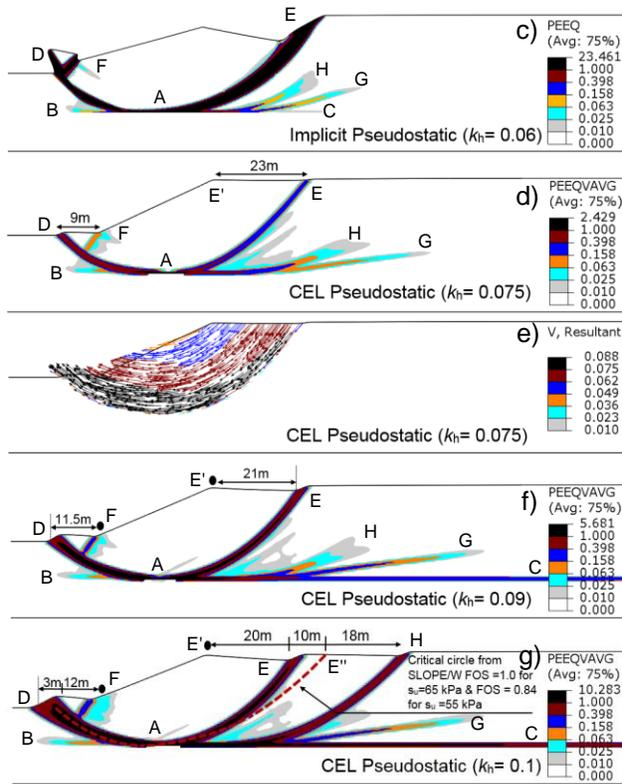
Figure 5. Analyses with post-peak degradation of undrained shear strength of clay (Case-3)
