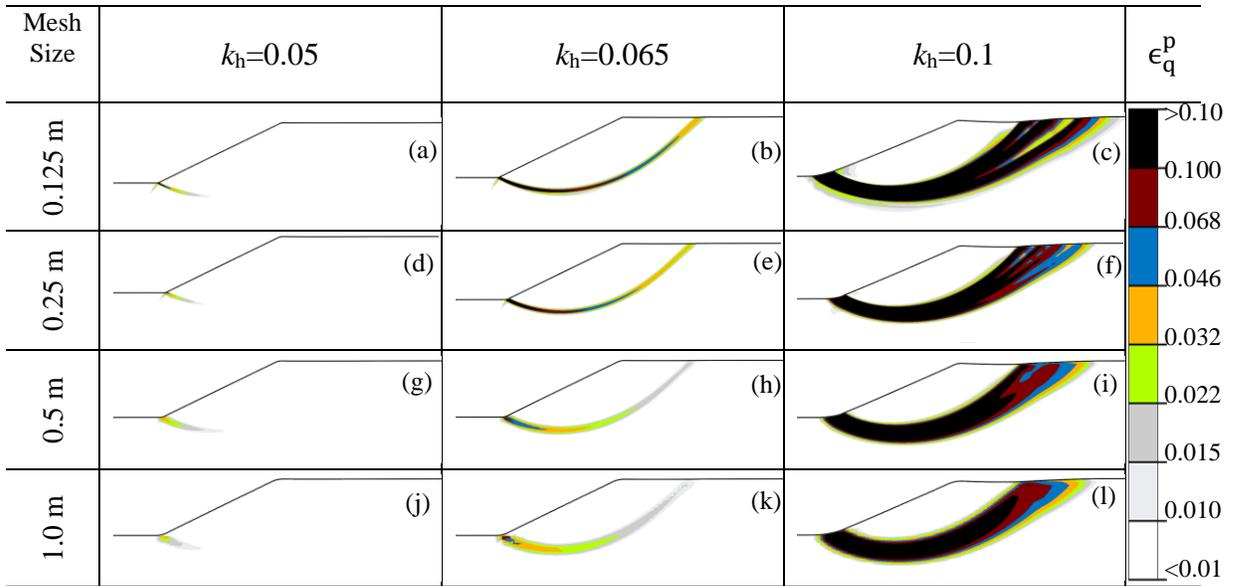
**Figure 3.5:** Mesh size effects on FE results based on pseudostatic analyses in Slope-II.
