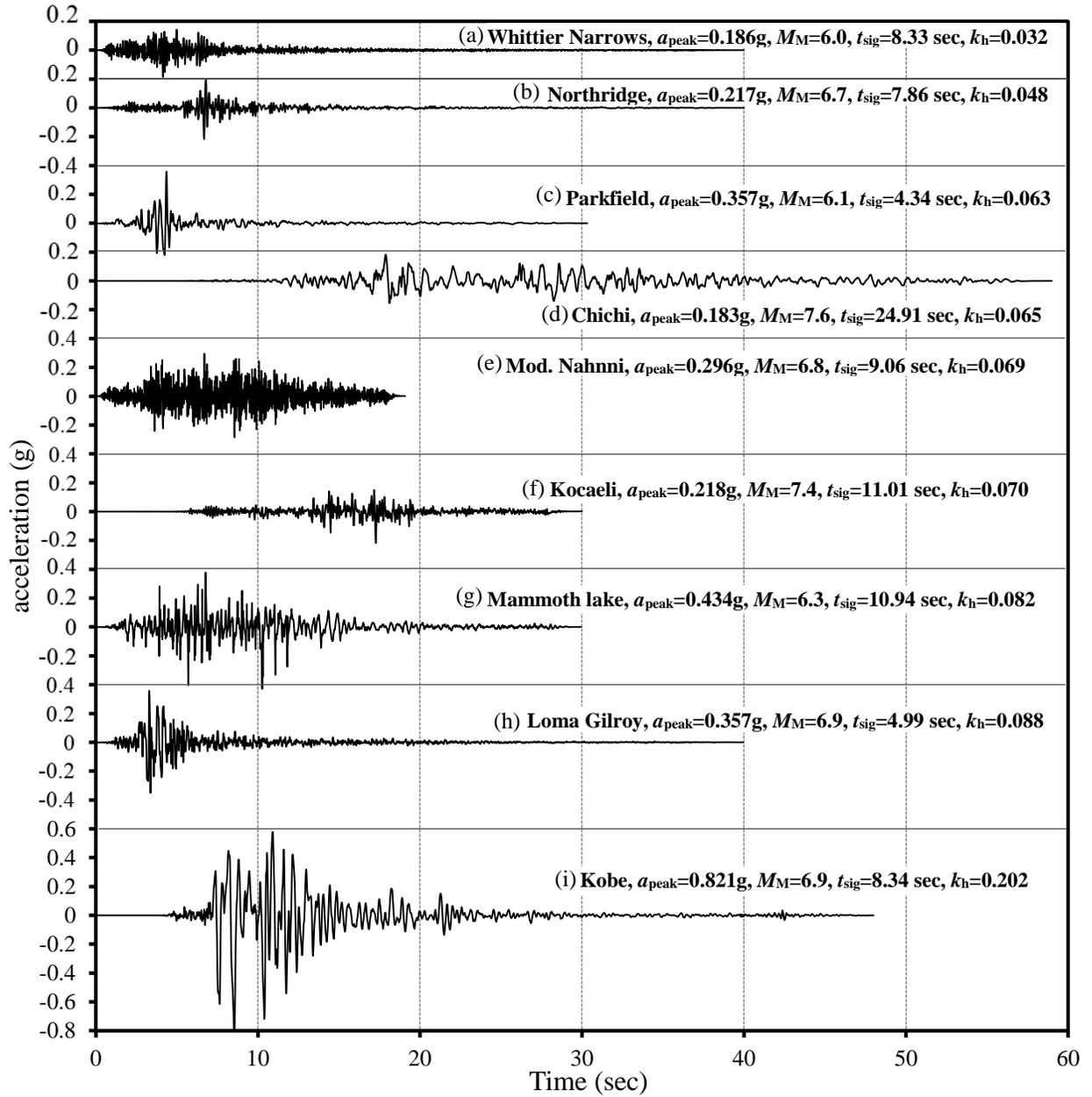
**Figure 3.7:** Acceleration time histories as reference earthquake input motions used in numerical simulation
