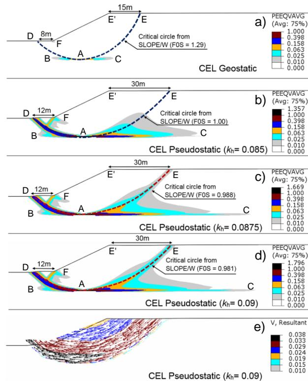
Figure 4. Shear strains and instantaneous velocity for undrained shear strength variations with depth of clay (Case-2)
