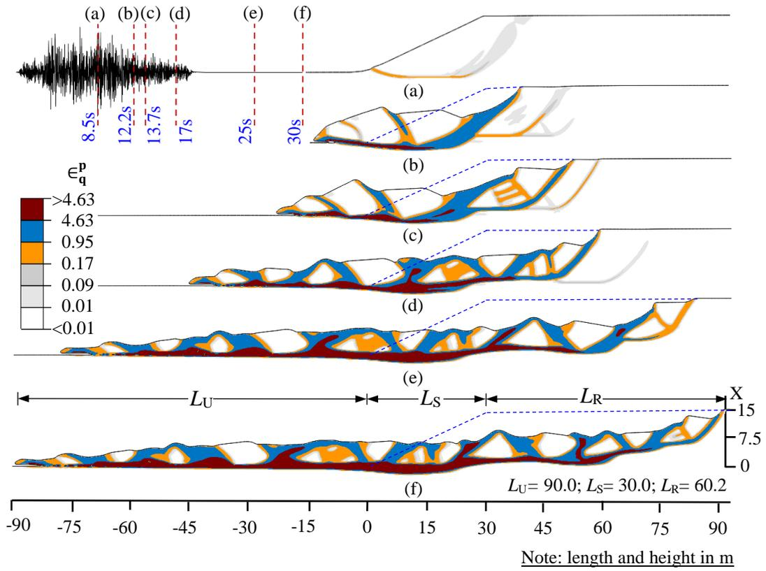
**Figure 4.4:** Slope-I: Development of failure surfaces
