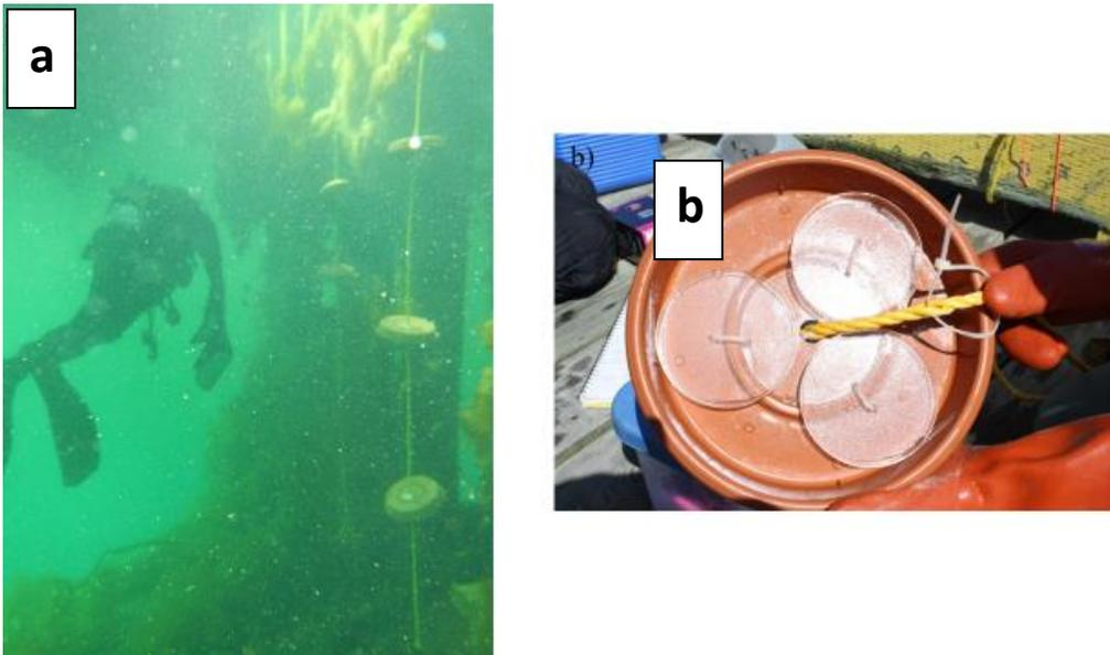
Figure 2.3.3.2: Collector design: a) Collectors suspended in the water column; b) plates zip-tied to bases on collectors.
