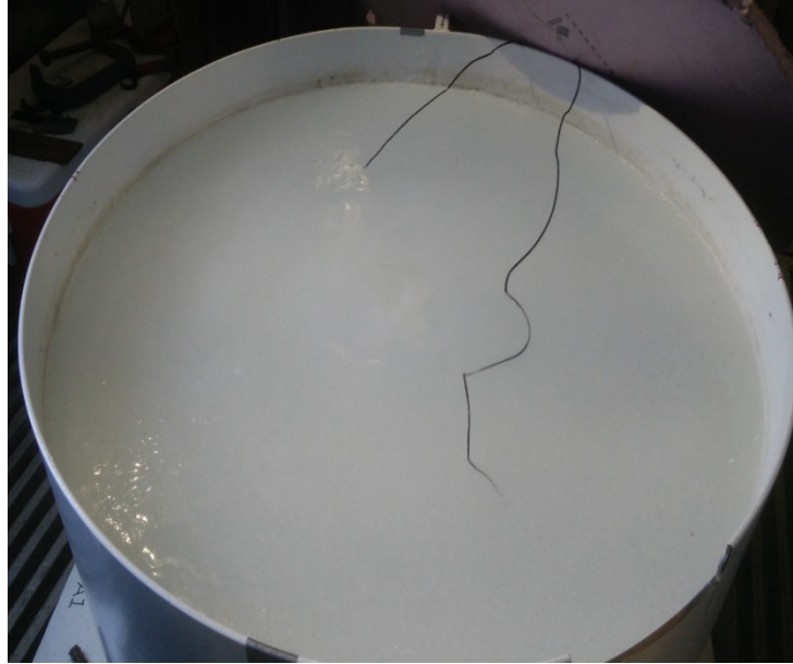
Figure 3.9: RTD probes placed in an ice specimen.
