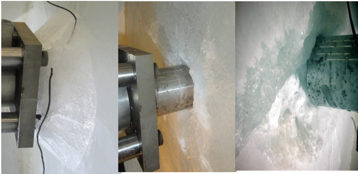
Figure 5.5: Images taken after indentation tests (100mm indenter; 2.5 mm/s) at temperatures: (Left) -1^{\circ}\text{C} ; (Centre) -7^{\circ}\text{C} ; (Right) -18.5^{\circ}\text{C} .
