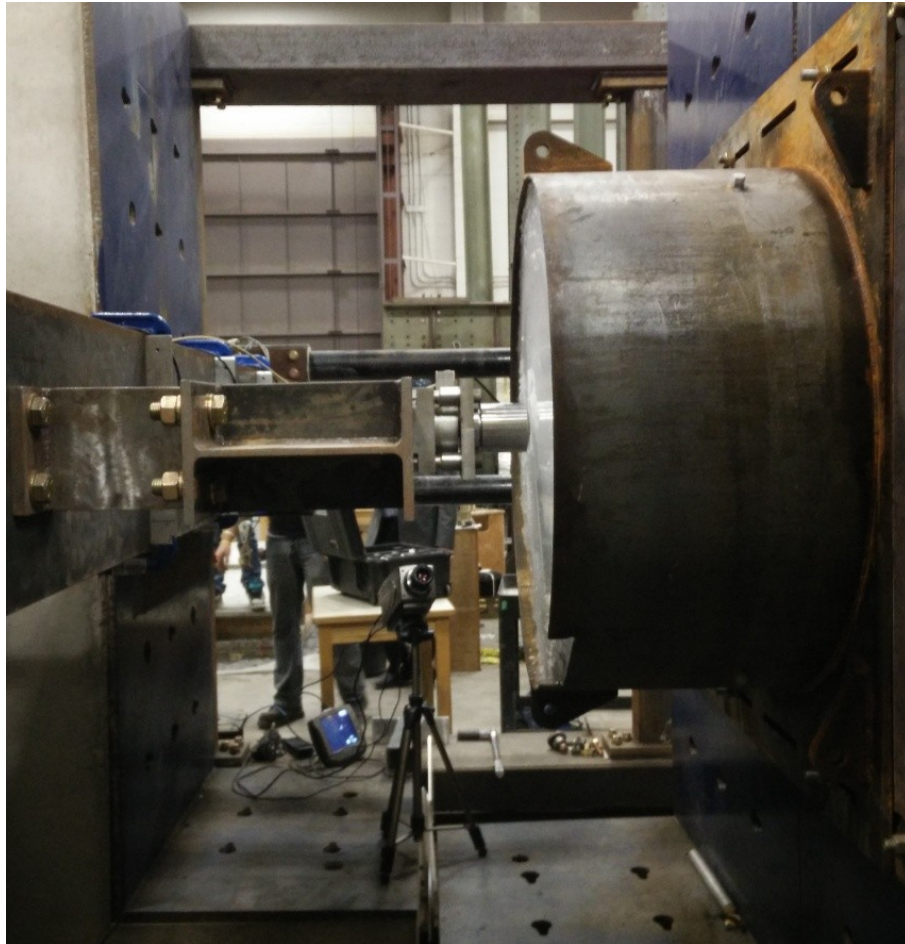
Figure 3.15: Ice sample mounted and ready to be tested.
