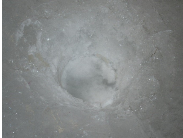
Figure 4.4: Post-test image of the indented area.
