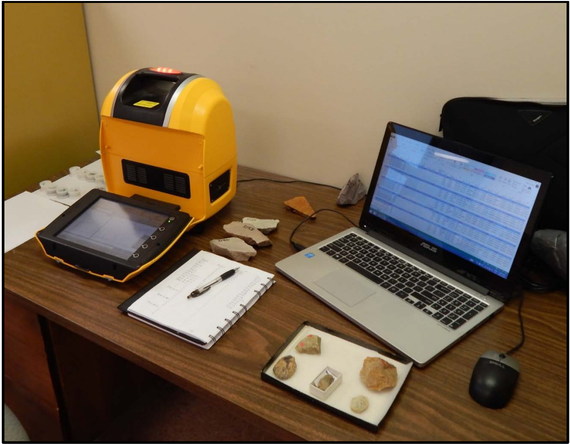
Figure 3-6: Benchtop OlympeX/Innov-X X5000 portable x-ray spectrometer.
